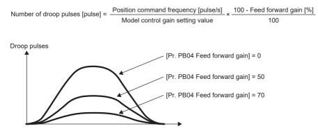
When [Pr. PB04] is set to "100", a large overshoot occurs at acceleration/deceleration although the droop pulses at a constant speed become "0".
