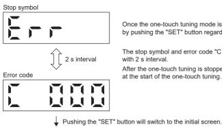
Once the one-touch tuning mode is in progress, the one-touch tuning mode can be stopped by pushing the "SET" button regardless of what is displayed on the screen.
