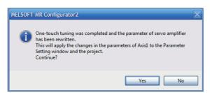
After one-touch tuning is completed, "0000" is displayed in the error code status. The settling time and overshoot amount are displayed in "Adjustment result".
