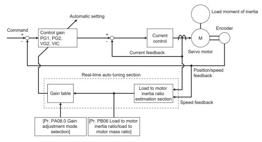
When a servo motor is accelerated/decelerated, the load to motor inertia ratio estimation section always estimates the load to motor inertia ratio from the current and speed of the servo motor. The results of estimation are written to [Pr. PB06 Load to motor inertia ratio/load to motor mass ratio]. These results can be confirmed on the status display screen on MR Configurator2.
