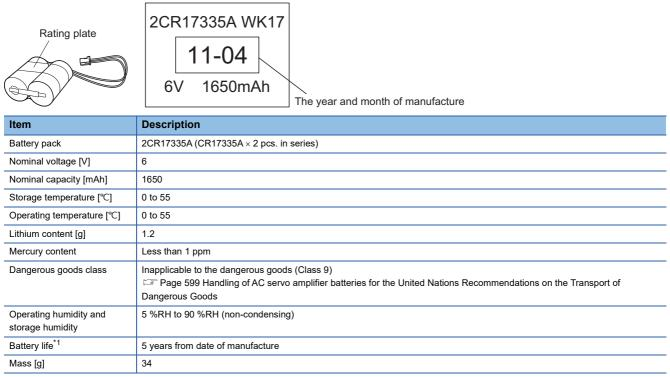
\*1 Quality of the batteries degrades by the storage condition. The battery life is 5 years from the production date regardless of the connection status.
