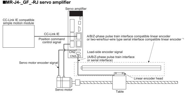
\*1 Applicable for the absolute position detection system when an absolute position linear encoder is used. In that case, a battery is not required.
