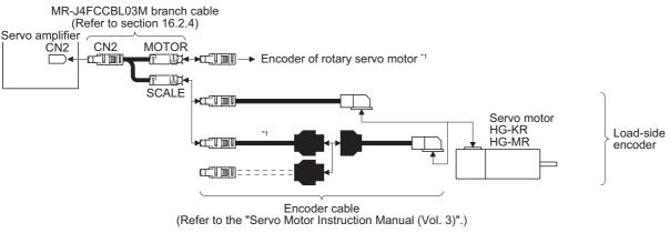
\*1 Use a two-wire type encoder cable. A four-wire type encoder cable cannot be used.
