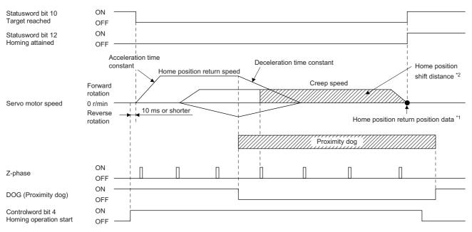
\*1 Home position return position data can be changed with [Pr. PT08] and [Pr. PT47]. Home position return position data is the current position at the time of home position return completion. (I/O mode only)
