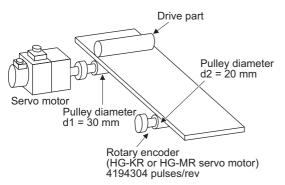
When the pulley diameters or reduction ratios differ, consider that in calculation.
