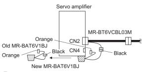
5. Mount the orange connector of the new MR-BAT6V1BJ. When the control circuit power supply is on, [AL. 9F.1] is canceled.
