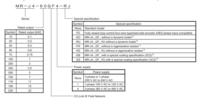
\*1 Indicates a servo amplifier of 11 kW to 22 kW that does not use a regenerative resistor as standard accessory.
