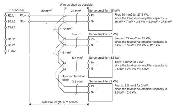
\*1 When using the servo amplifier of 7 kW or less, make sure to disconnect the wiring of built-in regenerative resistor (5 kW or less: P+ and D, 7 kW: P+ and C).
