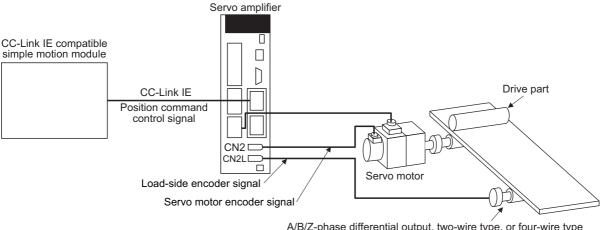
A/B/Z-phase differential output, two-wire type, or four-wire type rotary encoder HG-KR, HG-MR servo motor (4194304 pulses/rev) or synchronous encoder Q171ENC-W8 (4194304 pulses/rev)
