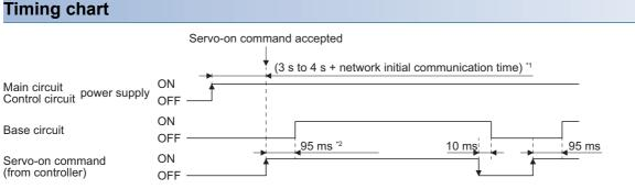
\*1 This range will be "5 s to 6 s + network initial communication time" for the linear servo system and fully closed loop system.
