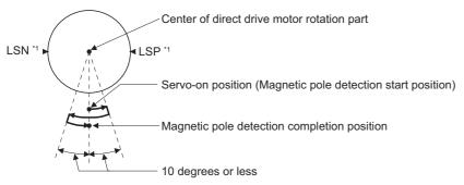
\*1 When you turn off LSP or LSN during the magnetic pole detection, the magnetic pole detection is carried on to the opposite direction. When LSP and LSN are off, [AL. 27 Initial magnetic pole detection error] occurs.
