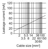
"Ig1" of 100 V class servo amplifiers is 1/2 of 200 V class servo amplifiers.
