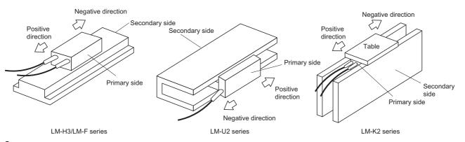
2. Confirm the increasing direction of the linear encoder.
