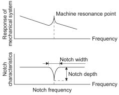
You can set five machine resonance suppression filters at most.
