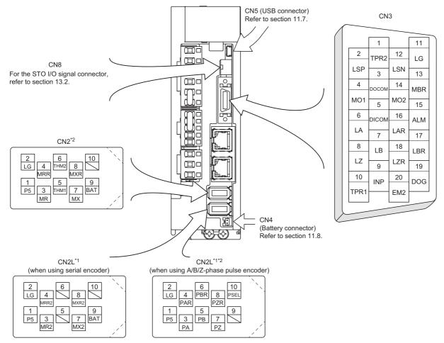
\*1 The MR-J4-\_GF\_ servo amplifier does not have CN2L connector.
