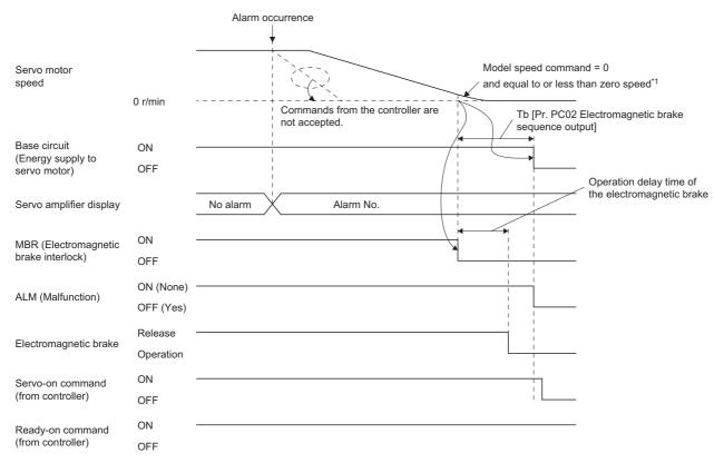
\*1 The model speed command is a speed command generated in the servo amplifier for forced stop deceleration of the servo motor.
