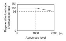
When closely mounting the servo amplifiers, operate them at the ambient temperatures of 0  $^{\circ}$ C to 45  $^{\circ}$ C or at 75% or smaller effective load ratio.
