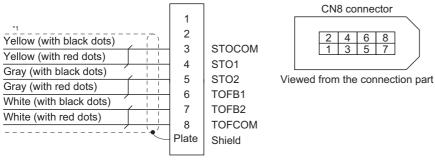
\*1 Do not use the two core wires with orange insulator (with red or black dots).
