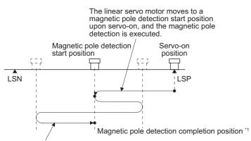
The linear servo motor reciprocates several times and returns to the magnetic pole detection start position to complete the magnetic pole detection and to go into the servo-lock status. At this time, there may be a gap, approximately a quarter of the pitch against magnetic pole, from the start position.
