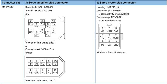
\*1 Keep open the pins shown with \_\_\_\_\_. Especially, pin 10 is provided for manufacturer adjustment. If it is connected with any other pin, the servo amplifier cannot operate normally.
