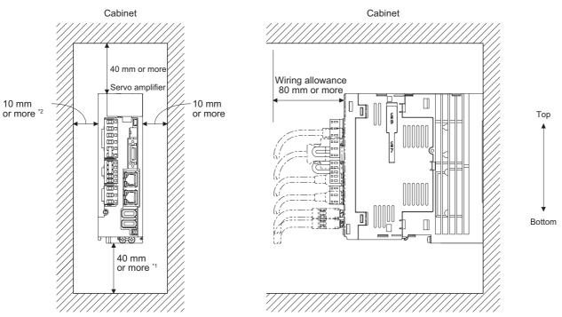
\*1 For 11 kW to 22 kW servo amplifiers, the clearance between the bottom and ground will be 120 mm or more.
