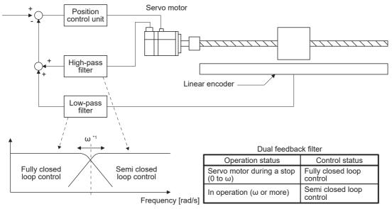
\*1 " $\omega$ " (a dual feedback filter band) is set by [Pr. PE08].
