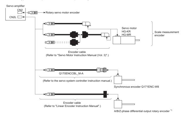
\*1 A/B/Z-phase differential output rotary encoders that can be used as a scale measurement encoder have the same specifications as the A/B/Z-phase differential output linear encoders. Refer to "Linear Encoder Instruction Manual".
