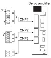
\*1 A pin for preventing improper connection is inserted to N- of CNP1 connector.
