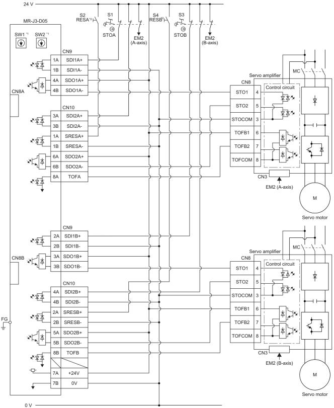
\*1 Set the delay time of STO output with SW1 and SW2. These switches are recessed to prevent accidental change of the setting.
