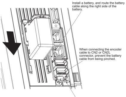
Install a battery, and connect the plug to the CN4 connector.
