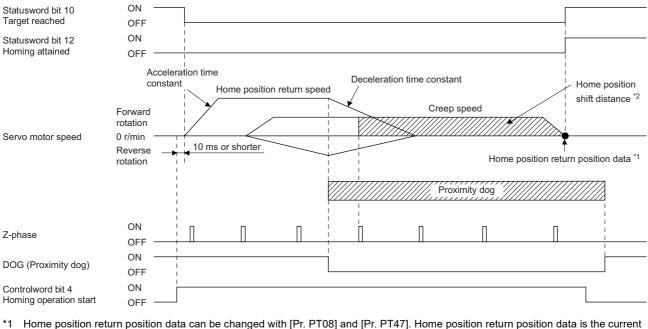
position return position data can be changed with [Pr. P108] and [Pr. P147]. Home position return position data is the cu
