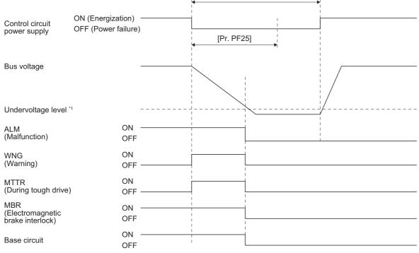
Instantaneous power failure time of the control circuit power supply
