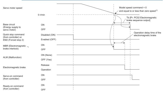
\*1 ON: Electromagnetic brake is not activated. OFF: Electromagnetic brake is activated.
