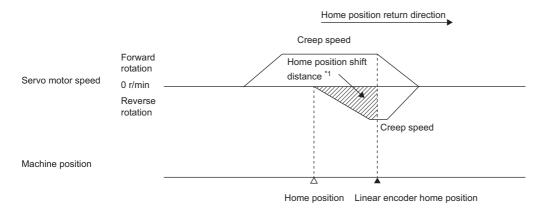
\*1 Home position shift distance can be changed with [Pr. PT07] and [Pr. PT69]. When the stroke end is detected
