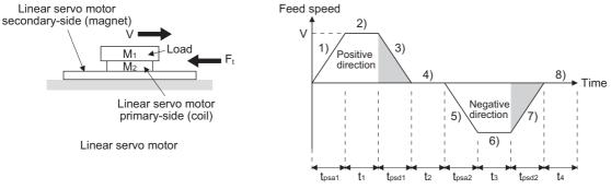
The following shows equations of the linear servo motor thrust and energy at the driving pattern above.
