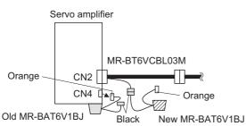
4. Remove the old MR-BAT6V1BJ from servo amplifier and mount the new MR-BAT6V1BJ. When the control circuit power supply is on, [AL. 9F.1] occurs after 3).
