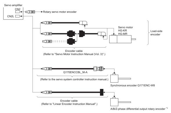
\*1 A/B/Z-phase differential output rotary encoders that can be used as a load-side encoder have the same specifications as the A/B/Zphase differential output linear encoders. Refer to "Linear Encoder Instruction Manual".
