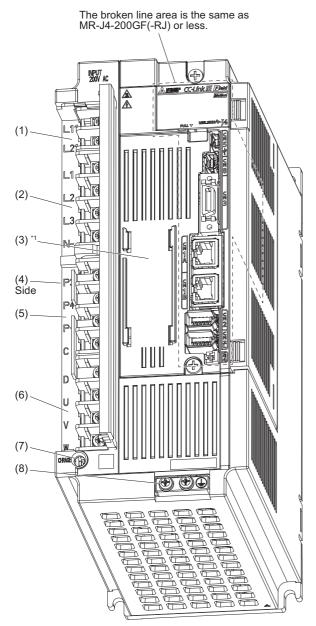
$<sup>^{\</sup>star 1}$   $\,$  Lines for slots around the battery holder are omitted from the illustration.
