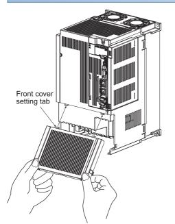
1) Insert the front cover setting tabs into the sockets of servo amplifier (2 places).
