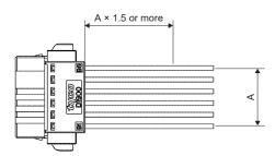
• Be sure that wires are not pulled excessively when the connector is inserted.
