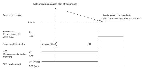
\*1 The model speed command is a speed command generated in the servo amplifier for forced stop deceleration of the servo motor.
