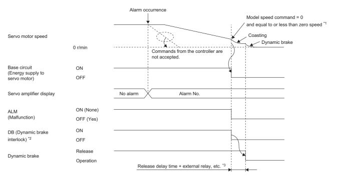
\*1 The model speed command is a speed command generated in the servo amplifier for forced stop deceleration of the servo motor.
