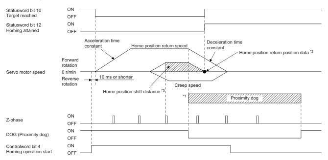
\*1 After the front end of the proximity dog is detected, if the rear end of the proximity dog is detected without stop, [AL. 90] occurs. Check the length of the proximity dog or check the home position return speed and creep speed.
