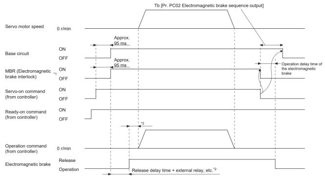
\*1 ON: Electromagnetic brake is not activated.
