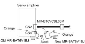
3. Remove the orange connector of the old MR-BAT6V1BJ. When the control circuit power supply is on, performing 3) without [AL. 9F.1 Low battery] triggers [AL. 9F.1].
