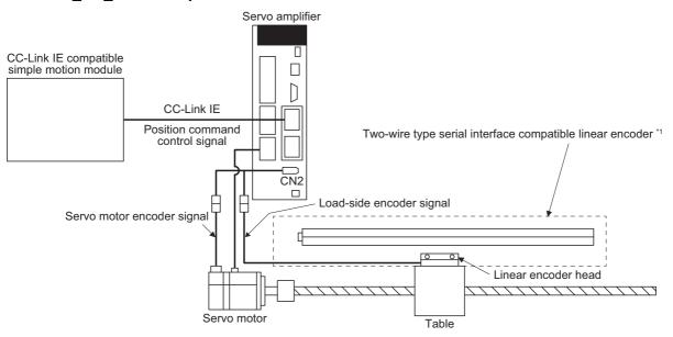
\*1 Applicable for the absolute position detection system when an absolute position linear encoder is used. In that case, a battery is not required.
