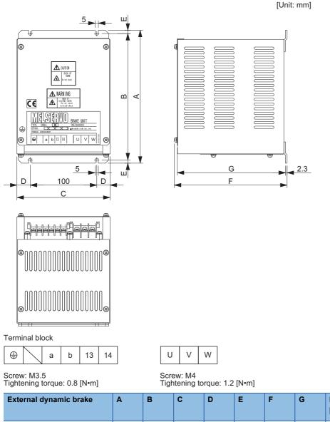
Connection wire [mm<sup>2</sup>]<sup>\*1</sup> Mass [kg] U/V/W Except U/V/W DBU-11K 200 190 140 20 5 170 163.5 2 5.5 (AWG 10) 2 (AWG 14) DBU-15K/DBU-22K-R1 250 238 150 25 6 235 228 6 5.5 (AWG 10) 2 (AWG 14)
