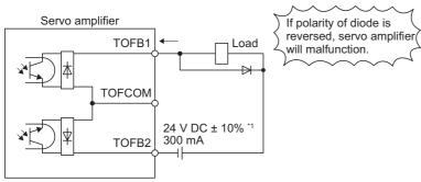
\*1 If the voltage drop (maximum of 5.2 V) interferes with the relay operation, apply high voltage (maximum of 26.4 V) from external source.
