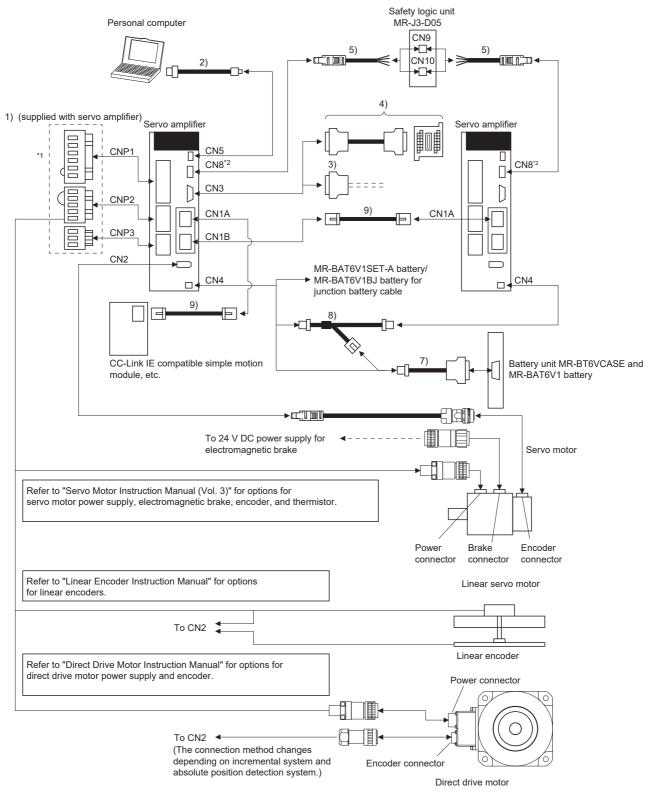
\*1 Connectors for 3.5 kW or less. For 5 kW or more, it is a terminal block.
