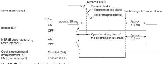
\*1 ON: Electromagnetic brake is not activated. OFF: Electromagnetic brake is activated.
