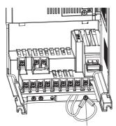
Built-in regenerative resistor lead terminal fixing screw
