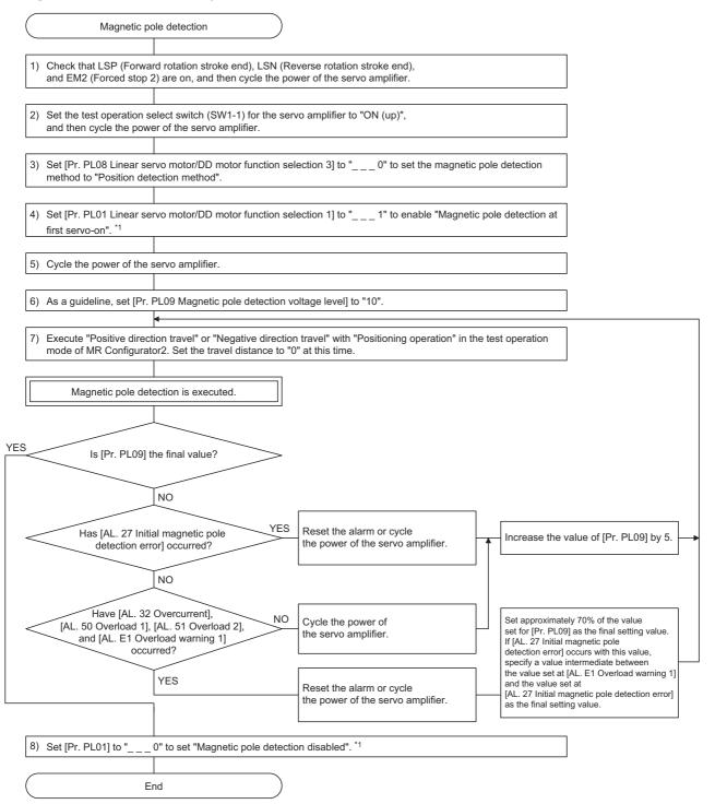
\*1 For the incremental system, the [Pr. PL01] setting is not required.
