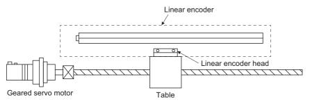
Calculate the number of linear encoder pulses per ball screw revolution.
