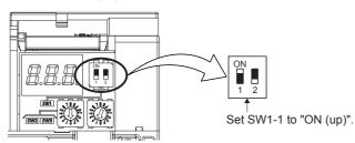
Turning "ON (up)" SW1-1 during power-on will not enable the test operation mode.
