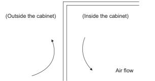
When air flows along the outer wall of the cabinet, effective heat exchange will be possible, because the temperature slope inside and outside the cabinet will be steeper.
