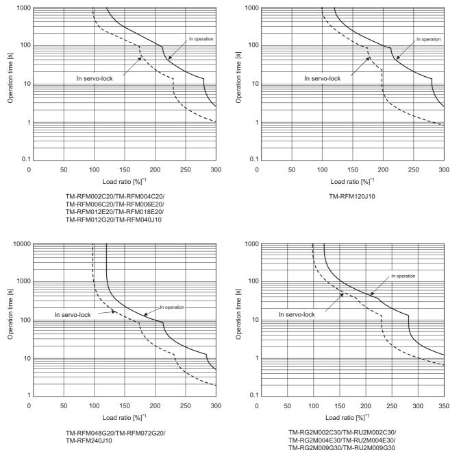
\*1 If operation that generates torque more than 100% of the rating is performed with an abnormally high frequency in a direct drive motor stop status (servo-lock status) or in a 50 r/min or less low-speed operation status, the servo amplifier may malfunction regardless of the electronic thermal relay protection.
