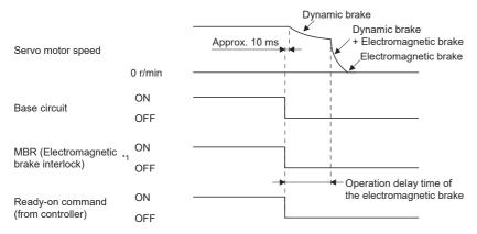
\*1 ON: Electromagnetic brake is not activated. OFF: Electromagnetic brake is activated.
