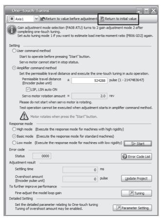
Clearing one-touch tuning is completed, the following window will be displayed. (returning to initial value)
