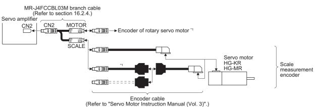
\*1 Use a two-wire type encoder cable. A four-wire type encoder cable cannot be used.
