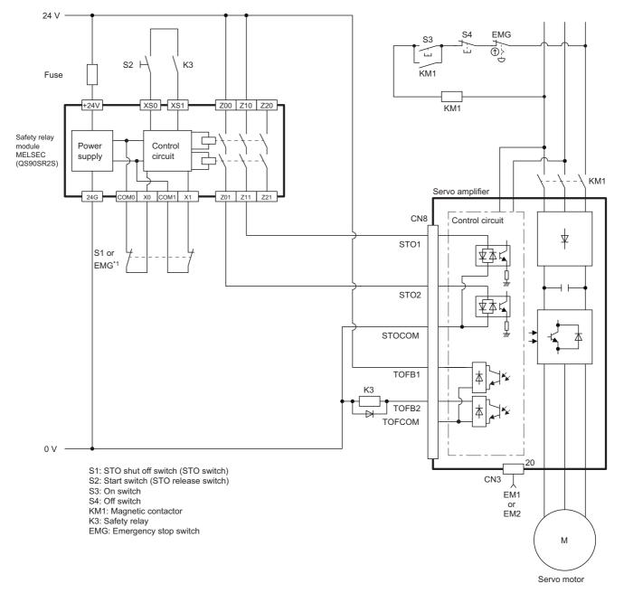
\*1 To enable the STO function of the servo amplifier by using "Emergency switching off", change S1 to EMG. The stop category at this time is "0". If STO is turned off while the servo motor is rotating, [AL. 63 STO timing error] will occur.
