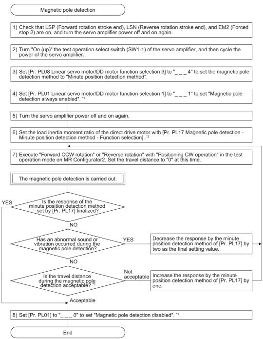
\*1 For the incremental system, the [Pr. PL01] setting is not required.
