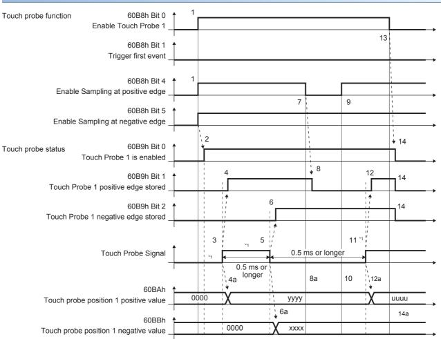
\*1 Turn on and off Touch Probe Signal so that both the on time and off time are 0.5 ms or longer.
