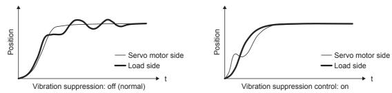
When the advanced vibration suppression control II ([Pr. PB02 Vibration suppression control tuning mode]) is executed, the vibration frequency at load side is automatically estimated to suppress load-side vibration two times at most.
