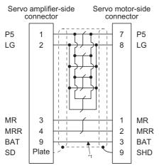
\*1 Always make connection for use in an absolute position detection system. Wiring is not necessary for use in an incremental system.
