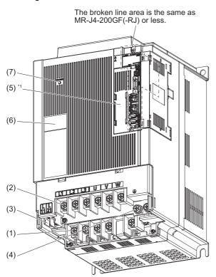
\*1 Lines for slots around the battery holder are omitted from the illustration.
