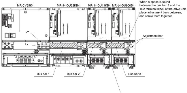
Screw the bus bars 2 and 3 together by placing one over the other.
