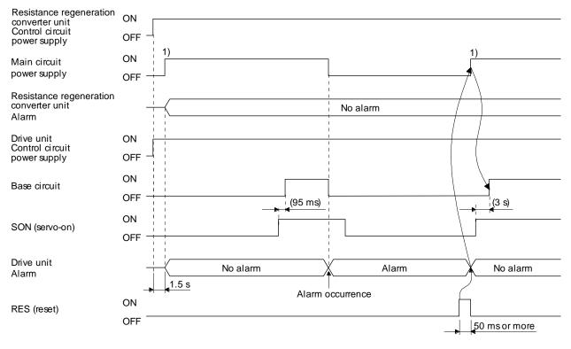
1) in figure After the start-up of the drive unit is completed, the main circuit power is supplied while the drive unit and the resistance regeneration converter unit have no alarm.
