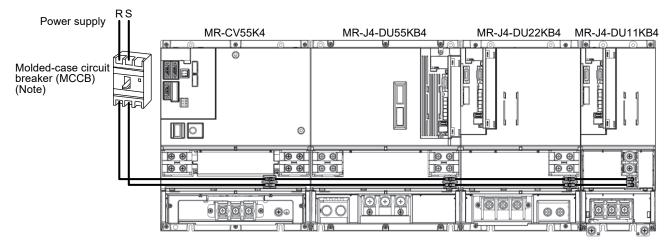
Note. Install a molded-case circuit breaker dedicated to the control circuit power supply. Do not use a molded-case circuit breaker for the main circuit power supply.
