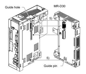
5) Insert the guide pins of the MR-D30 in the guide holes located on the side of the control interface.
