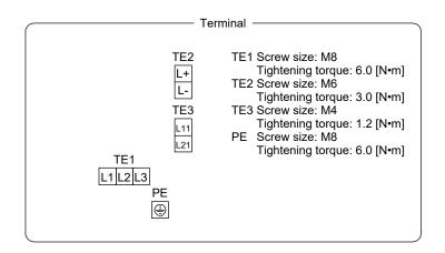
Mass: 12.1 [kg] Mounting screw Screw size: M5 Tightening torque: 3.24 [N•m]
