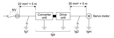
Use an earth-leakage current breaker designed for suppressing harmonics/surges. Calculate the terms of equation in section 8.9.1 from the figure.
