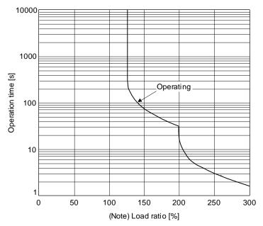
Note. Load ratio 100% indicates the rated output of the resistance regeneration converter unit. Refer to section 1.4.2 for rated output.
