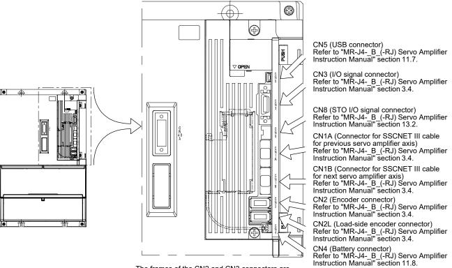
The frames of the CN2 and CN3 connectors are connected to the protective earth terminal in the drive unit.
