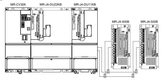
1.3.2 Combinations of the resistance regeneration converter unit and drive unit
