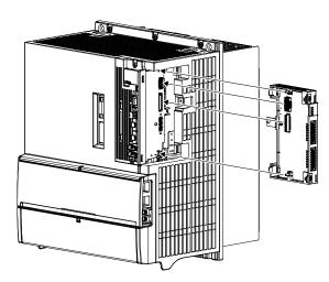
3) Insert the guide pins of the MR-D30 in the guide holes located on the side of the drive unit.
