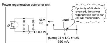
Note. If the voltage drop (maximum of 2.6 V) interferes with the relay operation, apply a high voltage (maximum of 26.4 V) from an external source.
