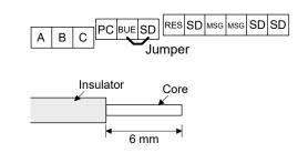
Wire the stripped cable after twisting to prevent the cable from becoming loose. In addition, do not solder it. Screw size: M3
