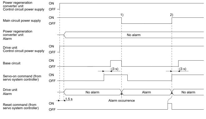
1) in figure When an alarm occurs in the drive unit, shut off the main circuit power supply with the external sequence.
