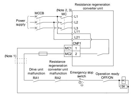
Internal connection diagram of CNP1
