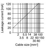
(2) Converter unit/drive unit's leakage current example (Iga)
