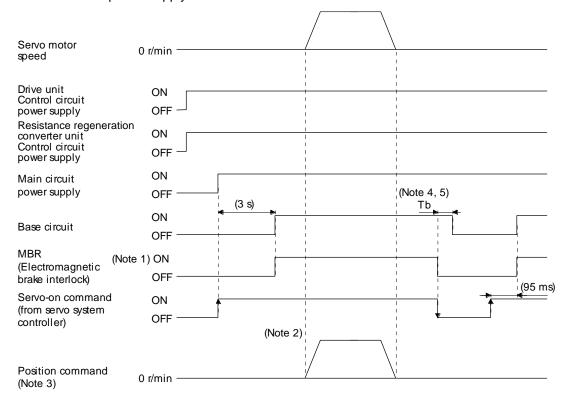
Note 1. When setting up an electromagnetic brake at customer's side, make up a sequence which will operate the electromagnetic brake as follow using MBR.
