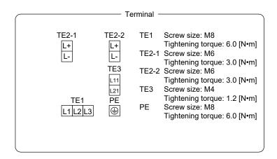
Mass: 25.0 [kg] Mounting screw Screw size: M5 Tightening torque: 3.24 [N•m]
