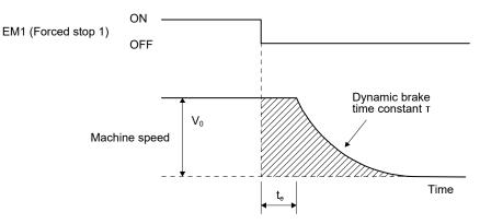
Use the following equation to calculate an approximate coasting distance to a stop.
