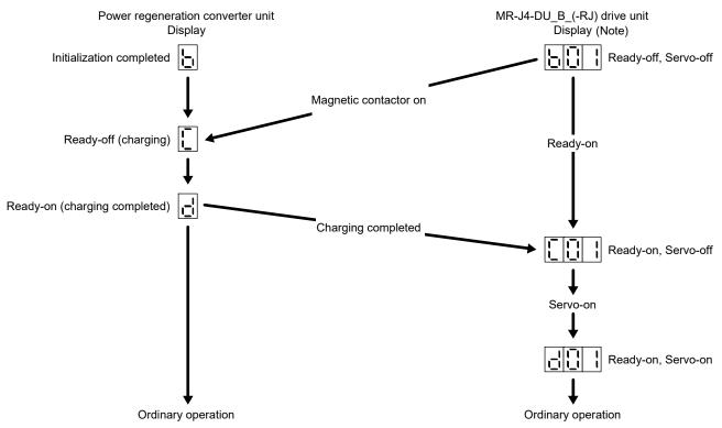
Note. For the detailed display transition of the drive unit, refer to "MR-J4-\_B\_(-RJ) Servo Amplifier Instruction Manual".
