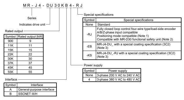
Note 1. The positioning mode is available only with MR-J4-DU\_A\_-RJ.
