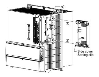
3) Insert the side cover setting clips into the recesses e) of the drive unit.
