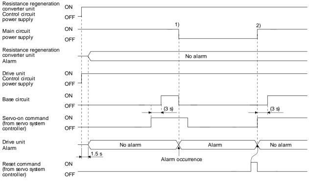
1) in figure When an alarm occurs in the drive unit, shut off the main circuit power supply using the external sequence.
