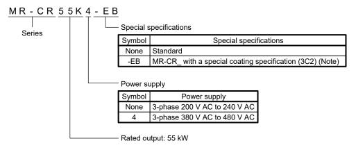
Note. Type with a specially-coated resistance regeneration converter unit board (IEC 60721-3-3:1994 Class 3C2). Refer to section 10.3 for details.
