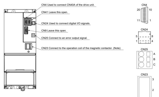
Note. The connector for CN23 and an open tool are supplied with the power regeneration converter unit.
