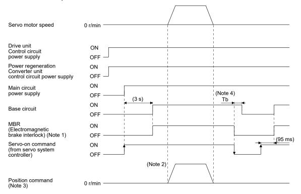
Note 1. When an electromagnetic brake is installed externally, configure a sequence which operates the electromagnetic brake with MBR as follows.
