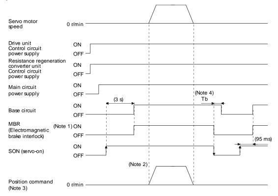
Note 1. When setting up an electromagnetic brake at customer's side, make up a sequence which will operate the electromagnetic brake as follow using MBR. ON: Electromagnetic brake is not activated.
