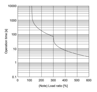
Note. Load ratio 100% indicates the continuous rating of the converter unit.
