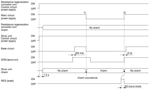
1) in figure When an alarm occurs in the drive unit, shut off the main circuit power supply using the external sequence.
