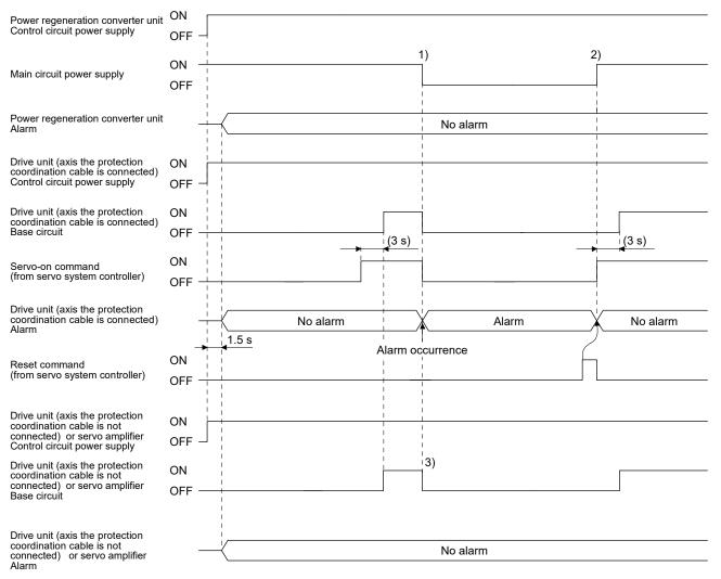
1) in figure When an alarm occurs in the drive unit, shut off the main circuit power supply with the external sequence.
