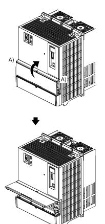
1) Pull up the cover using point A) as a support.
