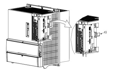
2) When mounting the MR-D30 for the first time, cut off the part a) from the case after removing the side cover. When cutting off the part c), be careful not to damage the case of the drive unit. After the part a) is cut off, inside of the drive unit will be exposed even after the side cover or the MR-D30 is attached. Prevent foreign materials from entering through the opened area into the drive unit.
