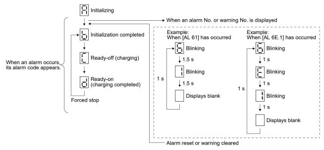
(4) Display transition of the power regeneration converter unit/MR-J4-DU\_B\_(-RJ) drive unit The following shows the display transition of the power regeneration converter unit in which a protection coordination is enabled and MR-J4-DU\_B\_(-RJ) drive unit.
