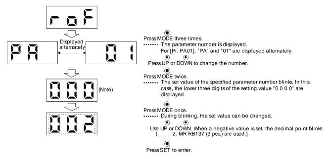
Note. When the lower three digits of the four digits are displayed, pressing the "MODE" button displays the fourth digit. However, do not change the setting of the fourth digit. Pressing the "MODE" button again resets the display to the lower three digits.
