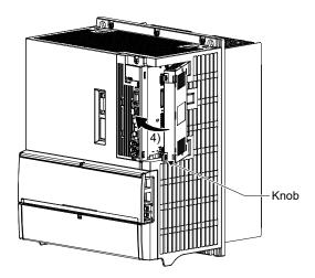
4) Push against the drive unit at the supporting point e) shown in procedure 1) until the clips clip into place.
