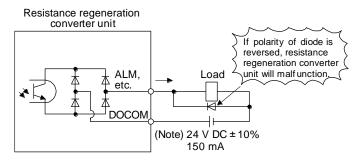
Note. If the voltage drop (maximum of 2.6 V) interferes with the relay operation, apply high voltage (maximum of 26.4 V) from external source.
