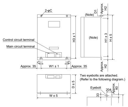
Note. Ventilation ports are provided on both sides and the top. The bottom is open.
