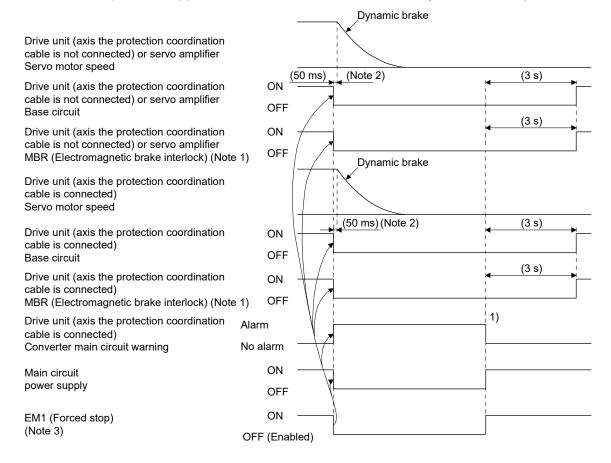
Note 1. When an electromagnetic brake is installed externally, configure a sequence which operates the electromagnetic brake with MBR as follows. ON: Electromagnetic brake is not activated. OFF: Electromagnetic brake is activated.
