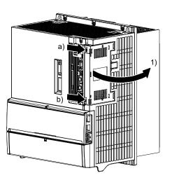
1) While pushing the clips (a), b)), and pull out the side cover in the arrow direction.
