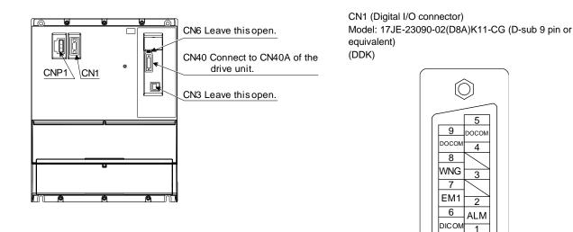
CNP1 (Magnetic contactor wiring connector) Model: GFKC 2,5/2-STF-7,62 (Phoenix Contact)
