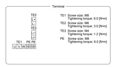
Mass: 15.2 [kg] Mounting screw Screw size: M5 Tightening torque: 3.24 [N•m] (3) MR-J4-DU30KB(-RJ)/MR-J4-DU37KB(-RJ)/MR-J4-DU45KB4(-RJ)/MR-J4-DU55KB4(-RJ)
