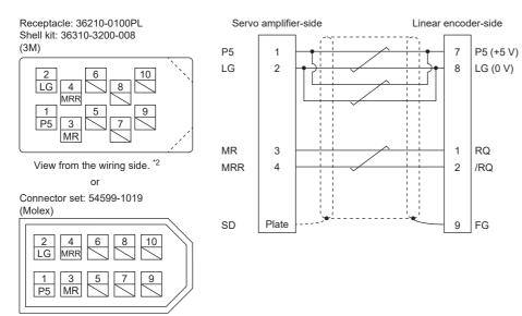
Housing: 1-172161-9 Connector pin: 170359-1 (TE Connectivity or equivalent) Cable clamp: MTI-0002 (Toa Electric Industrial)
