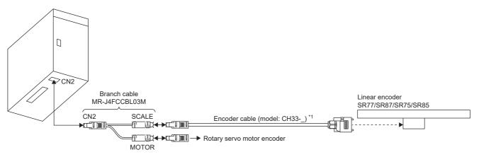
\*1 This optional cable is manufactured by Magnescale and should be prepared by the customer.
