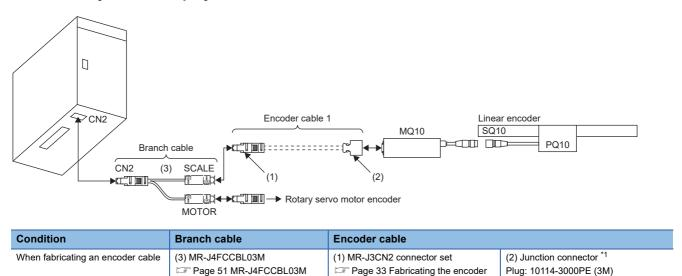
cable used to connect the servo
