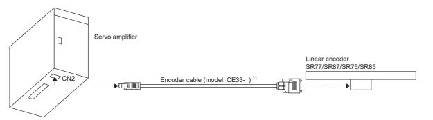
\*1 This optional cable is manufactured by Magnescale and should be prepared by the customer.
