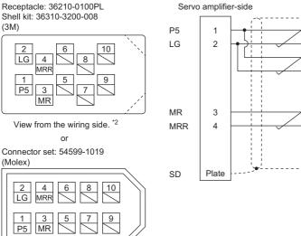
Linear encoder-side Linear encoder-side 1 2 3 4 Plate Linear encoder-side 7 8 P5 LG 1 RQ 9 FG Housing: 1-172161-9 Connector pin: 170359-1 (TE Connectivity or equivalent) Cable clamp: MTI-0002 (Toa Electric Industrial)
