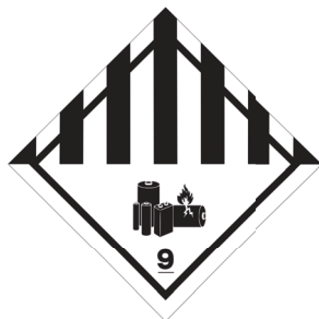
Figure 2: Lithium battery hazard label example
