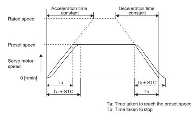
This function is enabled in the profile position mode, profile velocity mode, and positioning mode (point table method). This function is disabled during homing.
