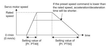
For example, for a servo motor with a rated speed of 3000 [r/min], set 3000 [ms] to accelerate from 0 [r/min] to 1000 [r/min] in 1000 [ms].
