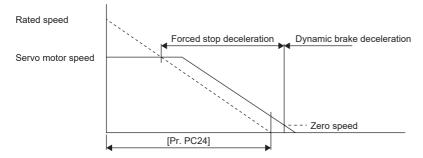
This servo parameter corresponds to [Quick stop deceleration (Obj. 6085h)]. When the object is mapped to the cyclic communication, do not write values with engineering tools because the controller overwrites the servo parameter values written with engineering tools.
