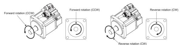
The positive and negative directions of the linear servo motor are as follows.
