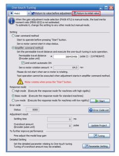
Once initialization of one-touch tuning is complete, the following window will be displayed. (When returning servo parameters to the initial value.)
