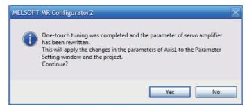
After one-touch tuning is completed, "0000" is displayed in the error code status. The settling time and overshoot amount are displayed in "Adjustment result".
