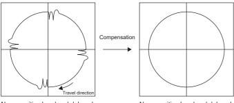
Non-sensitive band and delayed timing before compensation
