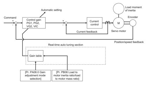
In auto tuning mode 2, the optimum control gain is automatically set based on the internal gain table, the value set for the load inertia moment ratio ([Pr. PB06]), and the responsiveness ([Pr. PA09]).
