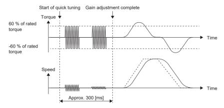
The following servo parameters are adjusted automatically in quick tuning.
