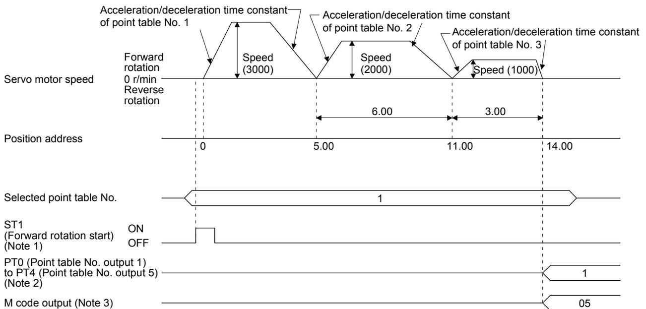
Note 1. Switching on ST2 (Reverse rotation start) starts positioning in the reverse rotation direction.
