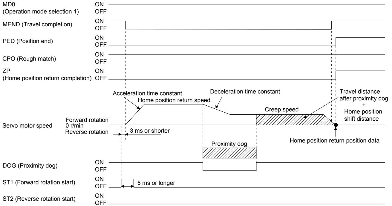
The setting value of [Pr. PT08 Home position return position data] is used as the position address at the home position return completion.
