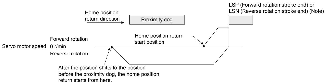
Note. The software limit cannot be used instead of LSP (Forward stroke end) and LSN (Reverse stroke end).
