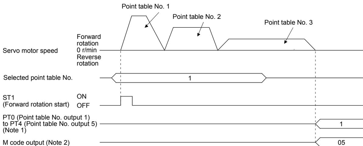
Note 1. For MR-JE-\_A servo amplifiers, up to four points of DO are available; therefore, PT0 to PT4 cannot be outputted simultaneously.
