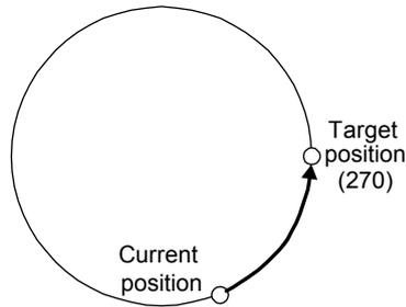
When the position data of -90.000 degrees is specified, the servo motor rotates in the CCW direction.
