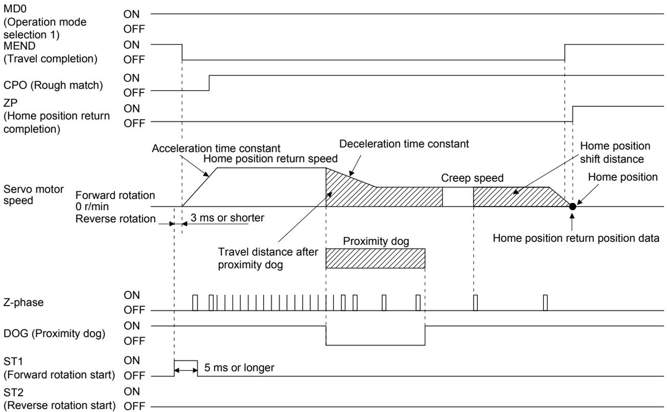
The setting value of [Pr. PT08 Home position return position data] is used as the position address at the home position return completion.
