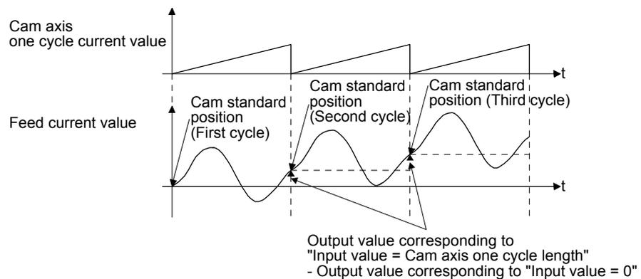
For to-and-fro control, use the output value corresponding to "Input value = Cam axis one cycle length" that is equal to output value corresponding to "Input value = 0".
