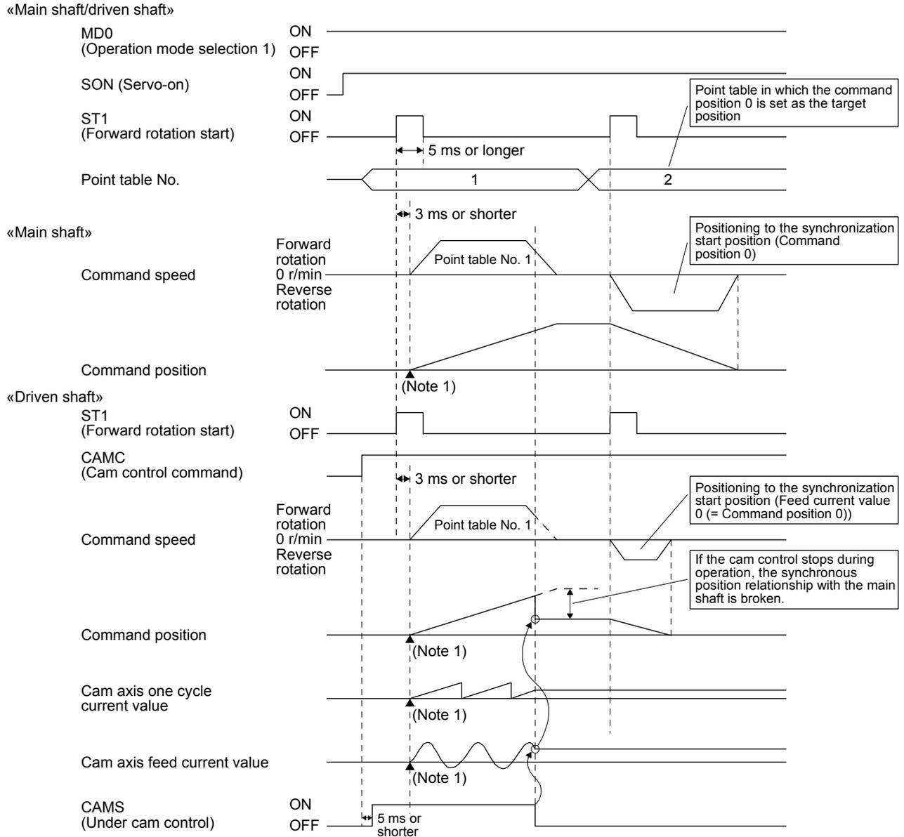
The above shows an example for when the synchronization starting point is the point where both command position and feed current value are "0".
