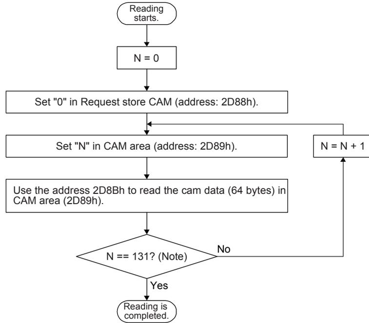
Note. The size of cam data is fixed to 8388 bytes. Thus, N, the setting range of the cam storage area is 0 to 131. Only a part of cam data cannot be read. Read the cam data stored in all areas.
