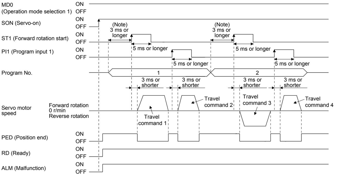
Note. The detection of external input signals is delayed by the time set in the input filter setting of [Pr. PD29]. Considering the output signal sequence from the controller and signal variations due to hardware, configure a sequence that changes the program selection earlier.
