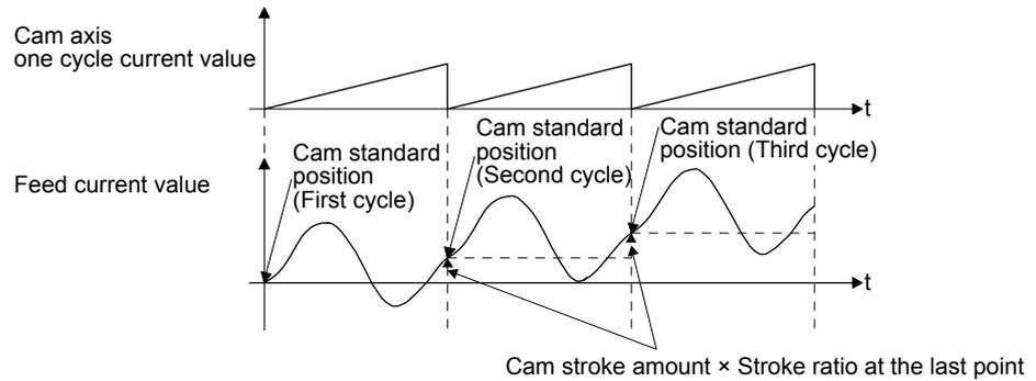
For to-and-fro control, create the cam data in which the stroke ratio at the last point is 0%.
