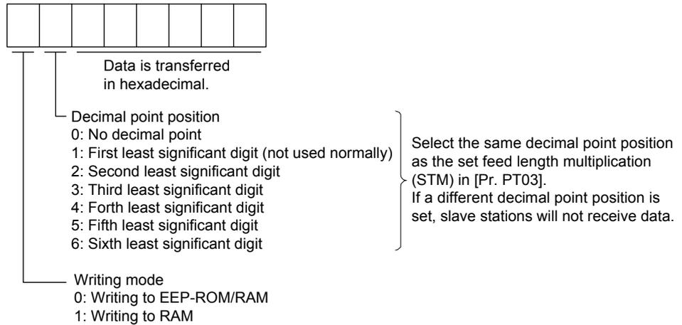
When changing the position data frequently using communication, set "1" to the write mode to change only the RAM data in the servo amplifier.
