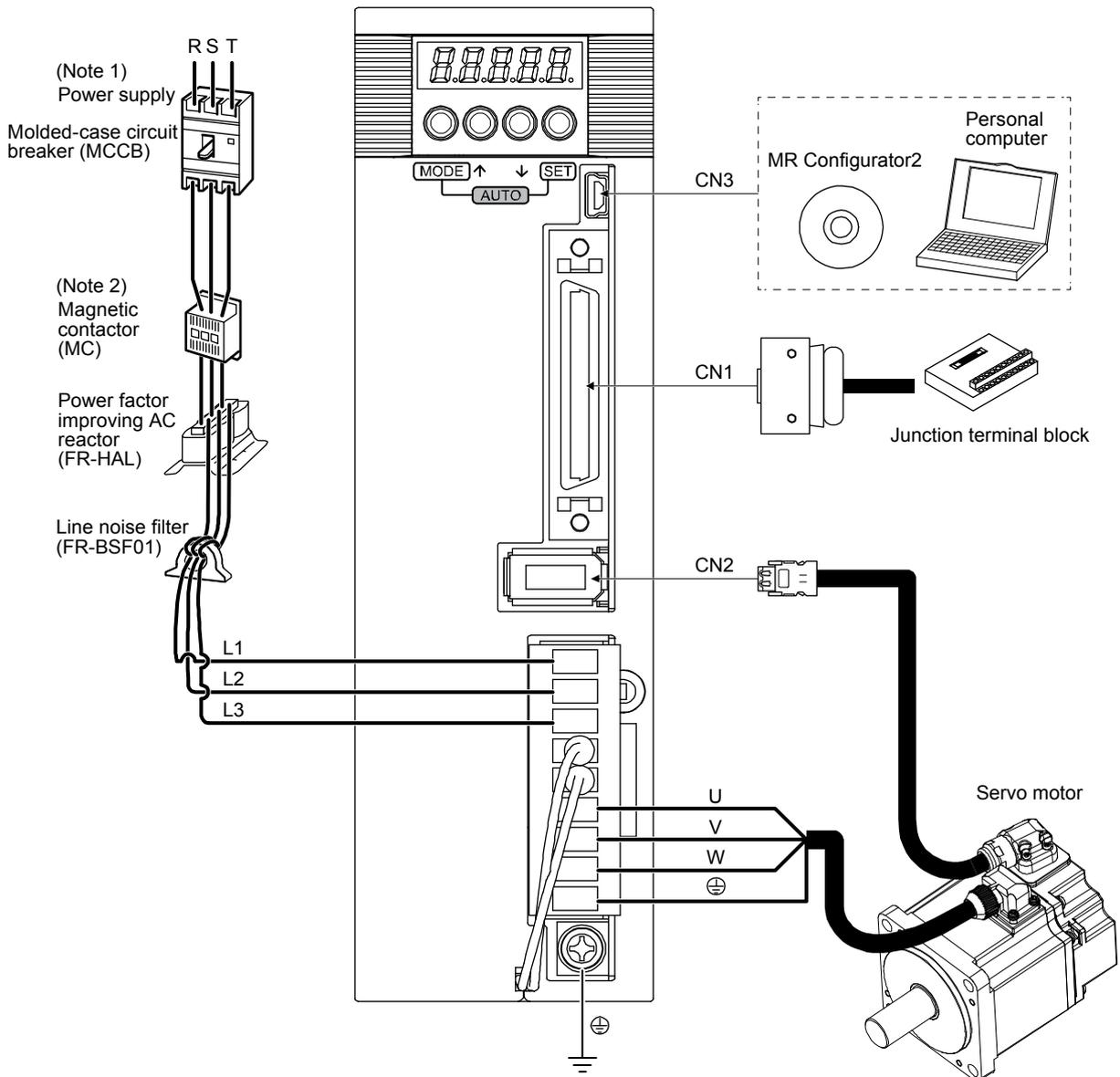
Note 1. For 1-phase 200 V AC to 240 V AC, connect the power supply to L1 and L3. Leave L2 open. For power supply specifications, refer to section 1.3 of "MR-JE-\_A Servo Amplifier Instruction Manual".
