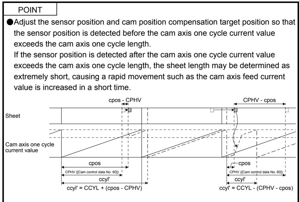
The cam position compensation processing compensates the difference between the target position for detecting the sensor and the actual position for detecting the sensor by shifting the cam axis one cycle current value.  $ccyl'$ , the cam axis one cycle length (sheet length) after compensation, is calculated as follows:
