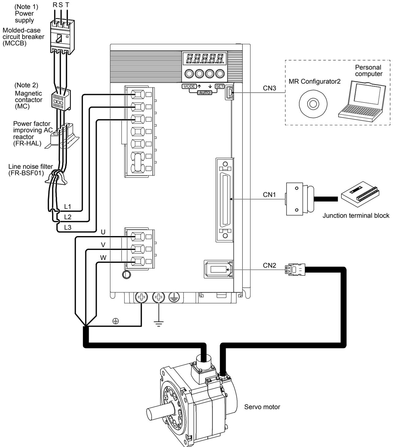
Note 1. A 1-phase 200 V AC to 240 V AC power supply may be used with the servo amplifier of MR-JE-200A. For 1-phase 200 V AC to 240 V AC, connect the power supply to L1 and L2. Leave L3 open. For power supply specifications, refer to section 1.3 of "MR-JE-\_A Servo Amplifier Instruction Manual".
