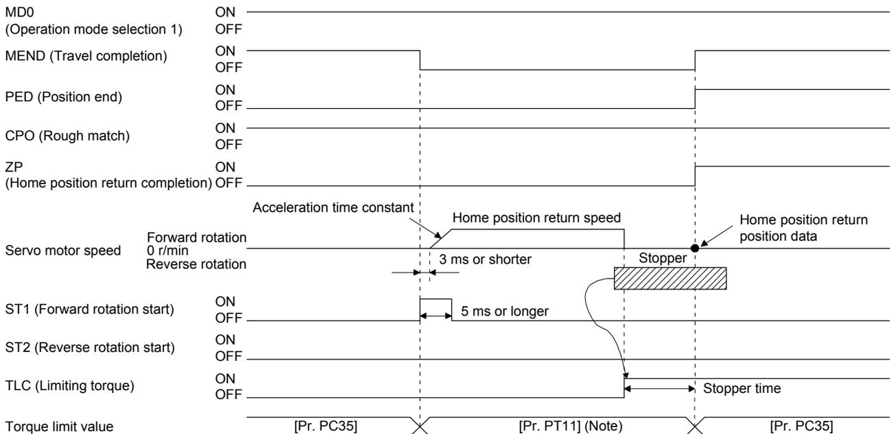
Note. The following torque limits are enabled.
