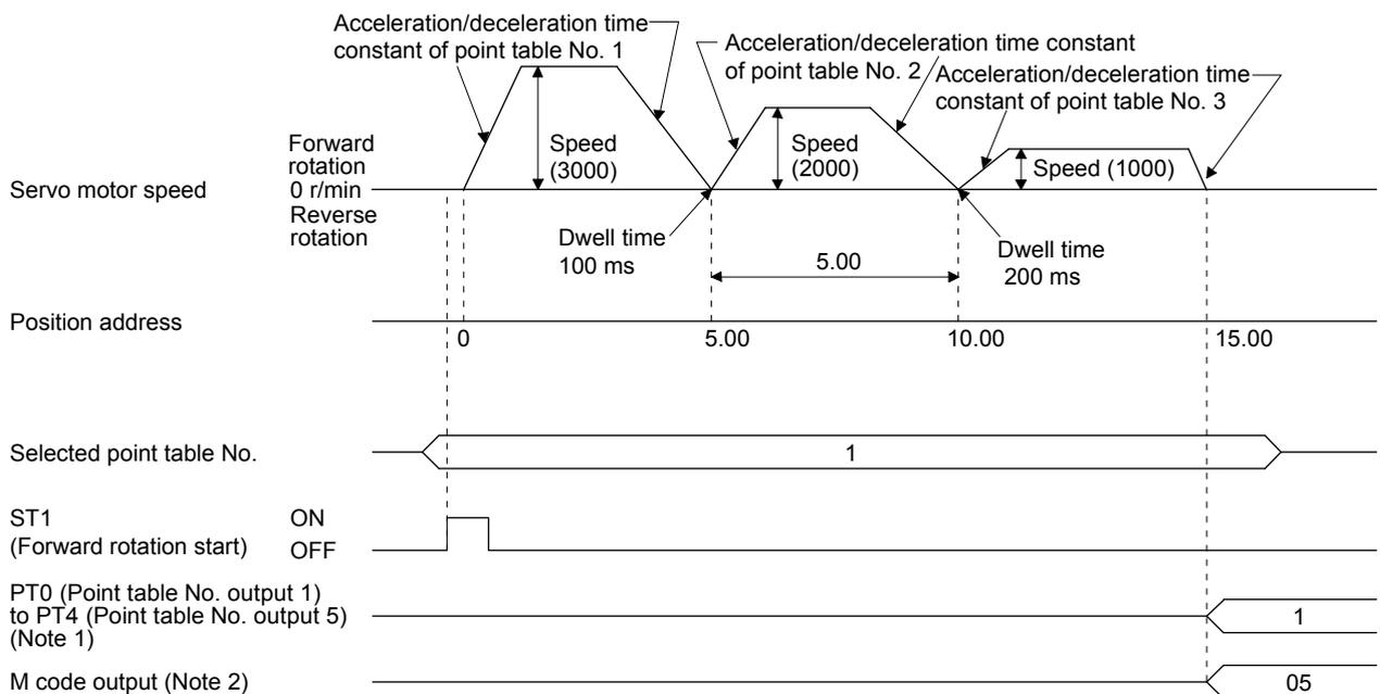
Note 1. For MR-JE-\_A servo amplifiers, up to four points of DO are available; therefore, PT0 to PT4 cannot be outputted simultaneously.
