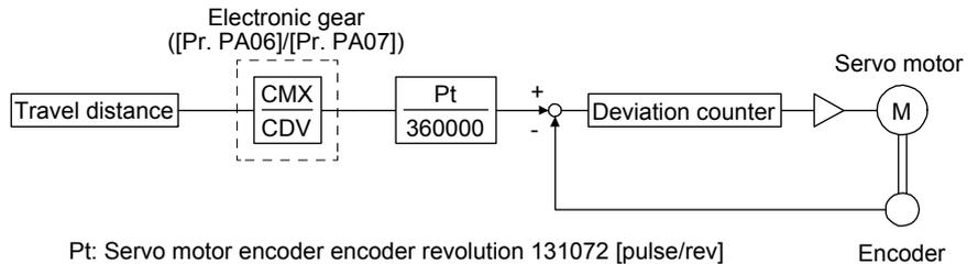
Pt: Servo motor encoder encoder revolution 131072 [pulse/rev]
