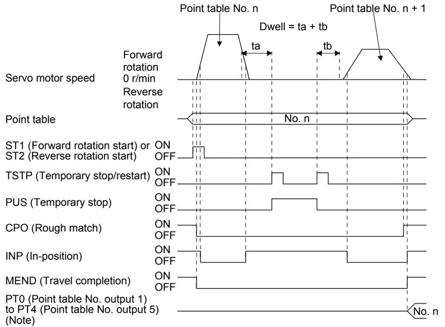
Note. For MR-JE-\_A servo amplifiers, up to four points of DO are available; therefore, PT0 to PT4 cannot be outputted simultaneously.
