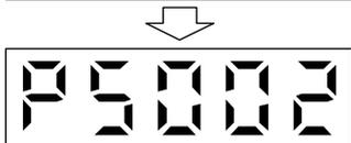
When the upper two digits or the lower two digits blink, the display returns to the teaching setting initial screen by pressing the "MODE" button.
