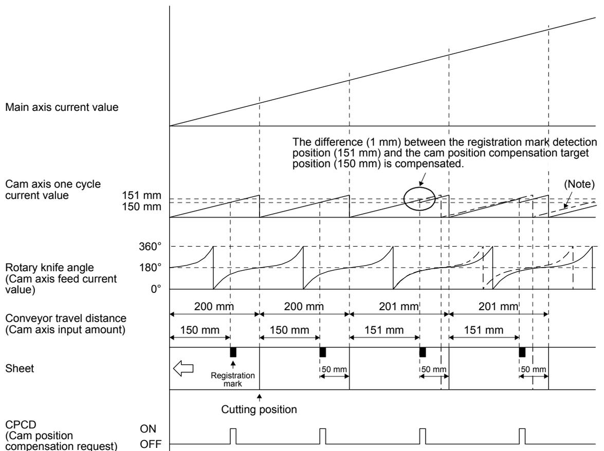
Note. The dot-and-dash line in the above figure shows a waveform of when compensation is not executed.
