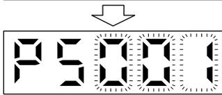
When the lower three digits blink, press the "UP" or "DOWN" button to select the point table.
