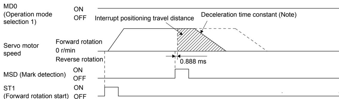
Note. Deceleration time constant of the point table at the time of start is applied for the point table method, and deceleration time constant set by the program in execution is applied for the program method.
