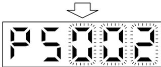
When the lower three digits blink, press the "SET" button to complete the teaching setting preparation. The upper two digits on the display will blink on completion of proper preparation
