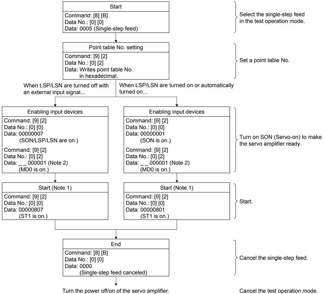
Note 1. Start it after checking ZP (Home position return completion). See the 4 bit of the read data with the command [1] [2] and data No. [8] [2].
