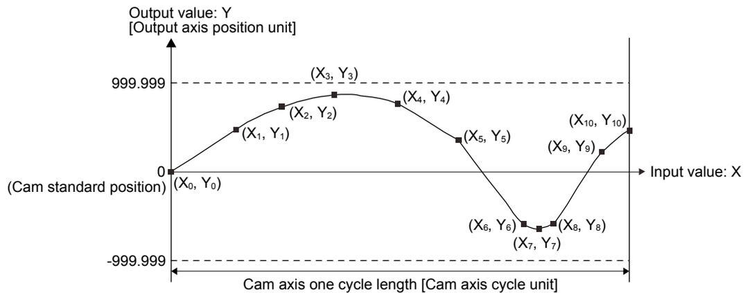
If "input value = 0" and "input value = cam axis one cycle length" are not set in the coordinate data, a control is executed by the line created from the closest two points.
