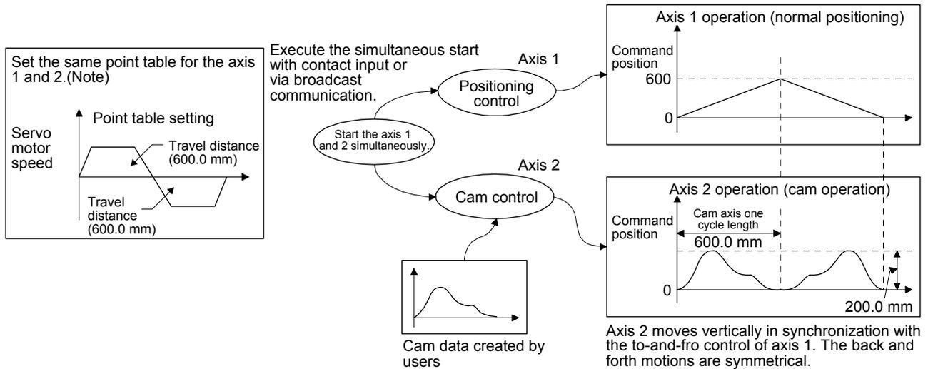
Note. Input the same positioning commands (point table data) to the driven shaft (axis 2) as those for the main shaft (axis 1).
