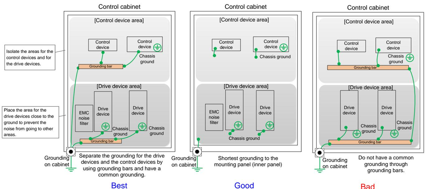
Fig. 11. Example of installing drive devices and control devices in the same control cabinet
