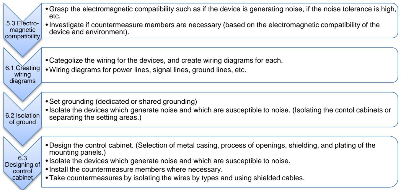
Fig. 6. Flow of designing control cabinet
