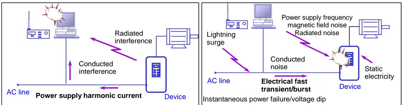
Fig. 1. EMC conceptual diagram
