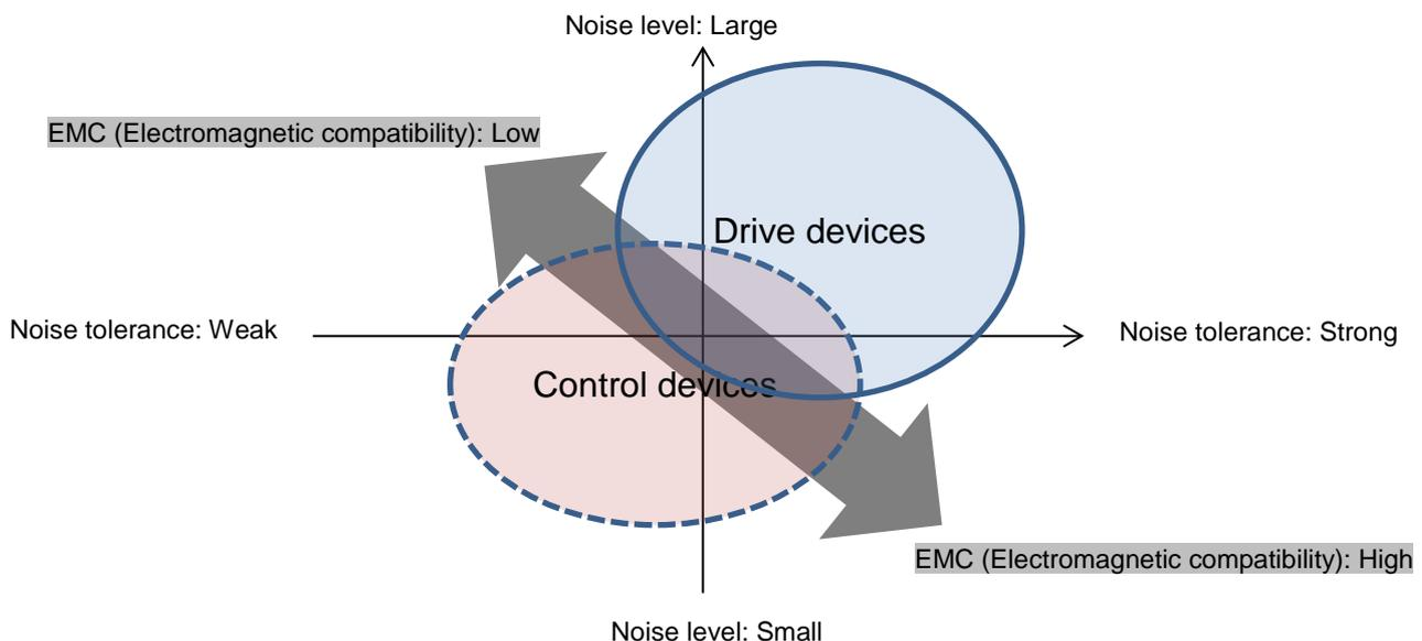
Fig. 7. Electromagnetic compatibility
