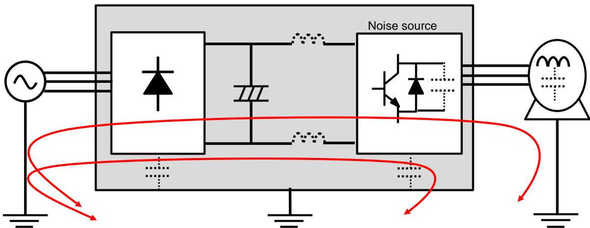
Fig. 4. Noise transmission path in a drive system having an inverter circuit
