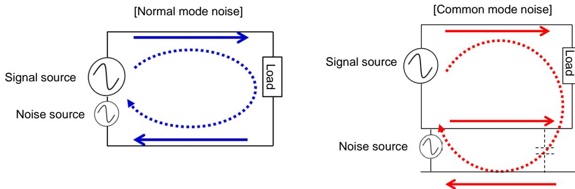
Fig. 2. Normal mode noise and common mode noise
