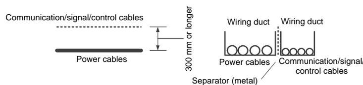
Fig. 9 Example of cabling
