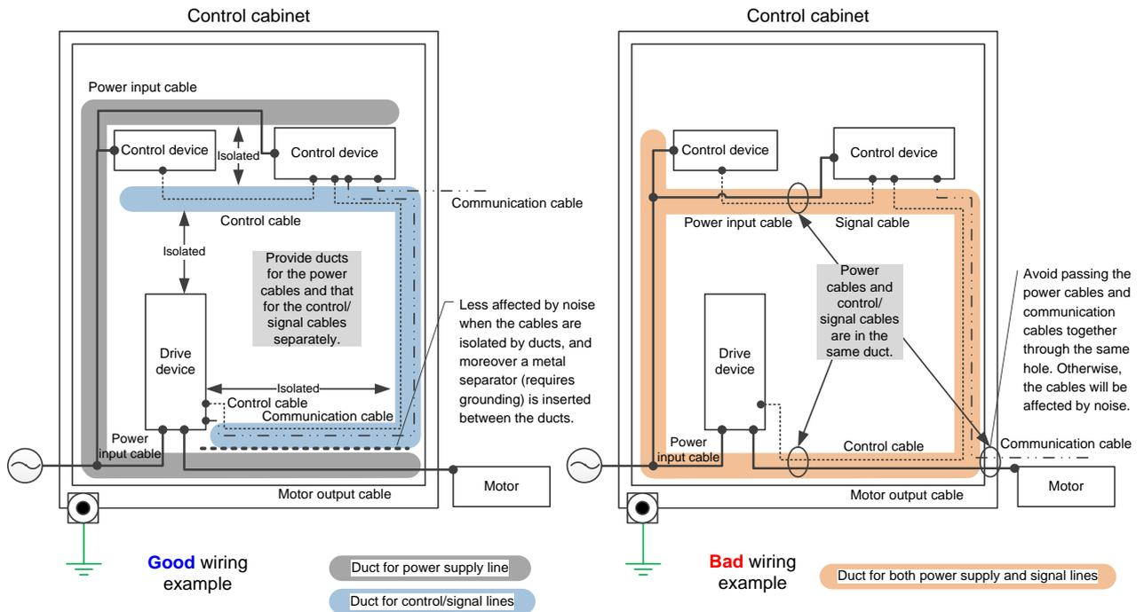
It is recommended that you keep a distance of 300 mm or longer between the power cables and the communication/signal/control cables. For some reason, if the cables are laid along close to each other, isolate the ducts and insert a metal separator to suppress the noise influence. Be sure to ground the separator to the cabinet.
