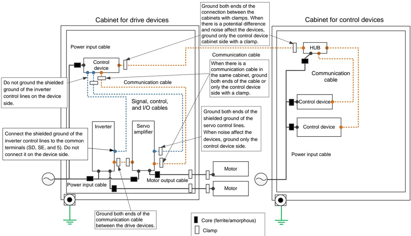
Fig. 13 Grounding of signal, control, and I/O shielded cables and communication cables
