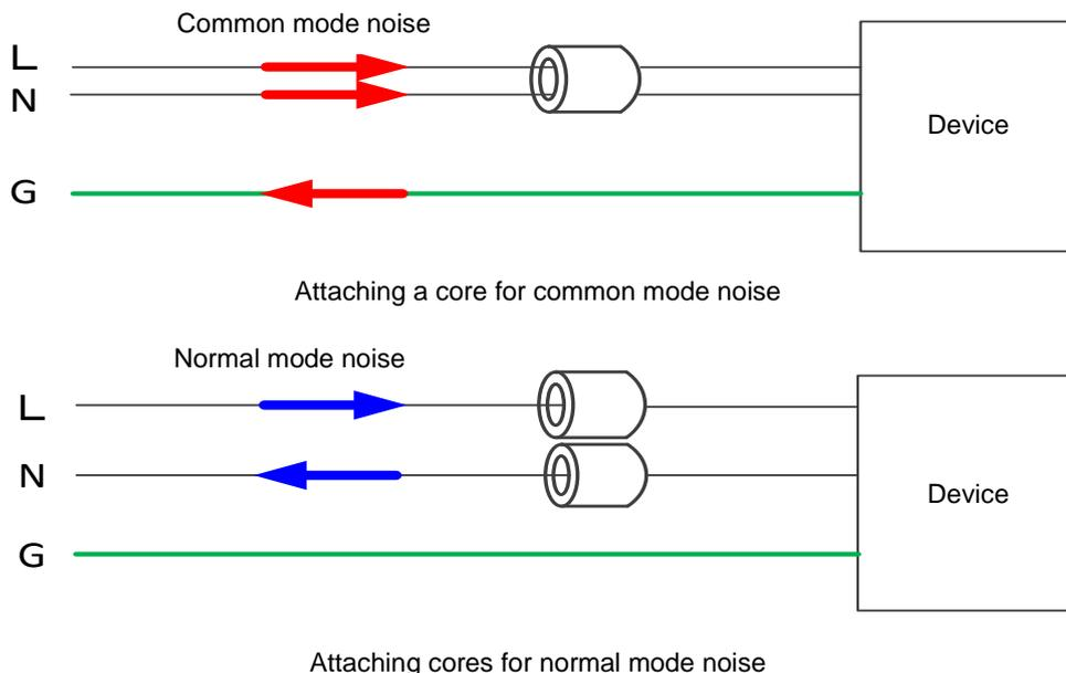
Fig. 19. Effective attachment of ferrite core or amorphous core
