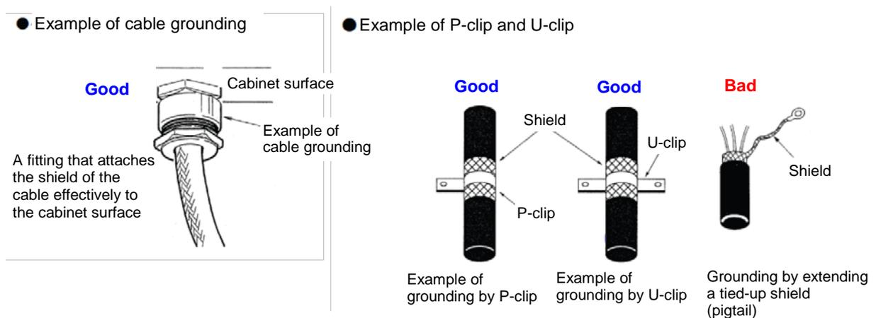
A cable clamp fitting is composed of a ground plate and a cable clamp.
