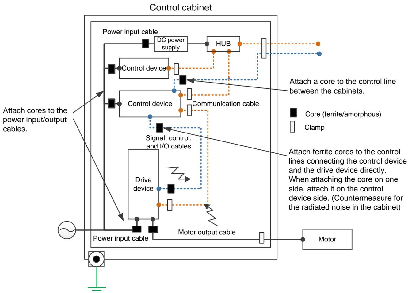
Fig. 20. Attachment position of ferrite core and amorphous core
