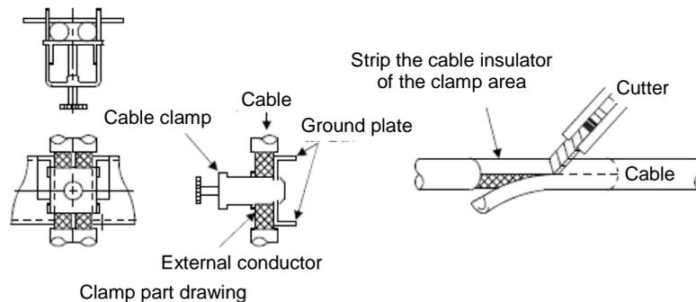
Fig. 12. Termination process of shielded cable
