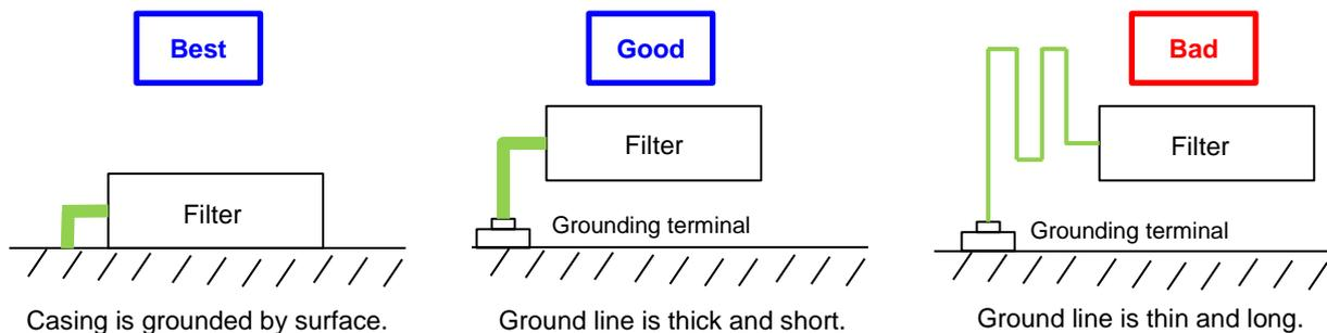
Fig. 22. Caution for installing EMC noise filter (2)
