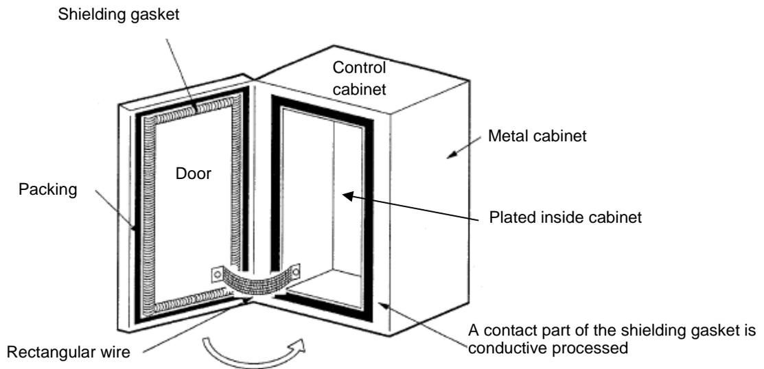
Fig. 16 Example of control cabinet with EMC countermeasures
