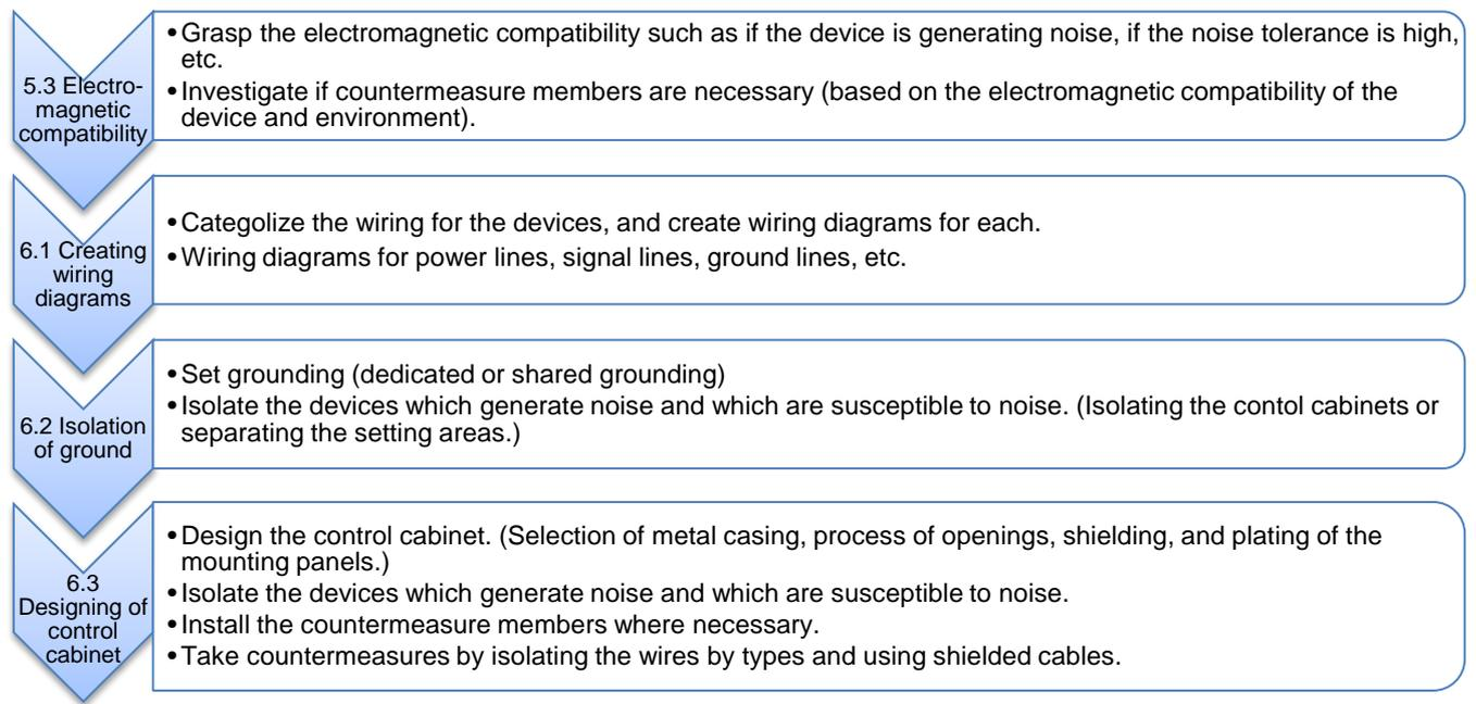
Fig. 6. Flow of designing control cabinet
