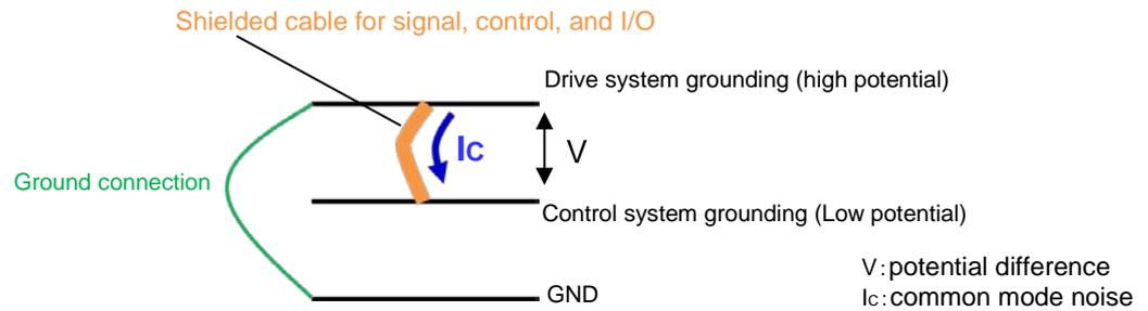
Fig. 14 Noise transmission mechanism of grounding lines of shielded cable
