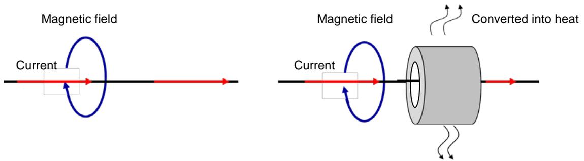
Fig. 18. Characteristics of ferrite core and amorphous core
