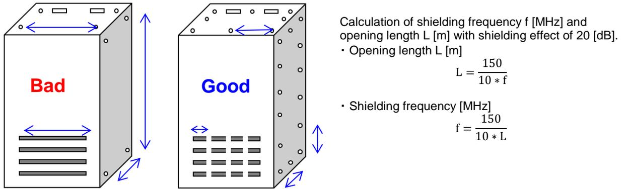
When the long side (indicated by  $\leftrightarrow$ ) of the opening is welded or screwed with an interval of 100 mm or shorter, noise of 150 kHz or less is shielded by 20 dB or more.
