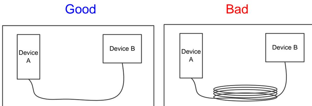
Fig. 8. Processing of extra length of cable
