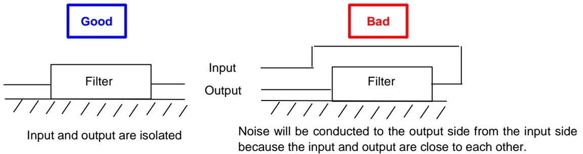
Fig. 21. Caution for handling EMC noise filter (1)
