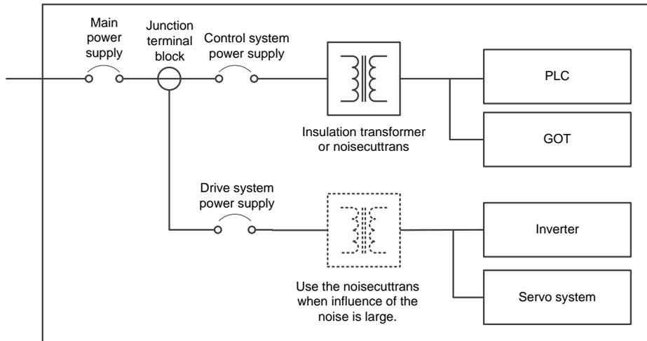
Fig. 23. Connection of insulation transformer or Noisecuttrans
