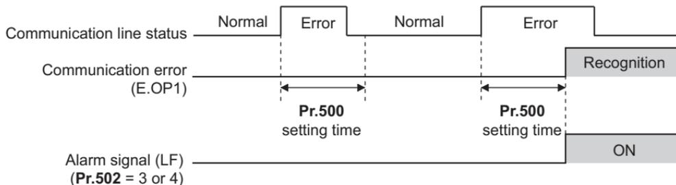
When a communication line error occurs and lasts longer than the time set in **Pr.500**, it is recognized as a communication error. If the communication returns to normal within the time, it is not recognized as a communication error, and the operation continues.
