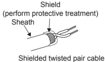
Strip the wires as follows. If too much of the wire is stripped, a short circuit may occur with neighboring wires. If not enough of the wire is stripped, wires may become loose and fall out. Twist the stripped end of wires to prevent them from fraying. Do not solder them.
