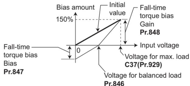
**Pr.840 = "2"** (at regeneration when the motor is in forward rotation)
