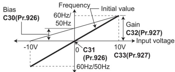
When **Pr.406** = "0, 5", terminal 6 acts as speed command or speed limit input and **C30 to C33** are used for calibration parameter.
