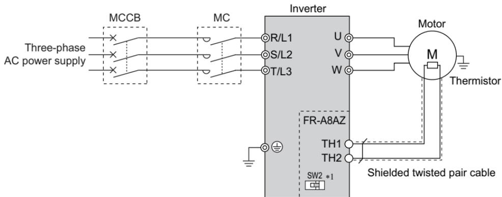
\*1 When calibrating the thermistor, change the switch for thermistor calibration. (Refer to [page 41](#))
