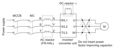
\*1 The converter unit (FR-CC2) is equipped with the DC reactor.
