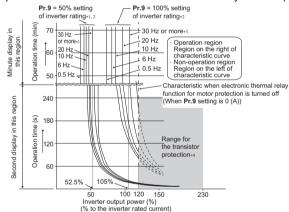
This function detects the overload (overheat) of the motor and trips the inverter by stopping the operation of the transistor at the inverter output side. (The operation characteristic is shown on the left.)
