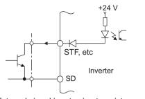
External signal input using transistor (sink logic)
