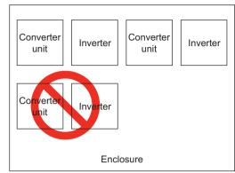
Arrangement of multiple inverters and converter units
