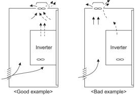
Arrangement of the ventilation fan and inverter
