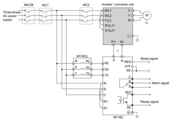
\*1 For wiring to terminals P/+ and N/- of the FR-F842-08660(400K) or lower inverters, up to two cables can be connected. For wiring to the terminals of the FR-F842-09620(450K) or higher inverters, up to four cables can be connected. To use more cables, use a bus bar.
