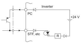
External signal input using transistor (source logic)
