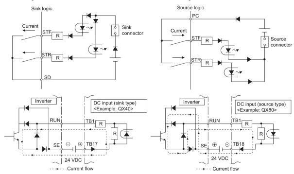
· When using an external power supply for transistor output
