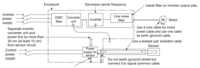
Do not earth (ground) enclosure directly. Do not earth (ground) control cable.
