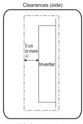
\*1 For replacing the cooling fan, 30 cm or more of space is necessary in front of the inverter. Refer to page 92 for fan replacement.
