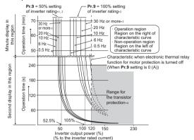
This function detects the overload of the motor, stops the operation of the inverter's output transistor, and stops the output. (The operation characteristic is shown on the left.)
