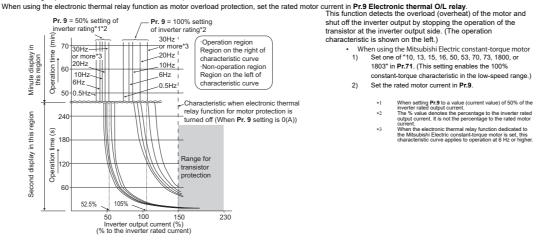
The internal accumulated heat value of the electronic thermal O/L relay is reset to the initial value by the inverter's power reset or reset signal input. Avoid unnecessary reset and power-OFF. Install an external thermal relay (OCR) between the inverter and motors to operate several motors, a multi-pole motor or a dedicated motor with one inverter
