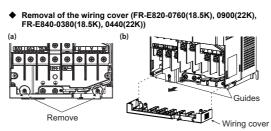
(a) Remove the mounting screws of the wiring cover. (b) Pull out the cover along the guides in the direction shown by the arrow in the (b) Tighten the mounting screws of the wiring cover (tightening torque: 0.6 to figure above
