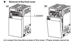
emoved.) (b) Pull out the cover using its lower side as a support. With the cover removed, the control circuit terminals can be wired and the plug-in option can be installed.
