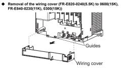
Reinstallation of the wiring cover (FR-E820-0240(5.5K) to 0600(15K), FR-E840-0230(11K), 0300(15K))
