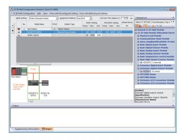
**6.** Select the high-speed counter module in "List of stations" on the "CC IE Field Configuration" window.
