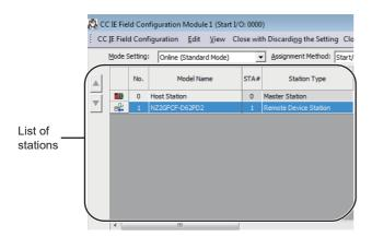
Select the high-speed counter module in "List of stations" on the "CC IE Field Configuration" window.
