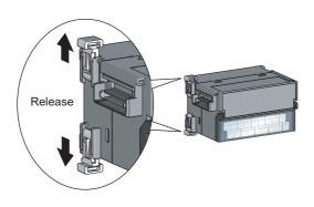
Release the module joint levers (two points) on the side of the extension module. Slide the levers vertically.
