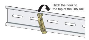
Hitch the upper hook of the DIN rail stopper to the top of the DIN rail.
