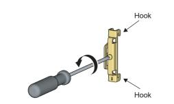
**5.** Hitch the bottom hook of the DIN rail stopper to the bottom of the DIN rail.
