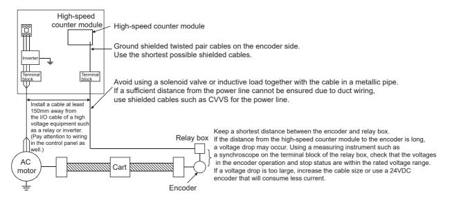
Ground the shielded twisted pair cable on the encoder side (relay box). (Wiring example: with a sink type encoder (24V))
