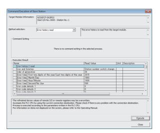
**6.** The error history of the high-speed counter module is displayed in "Execution Result".
