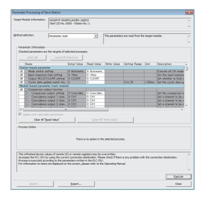
10. Click the [Execute] button to write the parameter to the high-speed counter module.
