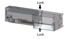
4. Lock the module joint levers (two points) on the side of the extension module. Slide the levers toward the module. Check that the modules are securely connected.
