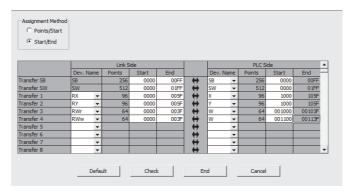
20. Write the set parameter to the CPU module of the master station and reset the CPU module.
