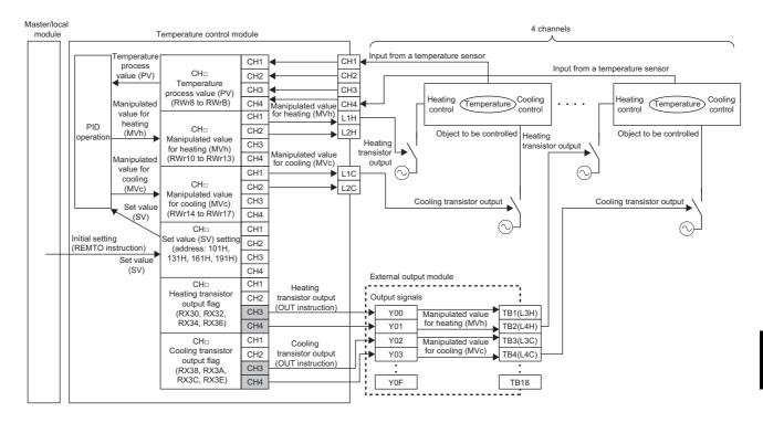
Ex. A program in which CH3 Heating transistor output flag (RX34) is assigned to Y0 of an output module Assign a refresh parameter as shown below.
