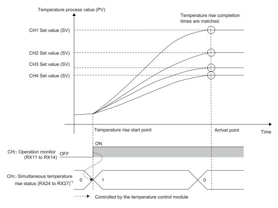
\*1 This becomes Simultaneous temperature rise in process (1) when the temperature rise starts; however, it becomes Simultaneous temperature rise not in process (0) before the temperature rise starts.
