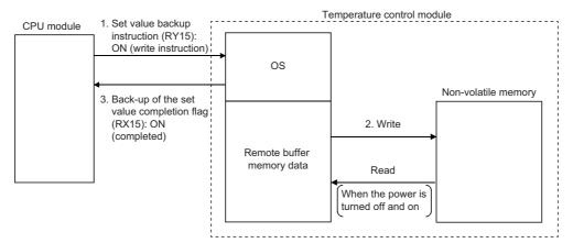
If data write to non-volatile memory does not complete, Back-up of the set value fail flag (RX17) turns on.
