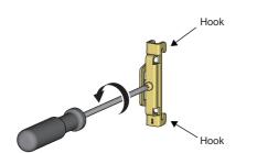
3. Loosen the screw on the DIN rail stopper.
