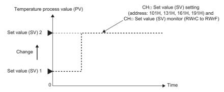
When the setting change rate limiter is specified: The value in CH□ Set value (SV) monitor (RWrC to RWrF) follows the set value (SV) of after the setting is reflected.
