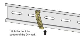
**4.** Hitch the lower hook of the DIN rail stopper to the bottom of the DIN rail.
