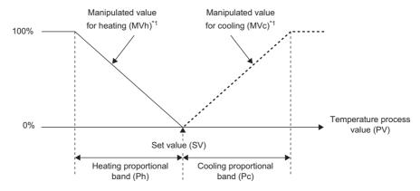
\*1 The value actually output is within the output limiter range set in CH $\square$  Heating upper limit output limiter (address: 105H, 135H, 165H, 195H) and CH $\square$  Cooling upper limit output limiter (address: 1C5H, 1CAH, 1CFH, 1D4H). ( $\square$  Page 321, Appendix 3 (10))
