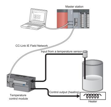
Ex. Heating-cooling control (heating and cooling)
