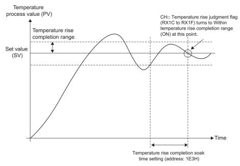
Set the temperature rise completion range and temperature rise completion soak time in the following remote buffer memory areas.
