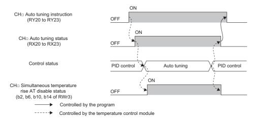
The temperature control module turns CH□ Simultaneous temperature rise AT disable status (b2, b6, b10, b14 of RWr3) to 1 (ON). With CH□ Auto tuning status (RX20 to RX23) on, the module performs the same processing as normal auto tuning.
