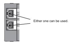
• When two connectors are used in line topology or ring topology, an Ethernet cable can be connected to the connectors in any combination. For example, the cable can be connected between PORT1s and between PORT1 and PORT2.
