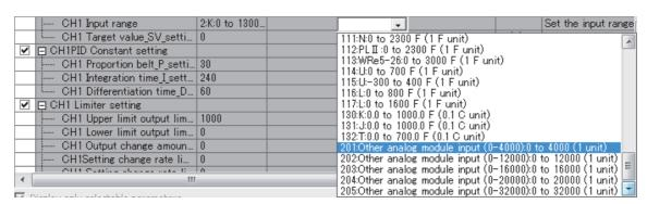
3. Store the value of another analog module (such as an A/D converter module) into CH□ Temperature process value for input with another analog module (PV) (RWw0 to RWw3).
