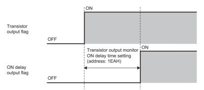
Transistor output monitor ON delay time setting (address: 1EAH) enables setting considering delay time (response/scan time delay) of actual transistor output. ( Page 345, Appendix 3 (41)) Transistor output monitor ON delay time setting (address: 1EAH) can be used to create a program to monitor the ON delay output flag and external output and judge the disconnection of transistor output.
