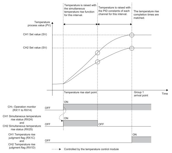
The signal does not turn to Simultaneous temperature rise not in process (OFF) at the completion of the temperature rise. As in the figure above, the temperature is raised to a certain point with the simultaneous temperature rise function, and the signal remains Simultaneous temperature rise in process (ON) for that interval. After that the temperature is raised with the PID constants of each channel, and the signal turns to Simultaneous temperature rise not in process (OFF).
