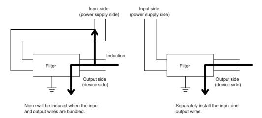
• Ground the noise filter grounding terminal to the control panel with the shortest cable possible (approx. 10cm).
