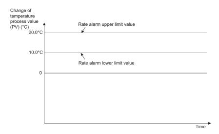
Ex. A setting of the rate alarm upper limit value and lower limit value to monitor that the temperature process value (PV) is falling within the specified range
