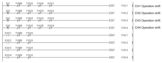
• Program that executes the auto tuning and backs up the PID constants in the non-volatile memory if the auto tuning is normally completed (program that stops the auto tuning when an alert is detected)
