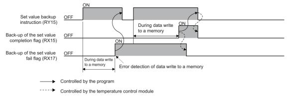
The signal turns off when Set value backup instruction (RY15) is turned on again and the data writing to the non-volatile memory is normally completed.
