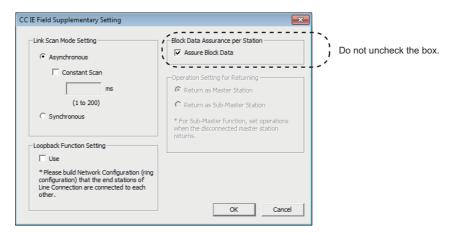
Do not set the parameter using the CCPASET instruction in the master station. If the CCPASET instruction is executed, correct operation of the temperature control module cannot be guaranteed because the module operates with the block data assurance per station disabled. (The CCPASET instruction is used to set parameter to a master/local module. For details on the CCPASET instruction, refer to the following.
