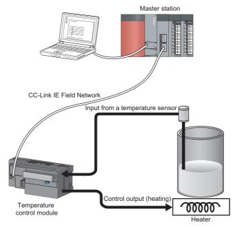
· Heating-cooling control (heating and cooling)
