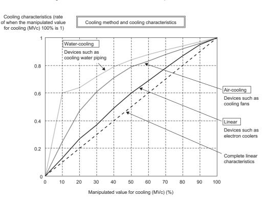
PID constants are calculated and executed based on this setting during auto tuning; therefore, more appropriate PID constants can be found by setting more applicable cooling characteristic of a device.
