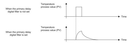
For the primary delay digital filter, set the time until the temperature process value (PV) changes by 63.3% (time constant).
