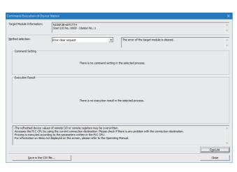
The process "Error clear request" will be executed. The operation of the device station may be changed by the execution of the process "Error clear request". Also it may overwrite the device value of the PLC CPU refreshing the remote I/O and remote registers. Please confirm safety before the execution.
