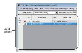
1. Select the temperature control module in "List of stations" on the CC IE Field Configuration window.
