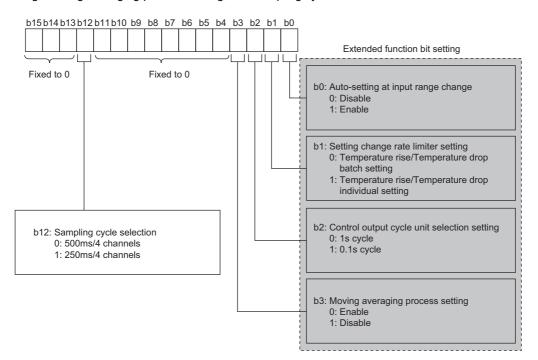
To enable these settings, turn off and on Initial data setting request flag (RY9) while the operations of all channels are stopped.
