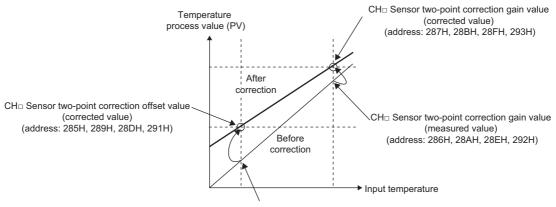
CH□ Sensor two-point correction offset value (measured value) (address: 284H, 288H, 28CH, 290H)
