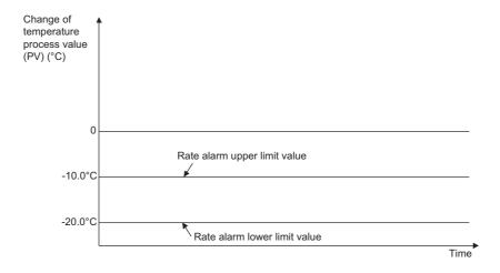
Ex. A setting of the rate alarm upper limit value and lower limit value to monitor that the temperature process value (PV) is changing within the specified range
