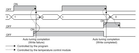
When the data writing to the non-volatile memory is completed normally, CH Write completion flag (address: b4 to b7 of 1104H) turns on.
