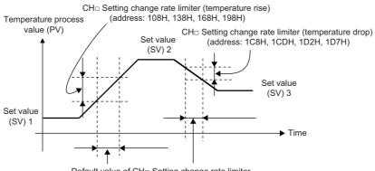
Default value of CH□ Setting change rate limiter unit time setting (address: 109H, 139H, 169H, 199H)
