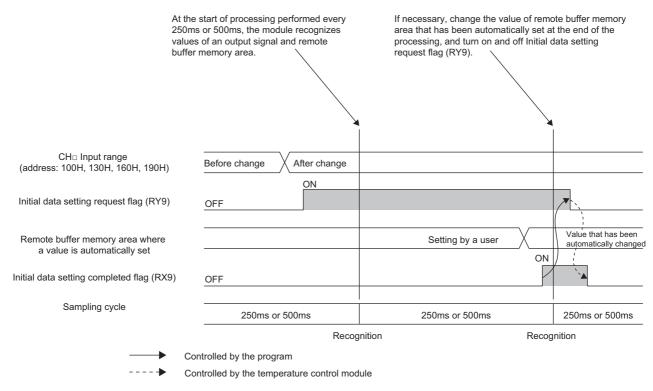
The sampling cycle differs depending on the setting of "Sampling cycle selection". ( Page 310, Section (1) (e))
