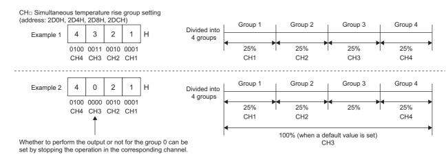
In Example 2, the maximum number of groups is four; therefore, timing is divided into four timing. Because no channel is set for Group 3, no channel starts transistor output at the timing for Group 3.
