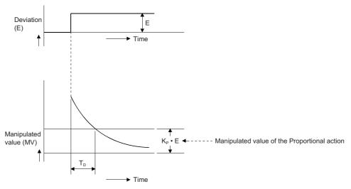
The derivative action is used as a PD action in combination with a proportional action, or a PID action in combination with a proportional action and an integral action. The derivative action cannot be used by itself.
