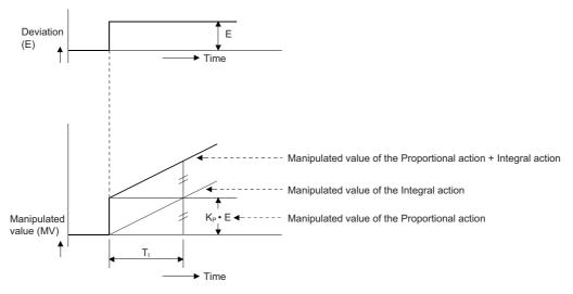
The integral action is used as a PI action in combination with a proportional action, or a PID action in combination with a proportional action and a derivative action. The integral action cannot be used by itself.
