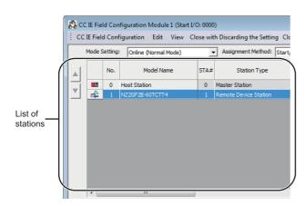
Select the temperature control module in "List of stations" on the CC IE Field Configuration window.
