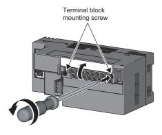
Open the terminal cover and loosen the terminal block mounting screws (two points).
