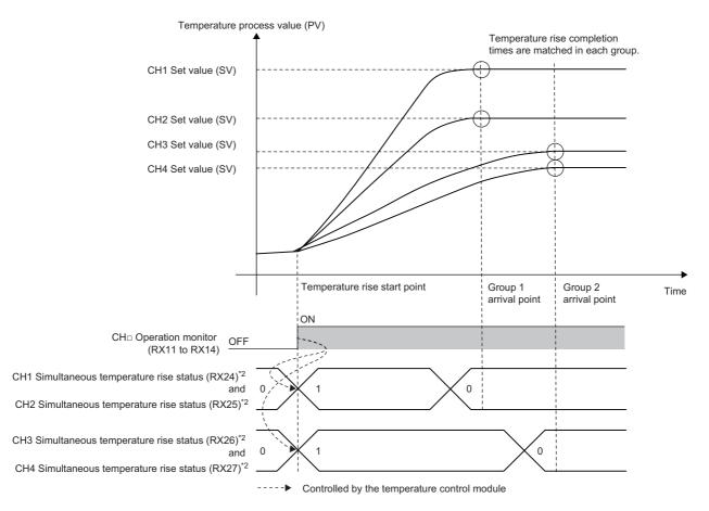
\*2 This becomes Simultaneous temperature rise in process (1) when the temperature rise starts; however, it becomes Simultaneous temperature rise not in process (0) before the temperature rise starts.
