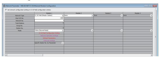
3. Display the CC IE Field Configuration window and configure the configuration and station number of the device station as follows.
