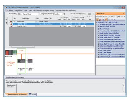
**6.** On the "CC IE Field Configuration" window, from "List of stations", select the main D/A converter module.
