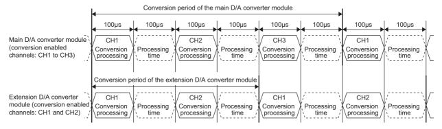
Conversion period of the main D/A converter module = (Conversion speed  $(100\mu s)$  + Processing time  $(100\mu s)$ ) × 3 =  $600\mu s$  Conversion period of the extension D/A converter module = (Conversion speed  $(100\mu s)$  + Processing time  $(100\mu s)$ ) × 2 =  $400\mu s$
