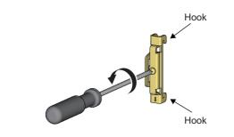
Hitch the bottom hook of the DIN rail stopper to the bottom of the DIN rail.
