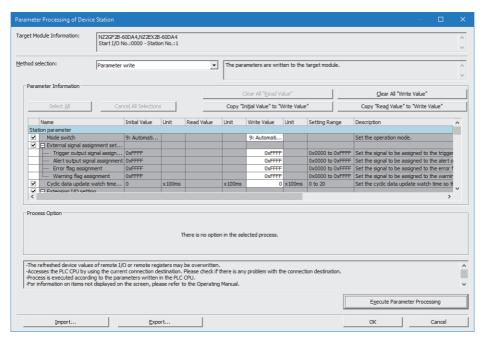
**10.** Click Execute Parameter Processing button to write the parameters to the D/A converter module.
