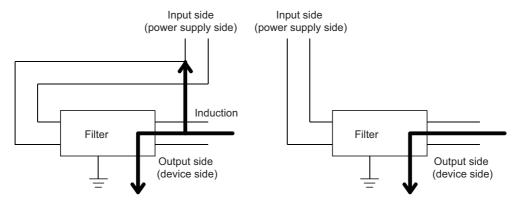
Noise is induced if an input line and an output line are bundled.
