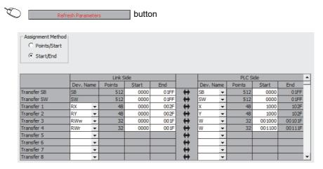
**6.** Write the set parameters to the CPU module of the master station, and reset the CPU module, or turn off and on the power supply.
