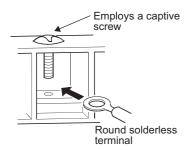
1. Loosen the terminal screw. A round solderless terminal can be connected as it is.
