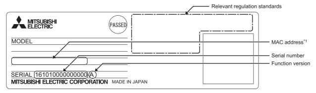
\*1 The extension D/A converter module does not have a MAC address.
