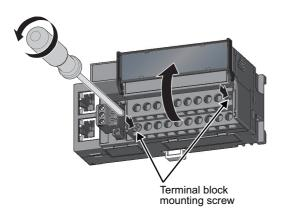
1. Open the terminal block cover and loosen the terminal block mounting screws (two points).
