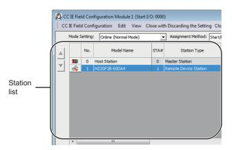
On the "CC IE Field Configuration" window, select the main D/A converter module from "List of stations".
