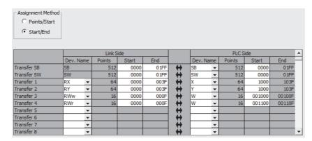
20. Write the set parameters to the CPU module of the master station, and reset the CPU module.
