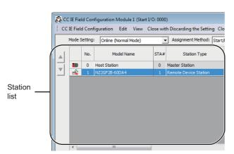
On the "CC IE Field Configuration" window, from "List of stations", select the main D/A converter module.
