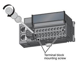
2. Tighten the terminal block mounting screws.
