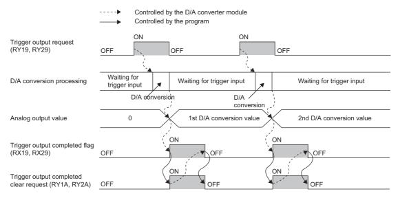
Even when Trigger output completed clear request (RY1A, RY2A) is turned on while Trigger output completed flag (RX19, RX29) is on, the D/A converter module accepts the trigger output request.
