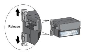
2. Release the module joint levers (two points) on the side of the extension module. Slide the levers vertically.
