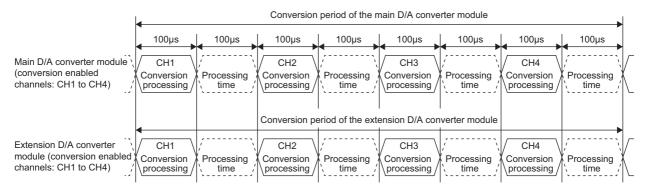
Conversion period of the main D/A converter module =  $(100\mu s + 100\mu s) \times 4 = 800\mu s$ Conversion period of the extension D/A converter module =  $(100\mu s + 100\mu s) \times 4 = 800\mu s$
