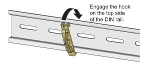
**6.** Hitch the upper hook of the DIN rail stopper to the top of the DIN rail.
