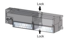
4. Lock the module joint levers (two points) on the side of the extension module. Slide the levers toward the module.
