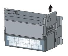
Remove the cover on the side of the main module.
