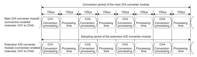
Conversion period of the main D/A converter module =  $(100\mu s + 100\mu s) \times 4 = 800\mu s$ Sampling period of the extension A/D converter module =  $(100\mu s + 100\mu s) \times 4 = 800\mu s$
