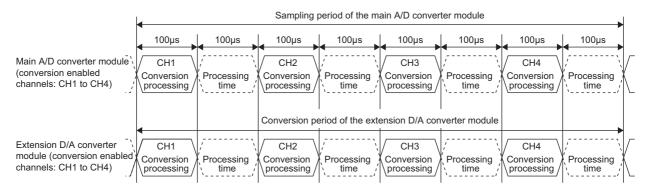
Sampling period of the main A/D converter module =  $(100\mu s + 100\mu s) \times 4 = 800\mu s$ Conversion period of the extension D/A converter module =  $(100\mu s + 100\mu s) \times 4 = 800\mu s$
