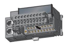
Open the terminal block cover to install the twopiece terminal block.
