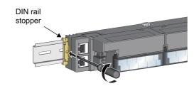
8. Hold the DIN rail stopper in the direction opposite to the arrow on the stopper and tighten the screw with a screwdriver.
