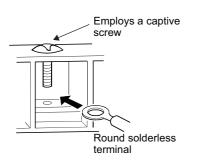
**1.** Loosen the terminal screw. A round solderless terminal can be connected as it is.
