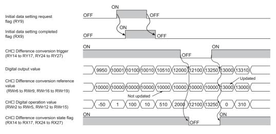
Before CH□ A/D conversion completed flag (RX10 to RX13, RX20 to RX23) turns on from off by turning on Initial data setting request flag (RY9) from off, changing CH□ Difference conversion trigger (RY14 to RY17, RY24 to RY27) from No request (OFF) to Trigger request (ON) results in operation with the difference conversion reference value taking on the digital operation value at the time when CH□ A/D conversion completed flag (RX10 to RX13, RX20 to RX23) turns on from off.
