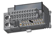
**1.** Open the terminal block cover to install the twopiece terminal block.
