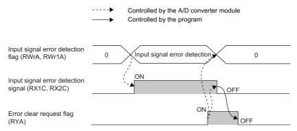
Check that Input signal error detection signal (RX1C, RX2C) is off before turning off Error clear request flag (RYA) from on. Turning on and off Error clear request flag (RYA) before Input signal error detection signal (RX1C, RX2C) turns off does not allow Input signal error detection signal (RX1C, RX2C) to be cleared.
