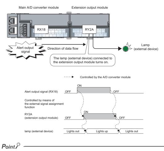
Assigning a remote input signal of the main A/D converter module to a remote output signal of the extension output module does not allow the assigned remote output signal to be turned on/off or monitored by program. Change or monitor the preassigned remote input signal of the main module. (In the above example, change or monitor Alert output signal (RX18).)
