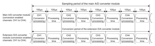
Sampling period of the main A/D converter module =  $(100\mu s + 100\mu s) \times 4 = 800\mu s$ Sampling period of the extension D/A converter module =  $(100\mu s + 100\mu s) \times 4 = 800\mu s$
