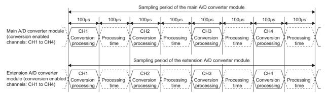
Sampling period of the main A/D converter module =  $(100\mu s + 100\mu s) \times 4 = 800\mu s$ Sampling period of the extension A/D converter module =  $(100\mu s + 100\mu s) \times 4 = 800\mu s$
