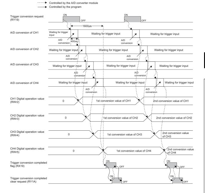
**Ex.** Operation until Trigger conversion completed flag (RX19) turns on from off after turning on Trigger conversion request (RY19) from off, with the main A/D converter module set to the following conditions:
