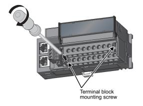
**2.** Tighten the terminal block mounting screws.
