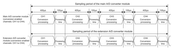
Sampling period of the main A/D converter module =  $(400\mu s + 100\mu s) \times 4 = 2000\mu s = 2ms$ Sampling period of the extension A/D converter module =  $(400\mu s + 100\mu s) \times 4 = 2000\mu s = 2ms$
