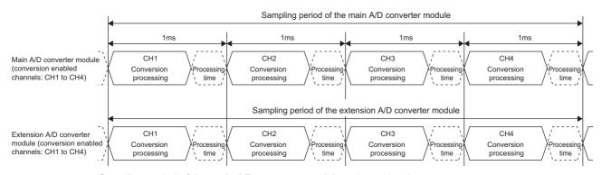
Sampling period of the main A/D converter module =  $1 \text{ms} \times 4 = 4 \text{ms}$ Sampling period of the extension A/D converter module =  $1 \text{ms} \times 4 = 4 \text{ms}$
