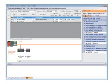
**6.** On the "CC IE Field Configuration" window, from "List of stations", select the main A/D converter module.
