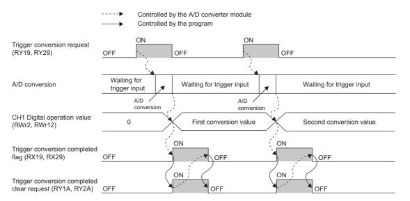
Even while Trigger conversion completed flag (RX19, RX29) is on, turning on Trigger conversion completed clear request (RY1A, RY2A) from off allows the A/D converter module to accept a trigger conversion request and then update the digital operation value.
