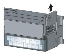
**1.** Remove the cover on the side of the main module. Save the removed cover without losing it.
