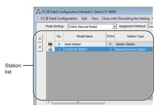
On the "CC IE Field Configuration" window, from "List of stations", select the main A/D converter module.
