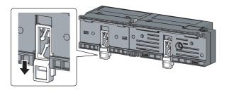
1. Pull down all DIN rail hooks on the back of the modules.
