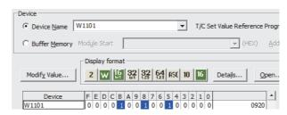
5. The A/D converter module starts operating in the set drive mode by turning off and on the module power supply or performing remote reset.
