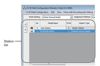
1. On the "CC IE Field Configuration" window, from "List of stations", select the main A/D converter module.
