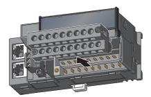
**1.** Open the terminal block cover and loosen the terminal block mounting screws (two points).
