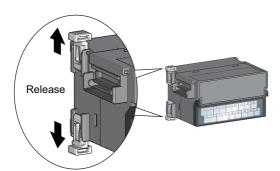
2. Release the module joint levers (two points) on the side of the extension module. Slide the levers vertically.
