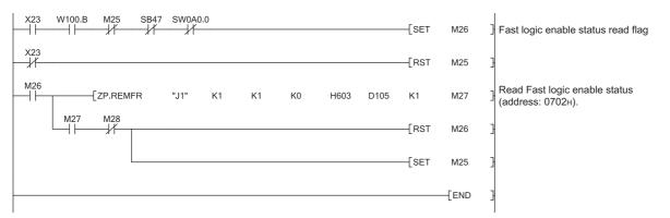
**2.** Write the program to the CPU module of the master station, and reset the CPU module, or turn off and on the power supply.
