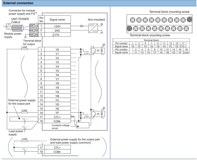
\*5 Only one wire can be connected to a terminal of the terminal block for module power supply and FG. Multiple wires cannot be connected to a terminal. Connecting two or more wires may cause a poor contact.
