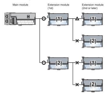
(1) Extension module that supports the connection of multiple extension modules
