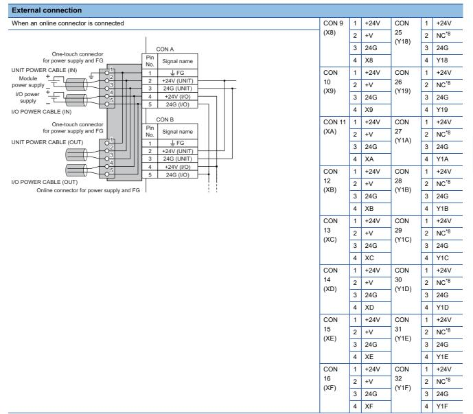
\*7 A non-wired connector must be connected to the empty slot of the connector for power supply and FG.
