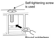
**1.** Loosen the terminal screw. Connect the round solderless terminal as it is.
