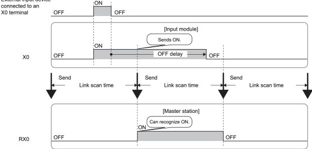
When the ON time of the target input signal is less than  $100\mu s$ , the module cannot recognize ON of the input and the input OFF delay function may not be performed.
