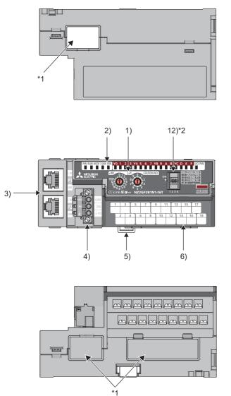
\*1 Do not remove this seal because it is used for a maintenance purpose.
