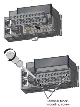
**1.** Open the terminal cover to install the terminal block.
