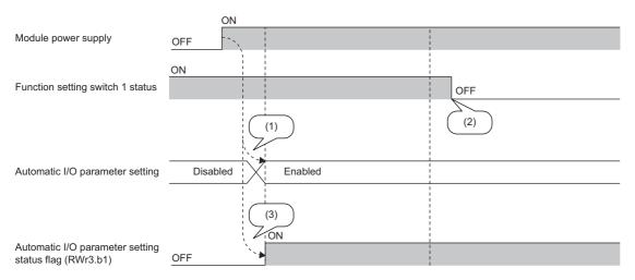
(1) The automatic I/O parameter setting is enabled or disabled depending on the status of the function setting switch 1 at power-on.
