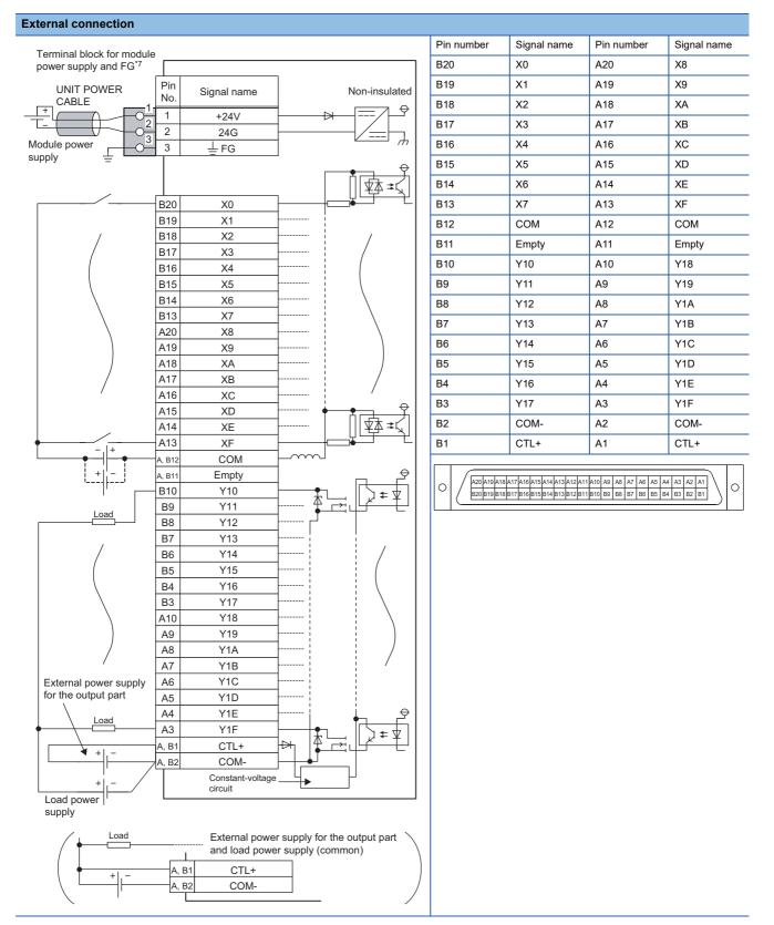
\*7 Only one wire can be connected to a terminal of the terminal block for module power supply and FG. Multiple wires cannot be connected to a terminal. Connecting two or more wires may cause a poor contact.
