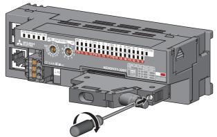
**2.** Tightening connector screws Tighten two connector screws (M2.6 screw).
