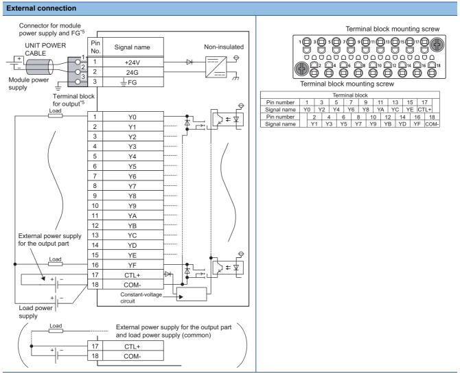
\*5 Only one wire can be connected to a wire insertion opening. Multiple wires cannot be connected to a terminal. Connecting two or more wires may cause a poor contact.
