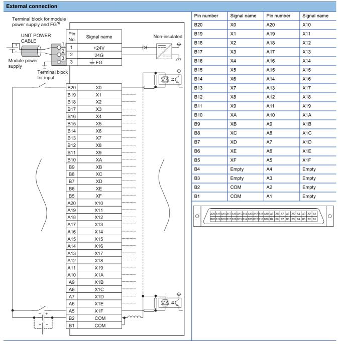
\*6 Only one wire can be connected to a terminal of the terminal block for module power supply and FG. Multiple wires cannot be connected to a terminal. Connecting two or more wires may cause a poor contact.
