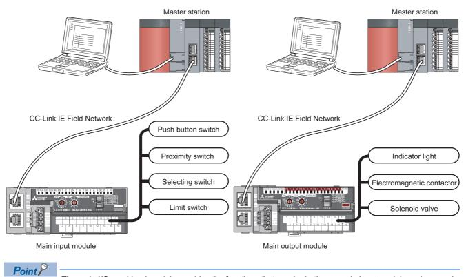
The main I/O combined module provides the functions that require both one main input module and one main output module.
