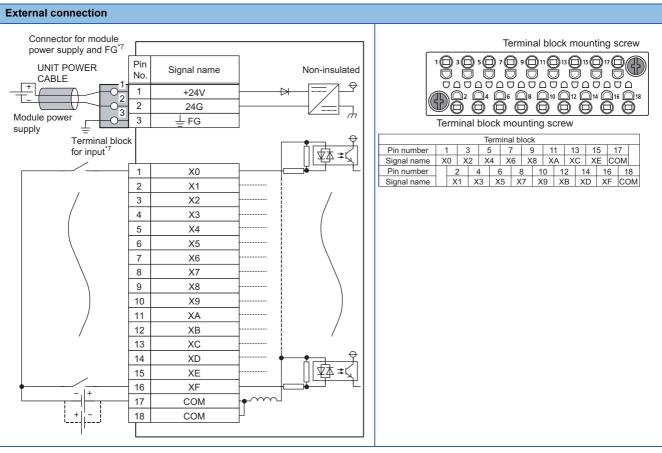
\*7 Only one wire can be connected to a wire insertion opening. Multiple wires cannot be connected to a terminal. Connecting two or more wires may cause a poor contact.
