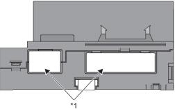
\*1 Do not remove this seal because it is used for a maintenance purpose.
