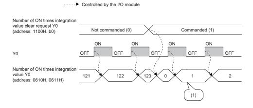
(1) The integration function is executed even when Number of ON times integration value clear command Y0 (address: 1100H.b0) is Commanded (1).
