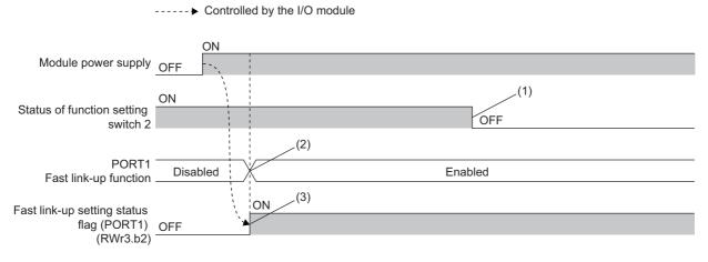
(1) The status of the fast link-up function (enabled/disabled) does not change even if the status of the function setting switch 2 changes during operation.
