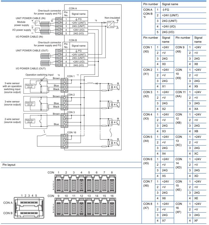
\*6 A non-wired connector must be connected to the empty slot of the connector for power supply and FG.
