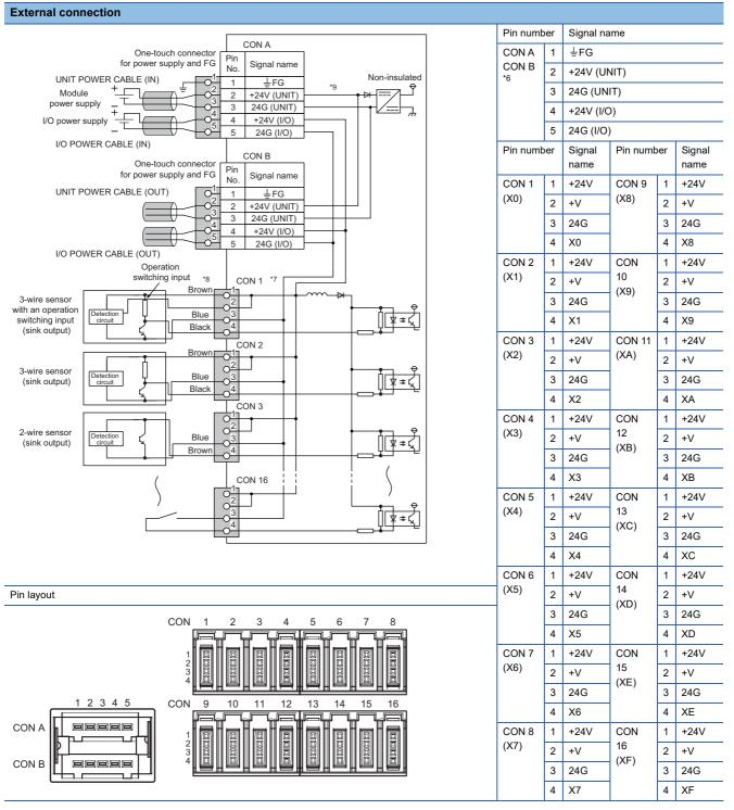
\*6 A non-wired connector must be connected to the empty slot of the connector for power supply and FG.
