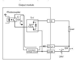
When the external power supply is powered on rapidly, the current (Ic) flows due to the stray capacitance(C). The current (Ic) flows to the gate of the transistor (Tr1) of the next stage and the output Y0 turns on for approximately  $100\mu$ s.
