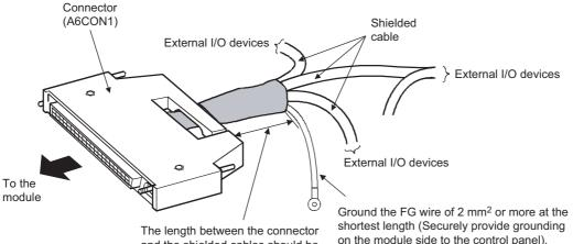
and the shielded cables should be the shortest possible.
