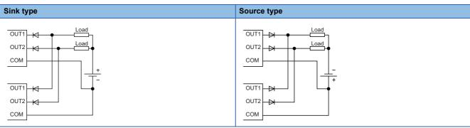
· When providing another circuit in parallel with a transistor output module
