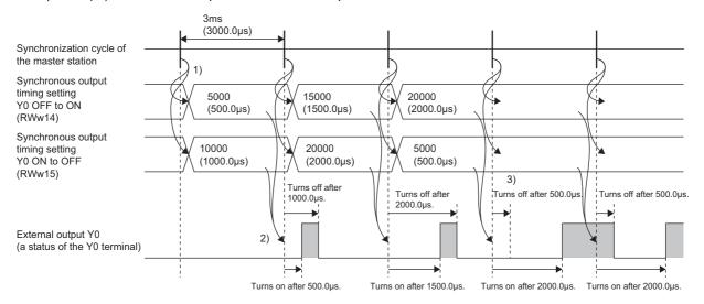
1)Synchronous output timing setting Y0 OFF to ON (RWw14) and Synchronous output timing setting Y0 ON to OFF (RWw15) are received at the change timing of the synchronization cycle of the master station.
