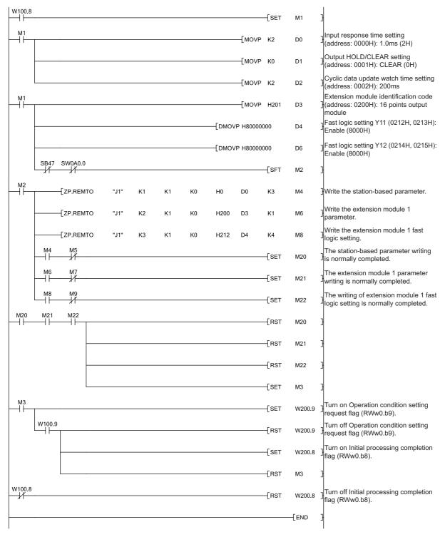
**2.** Write the program to the CPU module of the master station, and reset the CPU module, or turn off and on the power supply.
