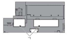
\*1 Do not remove this seal because it is used for a maintenance purpose.
