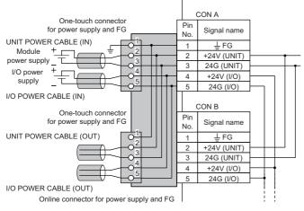
\*3 A non-wired connector must be connected to the empty slot of the connector for power supply and FG.
