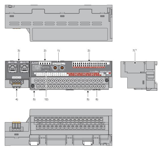
\*1 For the NZ2GF2B1-32D, NZ2GF2B1-32T, NZ2GF2B1-32TE, NZ2GF2B1-32DT, and NZ2GF2B1-32DTE, do not remove the cover because it is used for our maintenance purpose. If it is removed, a failure may occur.
