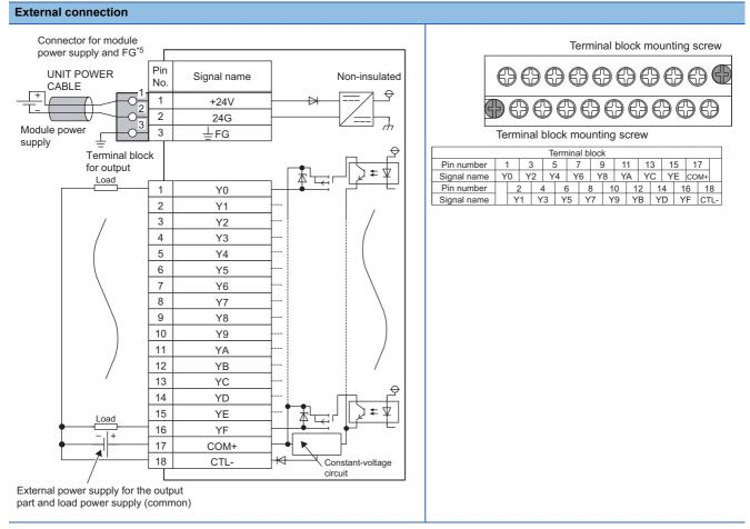
\*5 Only one wire can be connected to a terminal of the terminal block for module power supply and FG. Multiple wires cannot be connected to a terminal. Connecting two or more wires may cause a poor contact.
