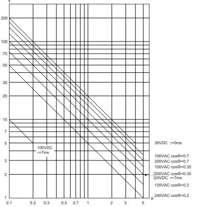
Use environment **Contact switching life** Rated switching voltage/current load 100 thousand times 1.5A at 200VAC, 1A at 240VAC (COS = 0.7) 100 thousand times 0.4A at 200VAC, 0.3A at 240VAC (COS = 0.7) 300 thousand times 1A at 200VAC, 0.5A at 240VAC (COS = 0.35) 100 thousand times 0.3A at 200VAC, 0.15A at 240VAC (COS = 0.35) 300 thousand times 1A at 24VDC, 0.1A at 100VDC (L/R = 7ms) 100 thousand times 0.3A at 24VDC, 0.03A at 100VDC (L/R = 7ms) 300 thousand times
