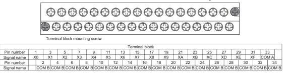
\*3 Only one wire can be connected to a terminal of the terminal block for module power supply and FG. Multiple wires cannot be connected to a terminal. Connecting two or more wires may cause a poor contact.
