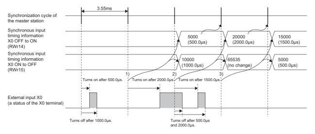
1)A value is stored in Synchronous input timing information X0 OFF to ON (RWr14) and Synchronous input timing information X0 ON to OFF (RWr15) at the change timing of the synchronization cycle of the master station.
