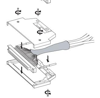
**1.** Loosen four screws of the connector and remove the screws. Then, open the connector cover from the connector side.
