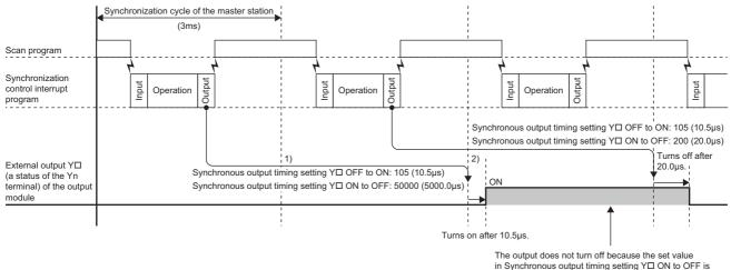
in Synchronous output timing setting  $Y\square$  ON to OFF is longer than the synchronization cycle of the master station.
