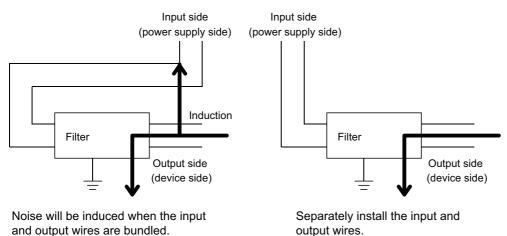
• Ground the noise filter grounding terminal to the control panel with the shortest cable possible (approx. 10cm).
