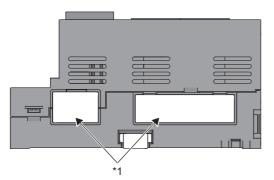
\*1 Do not remove this seal because it is used for a maintenance purpose.
