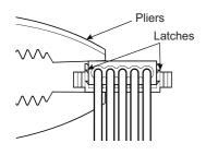
**1.** Check that the plug cover is engaged with the plug body.
