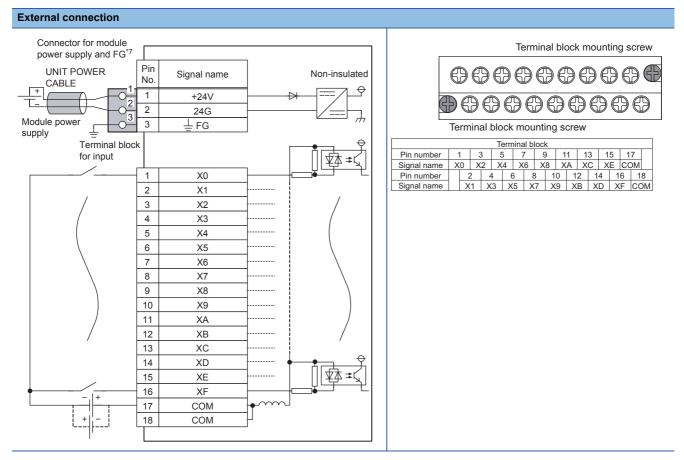
\*7 Only one wire can be connected to a terminal of the terminal block for module power supply and FG. Multiple wires cannot be connected to a terminal. Connecting two or more wires may cause a poor contact.
