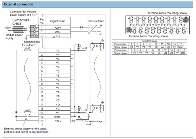
\*5 Only one wire can be connected to a wire insertion opening. Multiple wires cannot be connected to a terminal. Connecting two or more wires may cause a poor contact.
