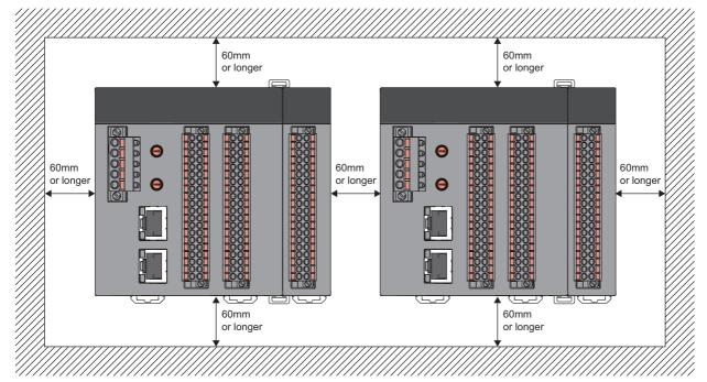
The figure above shows the examples for the NZ2GFSS2-32D and NZ2EXSS2-8TE.
