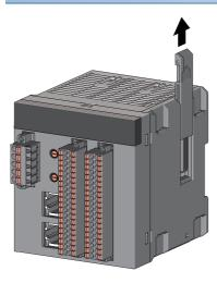
**1.** Remove the cover on the side of the module. Do not dispose of the removed cover, but store it.
