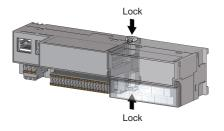
4. Lock the module joint levers (two points) on the side of the extension module. Slide the levers toward the module. Check that the extension module is securely connected after locking the levers.
