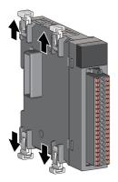
**2.** Release the module joint levers (four points) on the side of the extension module. Slide the levers to the outside of the module.
