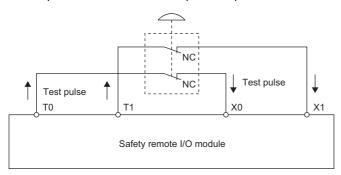
To use the input dark test function, use the test pulse output terminals (T0, T1, T2<sup>\*1</sup>, and T3<sup>\*1</sup>) and connect input devices. To use the input dark test function, use the input terminals and test pulse output terminals (T0, T1, T2<sup>\*1</sup>, and T3<sup>\*1</sup>) of the safety remote I/O module in the following combinations. An incorrect combination is regarded as a disconnection, and an error (input dark test error) occurs.
