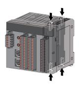
**4.** Lock the module joint levers (four points) on the side of the extension module. Slide the levers toward the module. Check that the extension module is securely connected after locking the levers.
