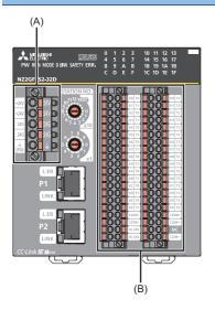
(A) Terminal block for module power supply and FG
