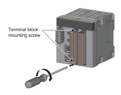
**2.** Tighten the terminal block mounting screws. Securely install the terminal block with the terminal block mounting screws. Failure to secure the terminal block may cause drop, short circuit, malfunction.
