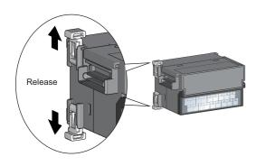
**2.** Release the module joint levers (two points) on the side of the extension module. Slide the levers to the outside of the module.
