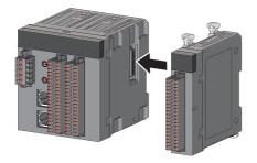
Insert the connector of the extension module into that of the main module so that they are securely engaged. Do not tilt the extension module when inserting the connector.
