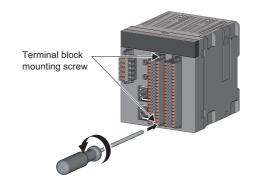
**1.** Loosen the terminal block mounting screws.
