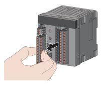
**2.** When the terminal block mounting screws are loosened, the terminal block can be removed.
