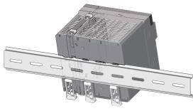
**2.** Hang the upper tabs of the module on a DIN rail, and push the module in position.
