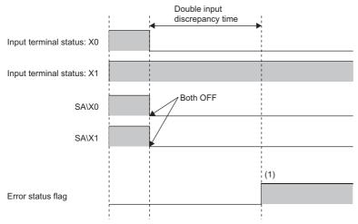
(1) After the double input discrepancy detection time elapses, a double input discrepancy detection error occurs.
