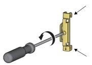
**4.** Loosen the screw on DIN rail stopper.
