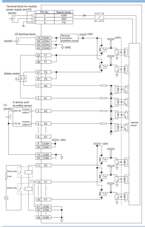
(1) The COM+ terminals can supply 24VDC as well.
