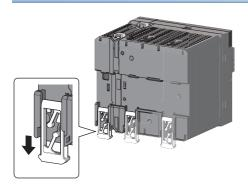
**1.** Pull down all DIN rail hooks on the back of the module. The hooks should be pulled down until they click.
