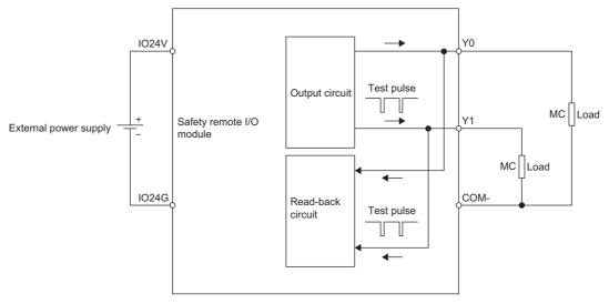
This function outputs test pulses to turn off the external output signal Y that is on and diagnoses the internal circuit for failure. Failures including circuit fixing and disconnection faults can be detected. The OFF time of test pulses and the number of pulse outputs used in one diagnostic can be set depending on the usage environment.
