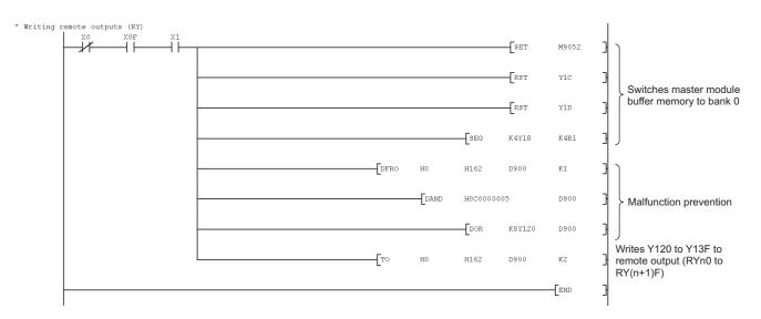
Figure 7.35 Program example for sending/receiving data with RISEND/RIRCV instruction (Continued)
