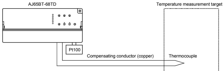
**(2) When performing cold junction compensation externally**
