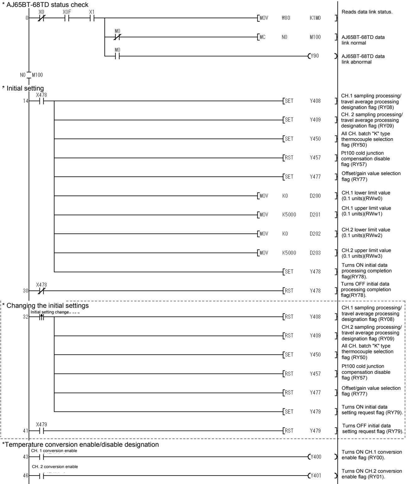
\*The program within the dotted frame is necessary only when the initial setting is changed.
