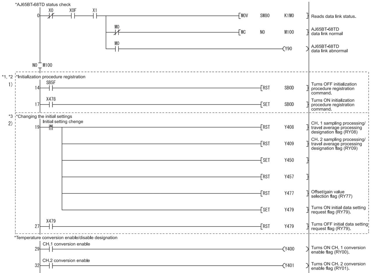
\*1: When making remote device station initialization procedure registration to multiple stations, correct the program within the dotted line 1) as shown below.
