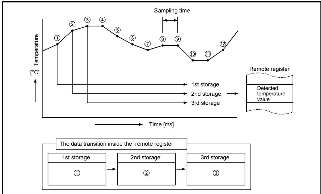
**(3) Changes caused by altering sampling processing/travel average processing settings**
