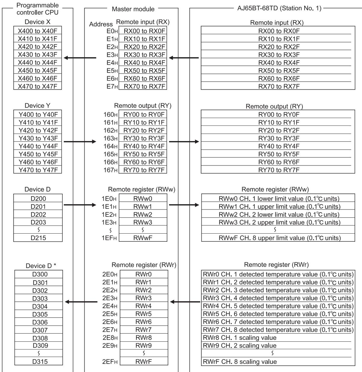
\* RWr0 to RWrF are assigned to D456 to D471 in the program example that uses the RRPA instruction (auto refresh parameter setting) on the ACPU/QCPU (A mode) (Refer to Section 5.5).
