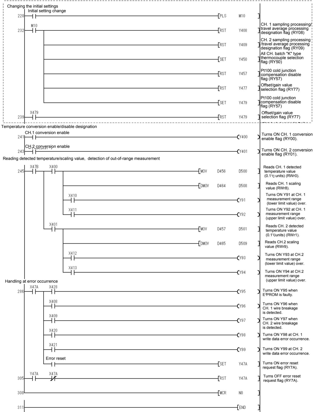
\*The program within the dotted frame is necessary only when the initial setting is changed.
