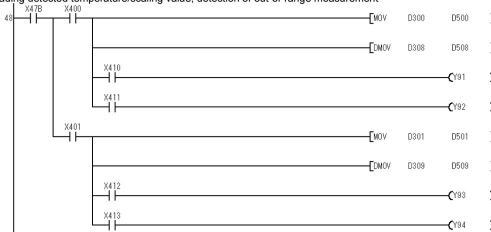
Reads CH. 1 detected temperature value (0.1°C units) (RWr0).
