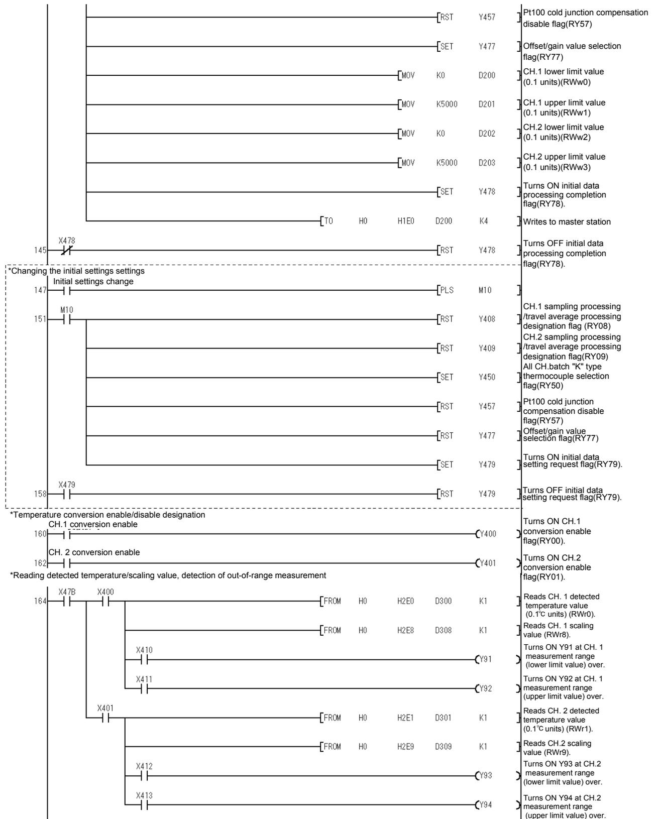
\*The program within the dotted frame is necessary only when the initial setting is changed.
