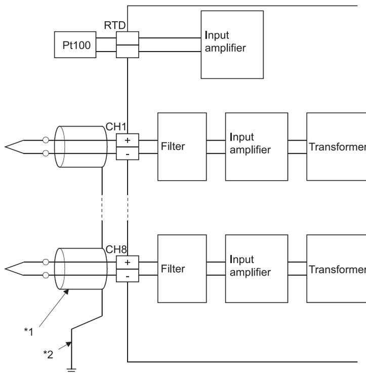
\*1 Be sure to use the shielded compensating conductor for the cable.
