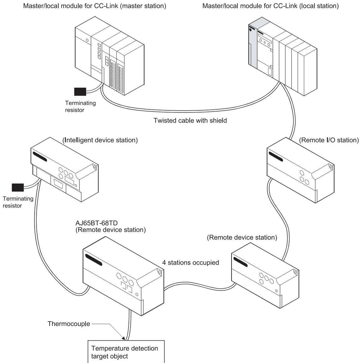
The maximum overall distance for the system is as follows (varies depending on transmission speed setting).
