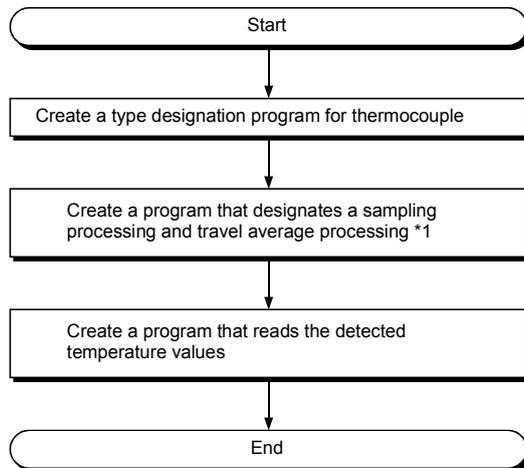
\*1 Only when executing error compensation with the value detected by travel average processing.
