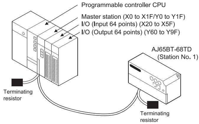
(2) Relationships between programmable controller CPU, master module and AJ65BT-68TD
