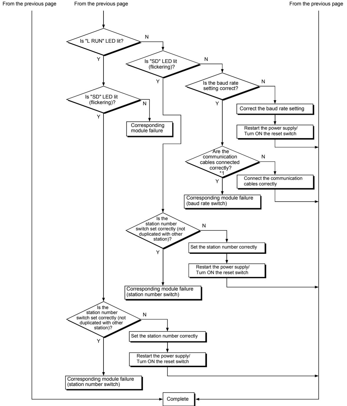
\*1 Check for short-circuits, reversed connection, wire breakage, terminal resistor, FG connection, overall distance and station-to-station distance.
