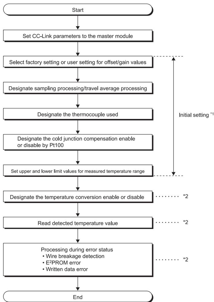
\*1 When the QCPU (Q mode) is used, initial setting can be made by the remote device station initialization procedure registration function. When the ACPU, QCPU (A mode) or QnACPU is used, use a sequence program to make the setting.
