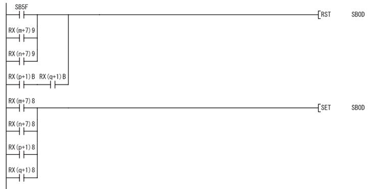
Note that the master module can register the initialization procedure of only the specified station out of the multiple remote device stations.
