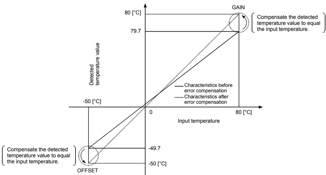
\* The error compensation may be executed using a standard DC voltage generator instead of inputting the temperature directly to a thermocouple.
