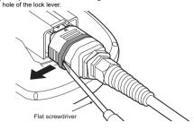
3) The external cable can be removed by pulling the whole plug connector while shifting the coupling of the plug connector to the cable side
