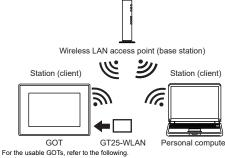
GOT2000 Series User's Manual (Hardware) For the setting and system configuration of wireless LAN function, refer to the
