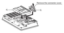
(5) Fix the CC-Link IE communication unit by tightening its mounting screws (4 places) with a tightening torgue of 0.36 to 0.48 N•m. (6) Fix the CC-Link IE communication unit by tightening two board fixing screws with a tightening torque of 0.36 to 0.48 N•m.
