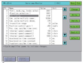
**5.** As the parameter setting window appears, enter the parameter setting with alphanumeric keys, and touch the [Enter] key to confirm the setting.
