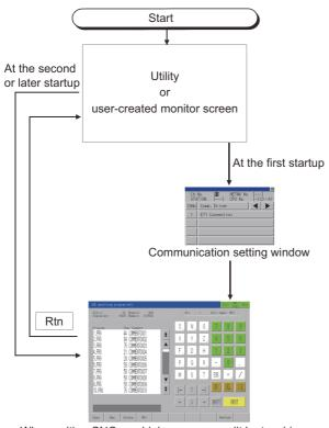
When exiting CNC machining program edit by touching Rtn, the last exited screen will be displayed at the next startup of CNC machining program edit.
