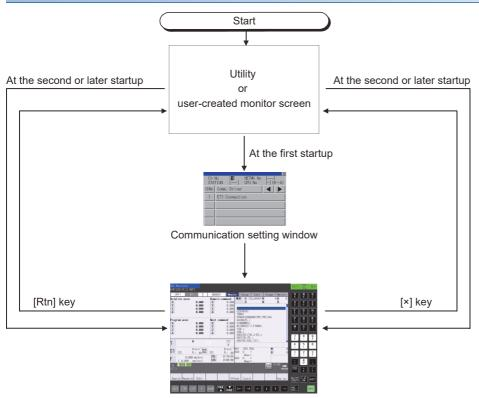
The initial screen specified with the special function switch appears at the next startup. If the initial screen is not specified, the last displayed screen appears at the next startup. For the details of the special function switch setting, refer to the following.
