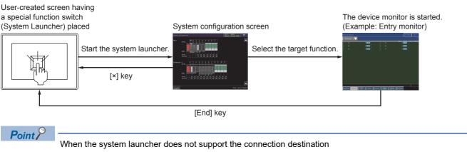
When the system launcher does not support the set connection destination, a dialog appears at the startup. For the details of the system launcher function, refer to the following.
