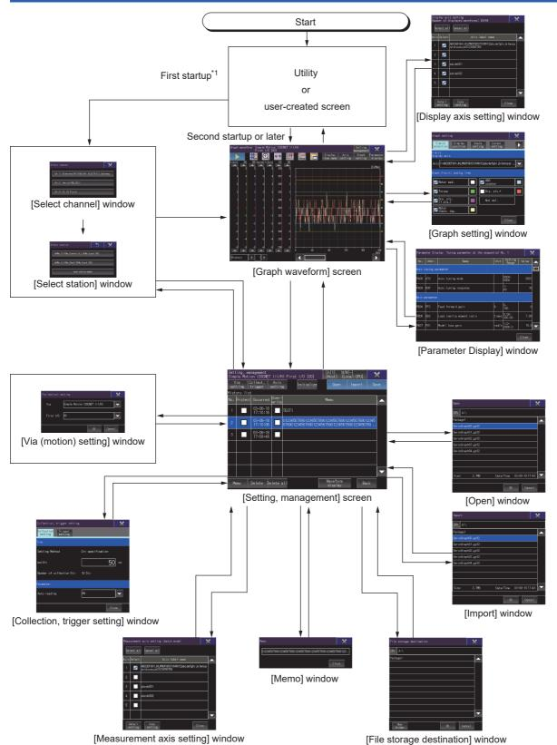
\*1 The [Graph waveform] screen appears at the first startup of the servo amplifier graph function, if the function is started with the special function switch in which the connection destination is specified.
