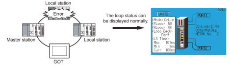
· When an error occurs in a local station which is not directly connected to a master station
