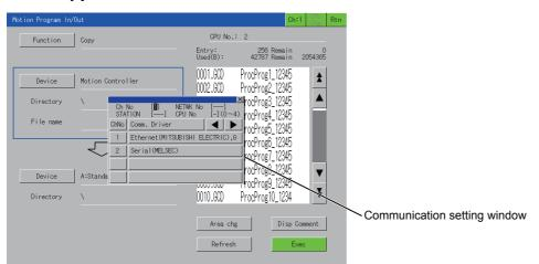
After the GOT is powered on, the communication setting window is displayed only at the first startup of the motion program I/ O.
