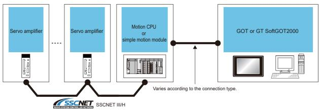
To connect a servo amplifier and the GOT through a Motion CPU (Q series), use a connection type other than the CC-Link IE Field Network connection.
