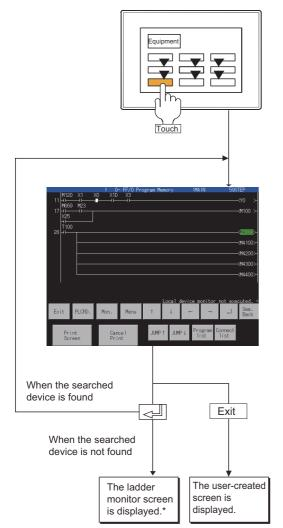
After coil-search, monitoring of the displayed ladder starts automatically.
