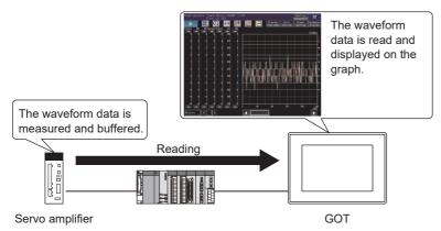
Up to 64 waveform data can be displayed simultaneously.
