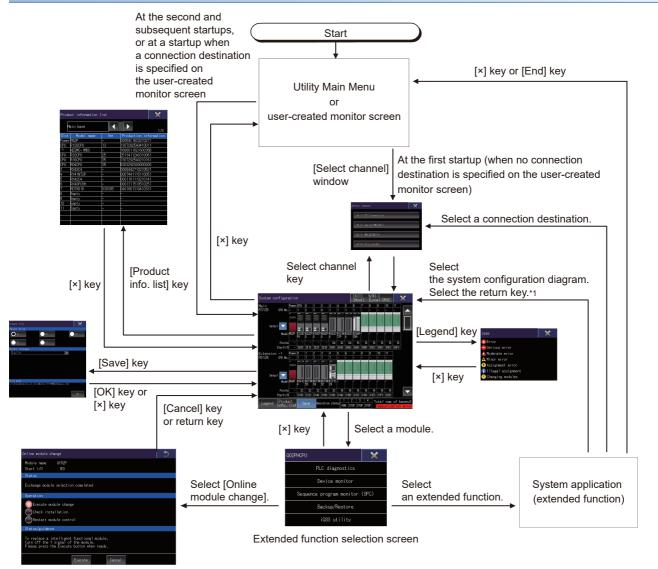
\*1 Only the system launcher (servo network) function is supported.
