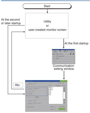
For exiting the CNC data I/O by touching Rtn, the last exited screen is displayed when the CNC data I/O starts next time.
