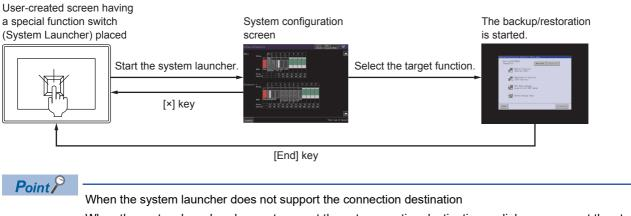
When the system launcher does not support the set connection destination, a dialog appears at the startup.
