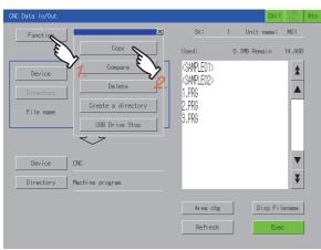
3. Touch the [Area chg] key to switch the frame to the copy source target.
