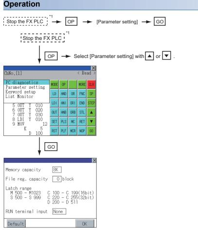
\*1 When checking parameters (not changing), it is not necessary to stop the PLC.
