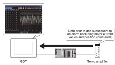
The data read from the connected servo amplifier can be output to a file.
