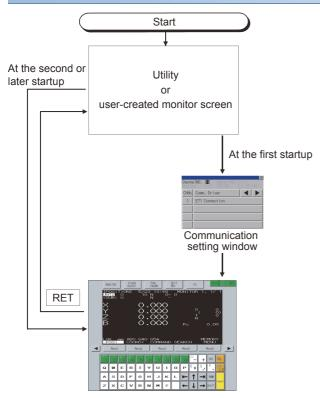
When exiting the CNC monitor function by touching RET, the last exited screen will be displayed when the CNC monitor function is started next time.
