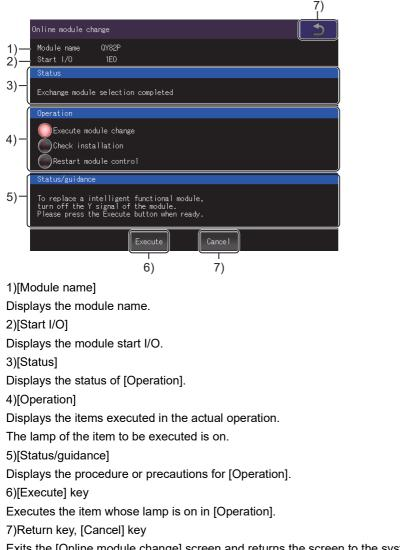
Exits the [Online module change] screen and returns the screen to the system configuration screen.
