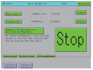
The servo amplifier rotates while the Forward or Reverse key is touched.
