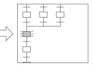
An active step in the block is displayed by automatically scrolling the screen.
