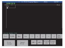
After searching for coil M120 that is in the OFF state, "M669" and "M23" are displayed as devices that are not conductive. Example: M669, M28
