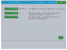
5. Select a function of the servo amplifier monitor.
