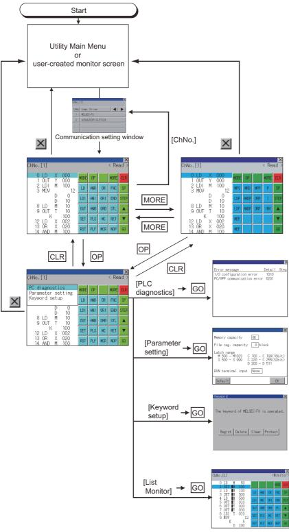
\*1 With setting special function switches (FX list monitor), the list monitor can be started on the monitor screen. When the list monitor is started on the monitor screen, the list editor cannot be used.
