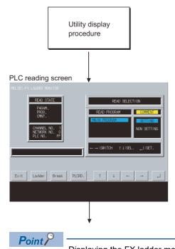
Displaying the FX ladder monitor screen The MELSEC-FX ladder monitor screen displays the sequence program that was executed when the PLC was read. If any of the set values of the sequence program is changed, re-read the PLC.
