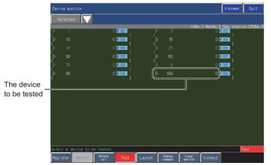
5. A dialog for setting the device value according to the device display format appears.
