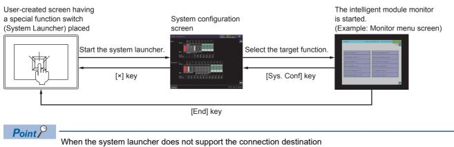
When the system launcher does not support the set connection destination, a dialog appears at the startup. For the details of the system launcher function, refer to the following.
