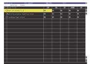
Alternatively, display the block list screen with the special function switch (Sequence program monitor (SFC)) for which [Block List] is selected for [Display Screen] in the switch setting.
