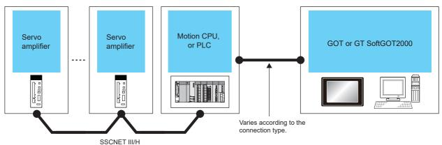
For the connection method between the GOT and the PLC, refer to the following.
