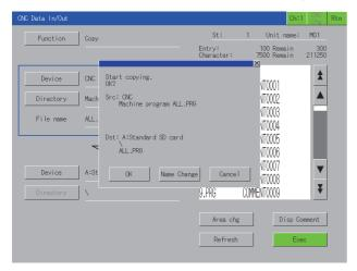
**4.** Touch the [Name Change] key on the copy confirmation window to display the key window. Touch the [AC] key to delete the existing file name from the input value display area.
