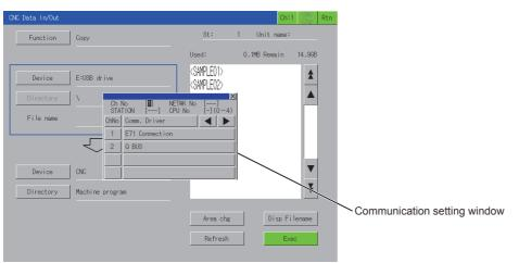
After the GOT is powered on, the communication setting window is displayed only at the first startup of the CNC data I/O. For displaying the communication setting window at the second or later startup, touch the [Ch:] key on the CNC data I/O screen.
