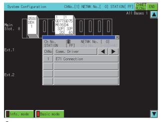
**2.** In the communication setting window, select one from channels No.1 to 4.
