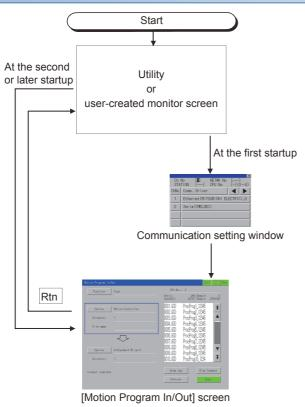
If the motion program I/O is exited with the [Rtn] key, the last displayed screen will appear at the next startup of the motion program I/O.
