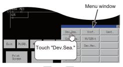
3. Using the 🔳 and 🕨 keys, switch the input area, and enter a device name and its number. \*1
