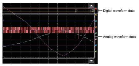
An arrow is displayed on the right edge of a digital waveform.
