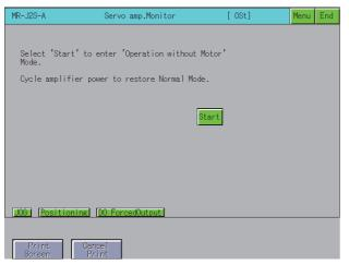
Simulates motion of the servo motor within the servo amplifier even when the servo motor is not connected.
