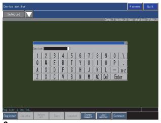
**3.** When a password is not set for a sequence program, touch the [ENTER] key to enter the specified device. When a password is set for the sequence program, the dialog for canceling the password appears when the [ENTER] is touched.
