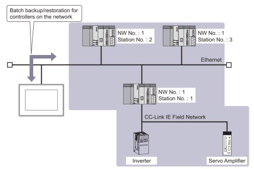
To backup or restore multiple controllers on the network, create a controller list file.
