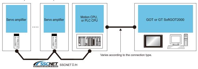
The GOT can be used with MR-J4-□B(-RJ), MR-J4W2-□B, MR-J4W3-□B, MR-JE-□B, MR-J5-□B(-RJ), MR-J5W2-□B, and MR-J5W3-□B in a system configuration.
