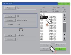
8. Touch the [Device] key to display the device selection window.
