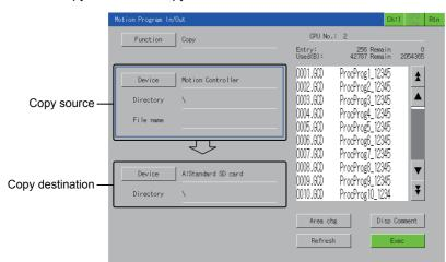
When [Motion Controller] is selected for the copy source, only a data storage can be selected for the copy destination. When the data storage is selected for the copy source, only [Motion Controller] can be selected for the copy destination. The following shows the copy procedure.
