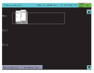
5. Touch the [Parameter Set.] key to display the parameter setting screen.
