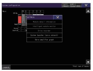
**4.** Touch the system launcher (servo network) from the function list to display the servo network configuration diagram. Page 826 Operating Procedure
