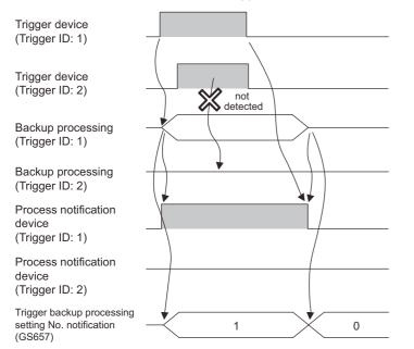
For ensuring the trigger backup, establish a handshake with the trigger device and the process notification device.
