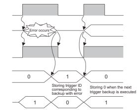
Trigger backup processing setting No. notification (GS657)
