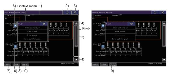
When a Motion module is selected (Amplifier display)
