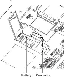
**5.** After installing the battery to the battery holder of the GOT, close the battery cover until it clicks.
