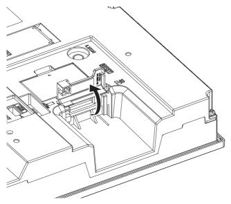
2. Open the SD card cover completely, and check that the SD card access LED is off. Then, hold an SD card with its front side facing up, and insert the card into the SD card interface.
