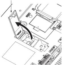
**3.** To replace the battery, remove the old battery, and then disconnect the connector.
