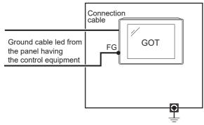
The malfunction due to the potential difference caused by the grounding in such a case may be prevented by reducing the voltage as shown in countermeasure example 1 below.
