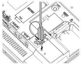
3. Pass the USB cable through a hole of the cable clamp and pull the band to fix the cable.
