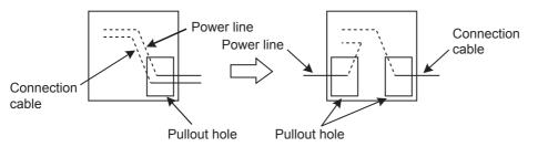
Keep the power line and communication cable inside the duct at least 100 mm away from each other. If that is not possible, the use of a metal separator inside the duct can reduce noise interference.
