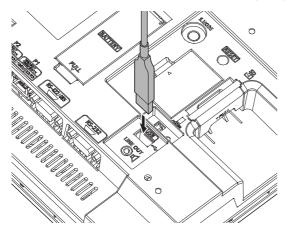
**2.** Insert a cable clamp to the mounting hole for a cable clamp shown in the following figure and push it until you hear a clicking sound.
