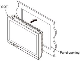
**2.** Align the fittings (four fittings) on the installation holes on the GOT, and tighten the screws within the specified torque range (0.36 N·m to 0.48 N·m).
