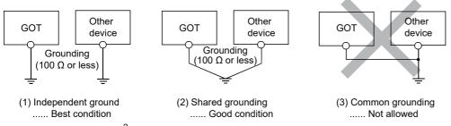
• Use the cable of 2 mm<sup>2</sup> or longer for grounding. Set the ground point as close to the GOT as possible to shorten the grounding cable.
