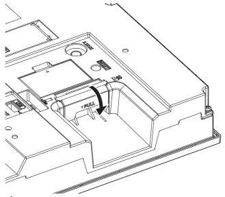
4. When the SD card cover is closed, the access to the SD card is allowed.
