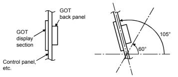
The GOT will have a longer lifetime if used within the mounting angles shown above. Ideally, the temperature inside the control panel should not exceed 0 to 40°C.
