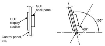
The GOT will have a longer lifetime if used within the mounting angles shown above. Ideally, the temperature inside the control panel should not exceed 0 to 40°C.
