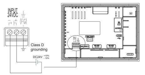
Tightening torque for the power terminals: 0.5 to 0.6 N·m
