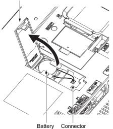
**3.** After removing the battery from the battery holder of the GOT, unplug the connector.
