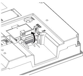
2. Open the SD card cover completely, and check that the SD card access LED is off. Then, push the SD card in to eject it.
