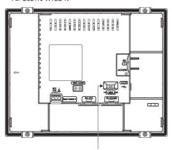
Terminating resistor selector switch
