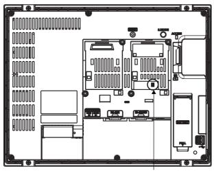
Terminating resistor setting switch (inside the cover)
