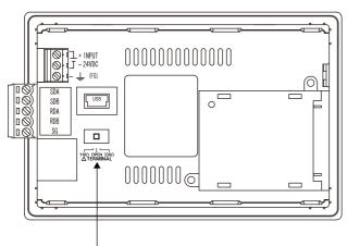
Terminating resistor selector switch
