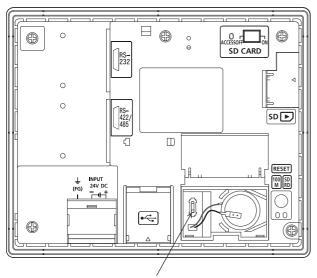
Terminating resistor selector switch
