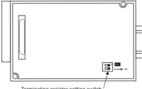
Terminating resistor setting switch
