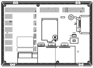
Terminating resistor setting switch (inside the cover)
