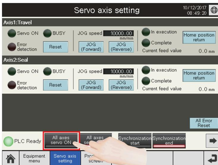
2. Touch the [All axes servo ON] switch. All axes are in the servo-on status.
