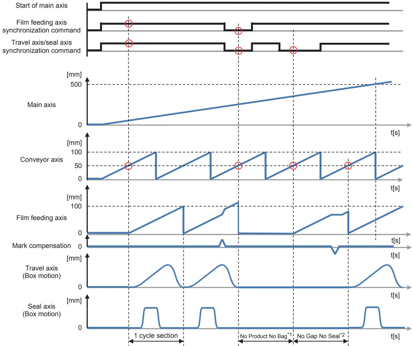
\*1 When workpieces are not conveyed or spaces between workpieces are too wide, this function stops the travel axis, seal axis, and film feeding axis to prevent packaging mistakes.
