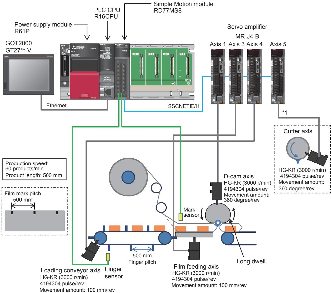
\*1 The end seal part has been configured with the long dwell. This application package also includes programs to generate cam patterns for using the rotary cutter.
