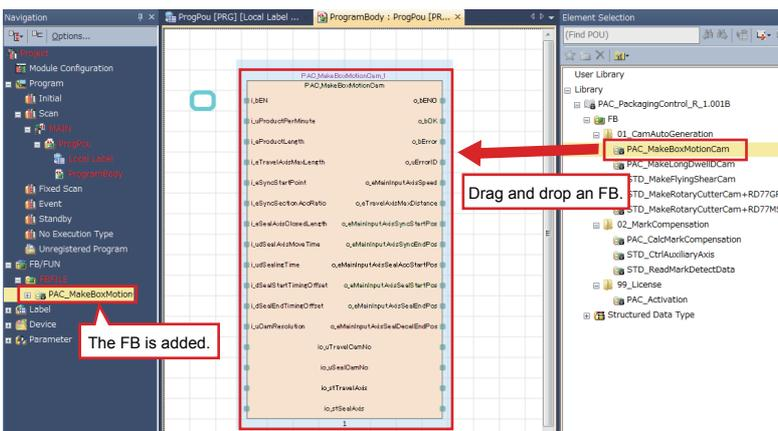
9. Select the FB to be used from the Element Selection window, and drag and drop it into the work window. The FB is added in the Navigation window.
