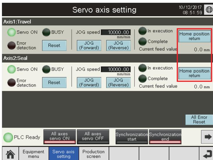
3. When this is the first startup of the system, touch the [Home position return] switch of each axis and perform home position return operations.
