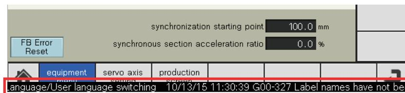
When a GOT system alarm occurs, a system alarm is displayed overlapping the bottom of the screen that is being displayed.
