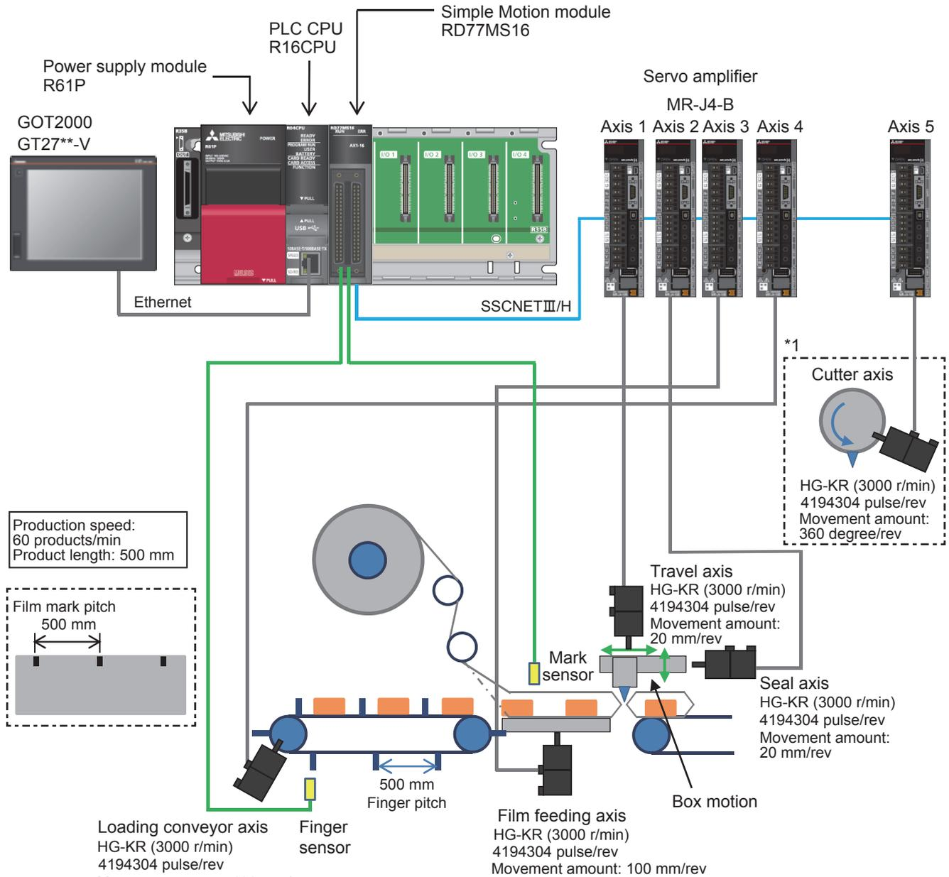
\*1 The end seal part has been configured with the box motion. This application package also includes programs to generate cam patterns for using the rotary cutter.
