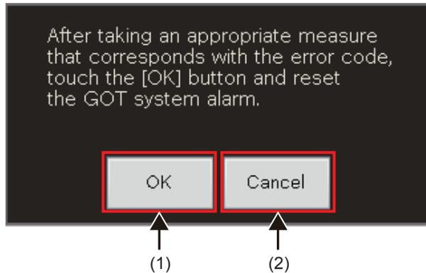
When a GOT system alarm has occurred, touching the system alarm message display area (bottom of the screen) displays this screen.
