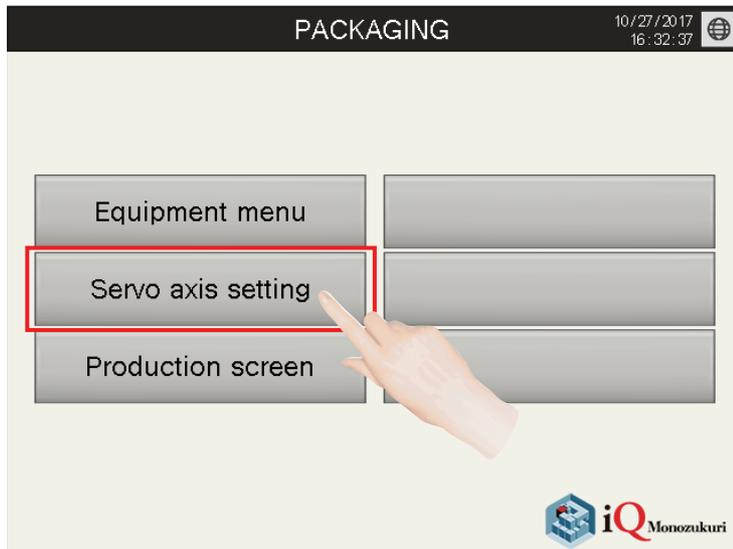
1. Write project data to the PLC CPU and GOT and start the system. Touch [Servo axis setting] to display the servo axis setting screen.
