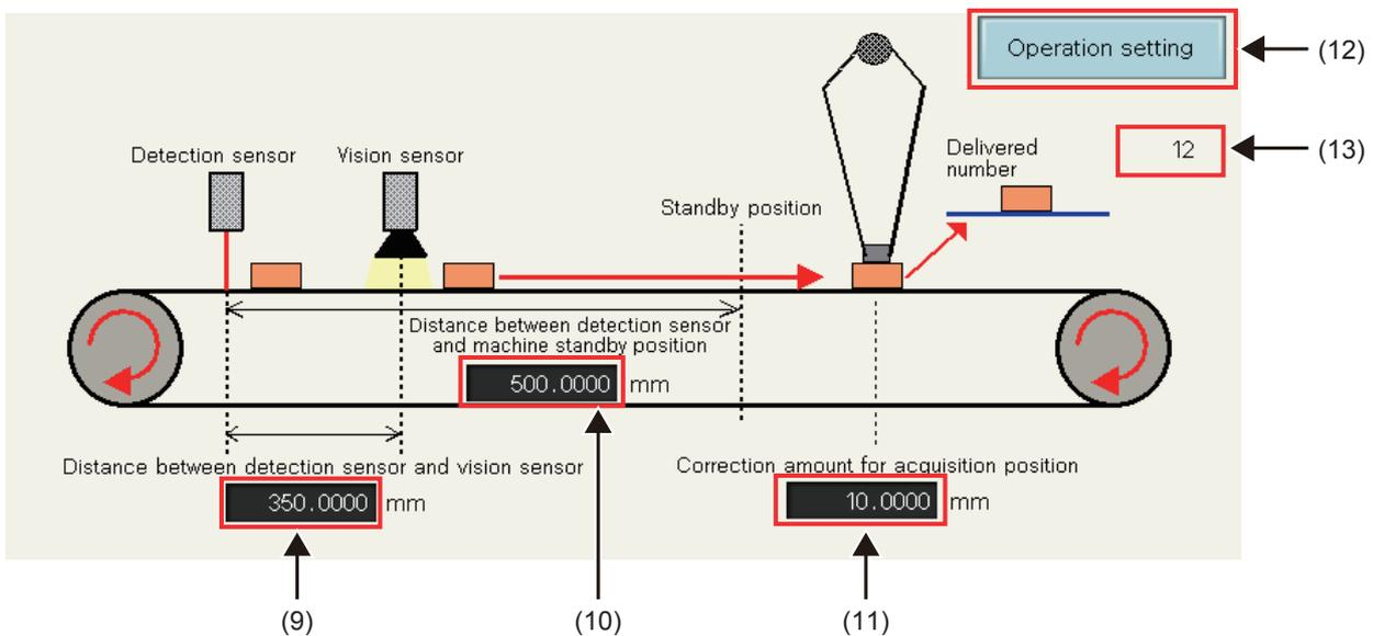
(9) Distance between detection sensor and vision sensor
