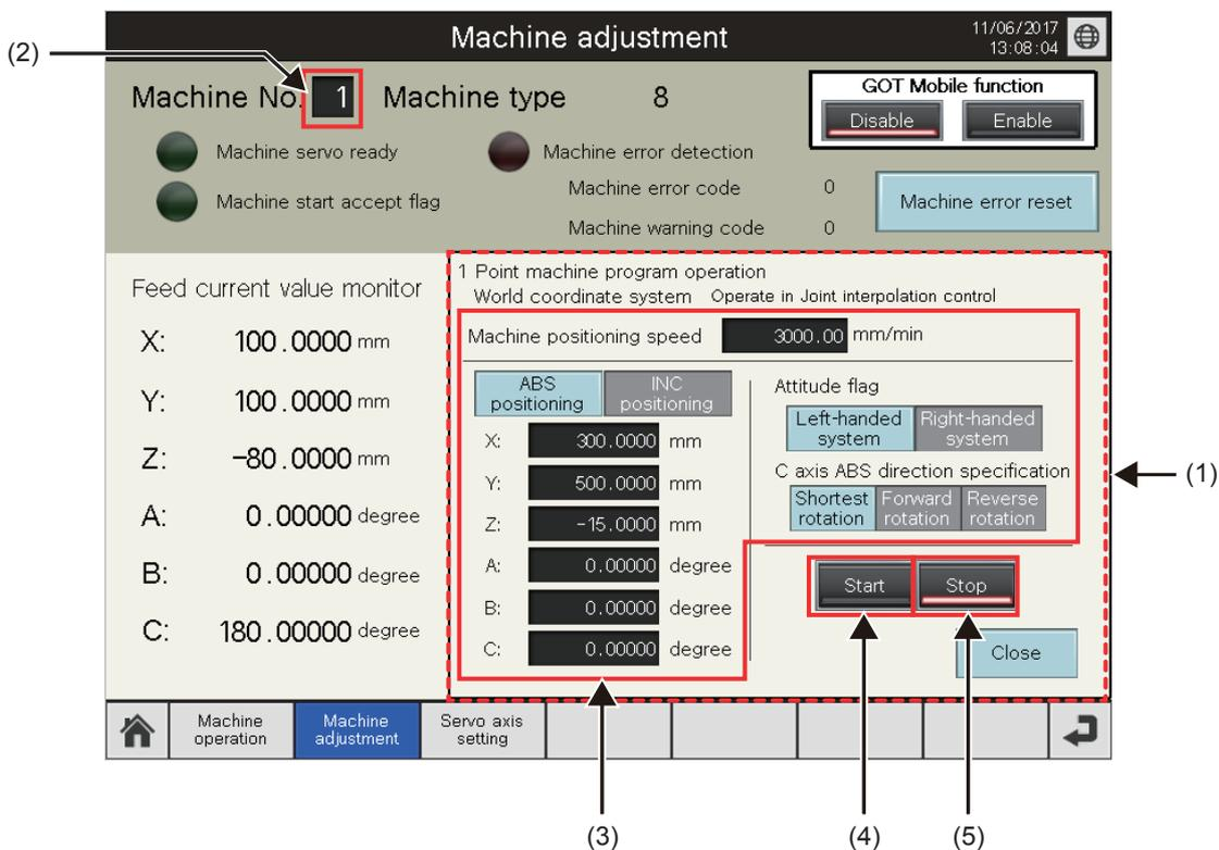
(1) Settings and operations of the 1 Point machine program operation are performed on the 1 Point machine program operation window screen.
