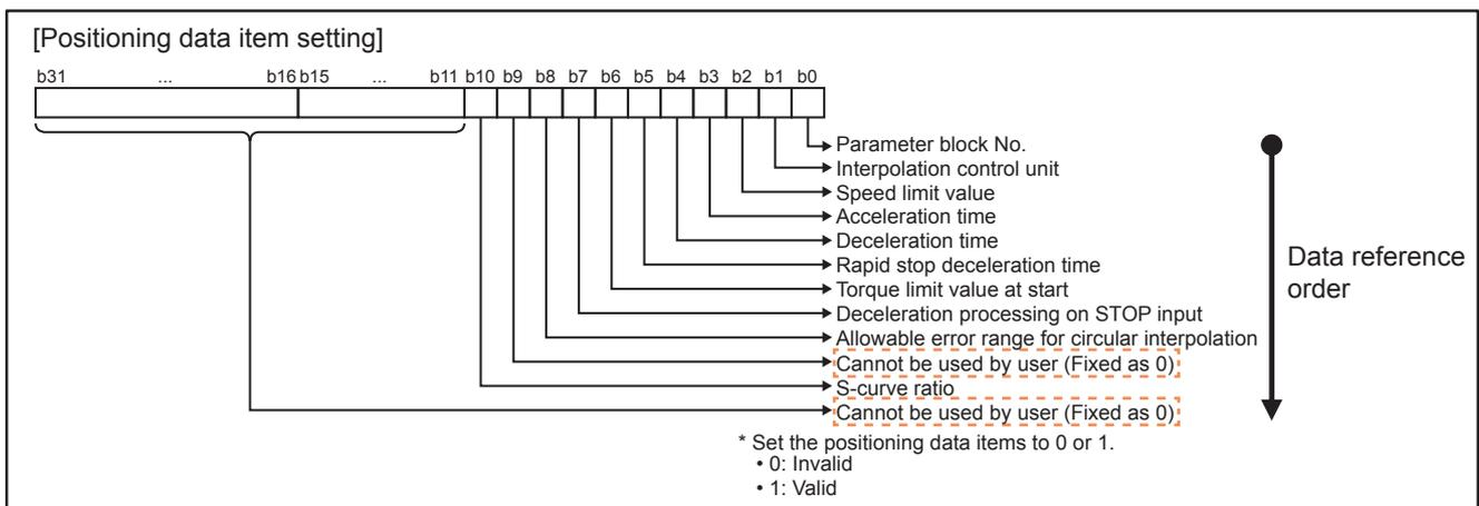
If the setting is not invalid (-1), turn ON the corresponding bit of the positioning data item setting, and save it as a positioning data item. Thereafter, perform two-word offset for the reference-source device and storage-destination device.
