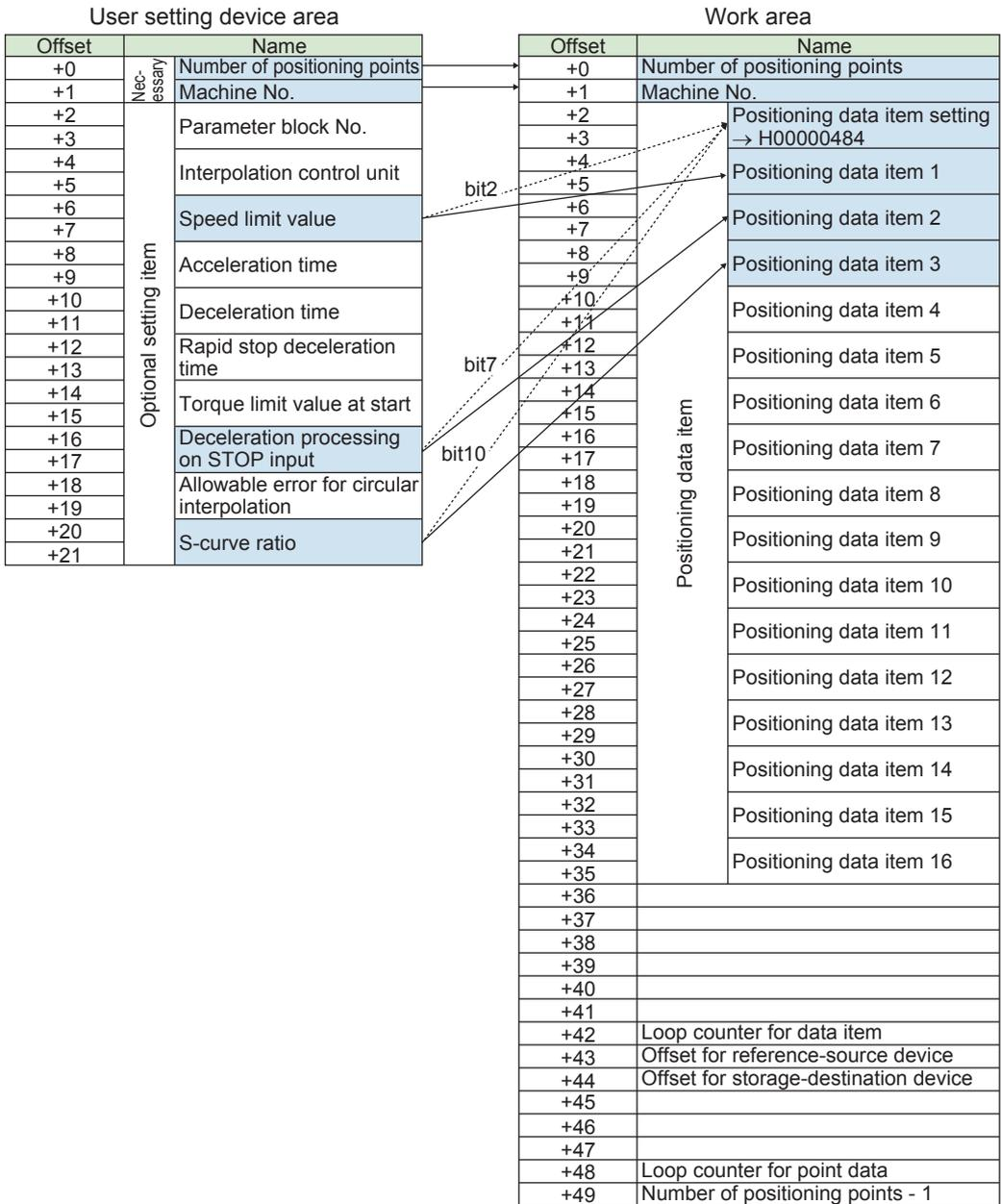
4. Transfer the data (36 words) of the prepared header part in a batch as shown below.
