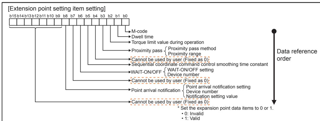
If the setting is not invalid (-1), turn ON the corresponding bit of the positioning data item setting, and save it as a positioning data item. Thereafter, perform two-word offset for the reference-source device and storage-destination device.
