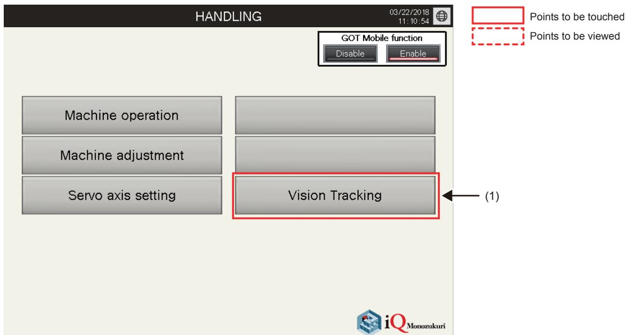
(1) Write the project data to the PLC CPU, Motion CPU, and GOT. After starting up the system, touch the [Vision Tracking] switch to open the Vision Tracking screen.
