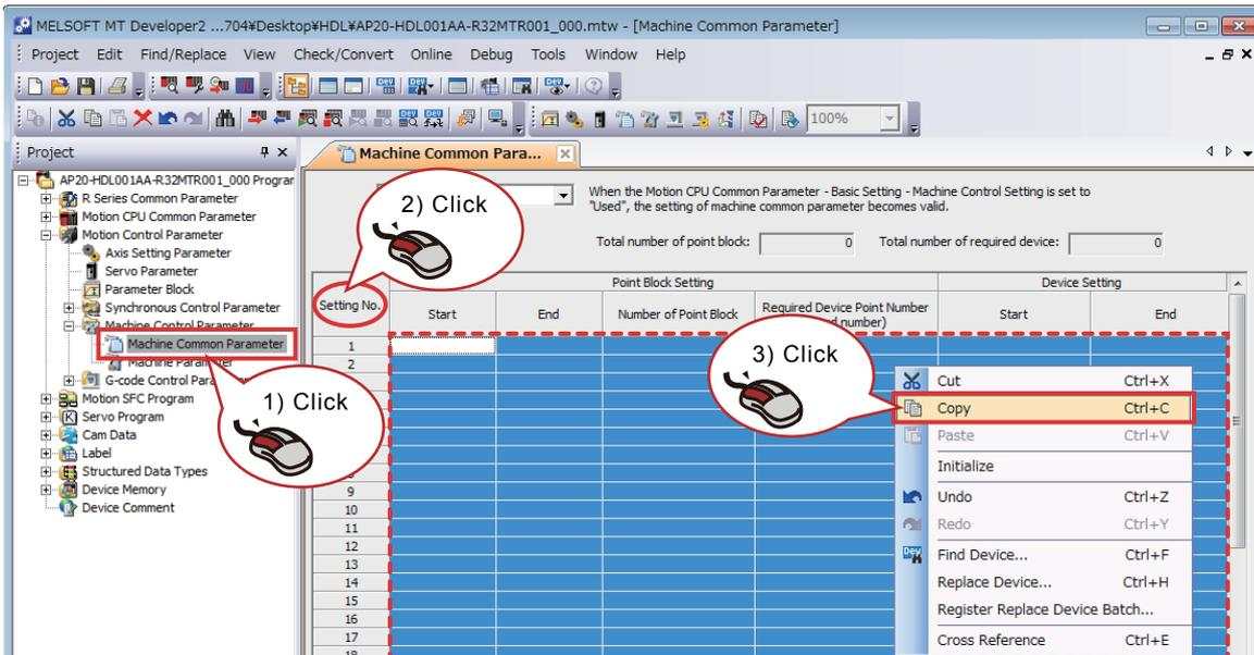
Open the tool, and paste the machine common parameters on the same setting screen in the [PARAM] sheet.
