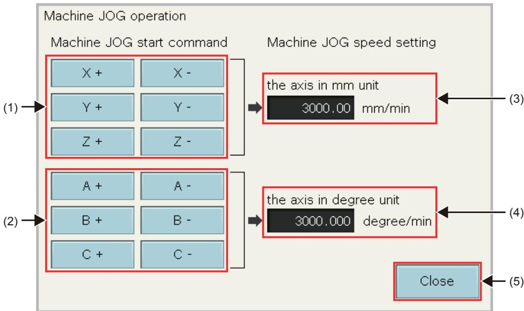
(1) Machine JOG start command (coordinates X, Y, and Z)
