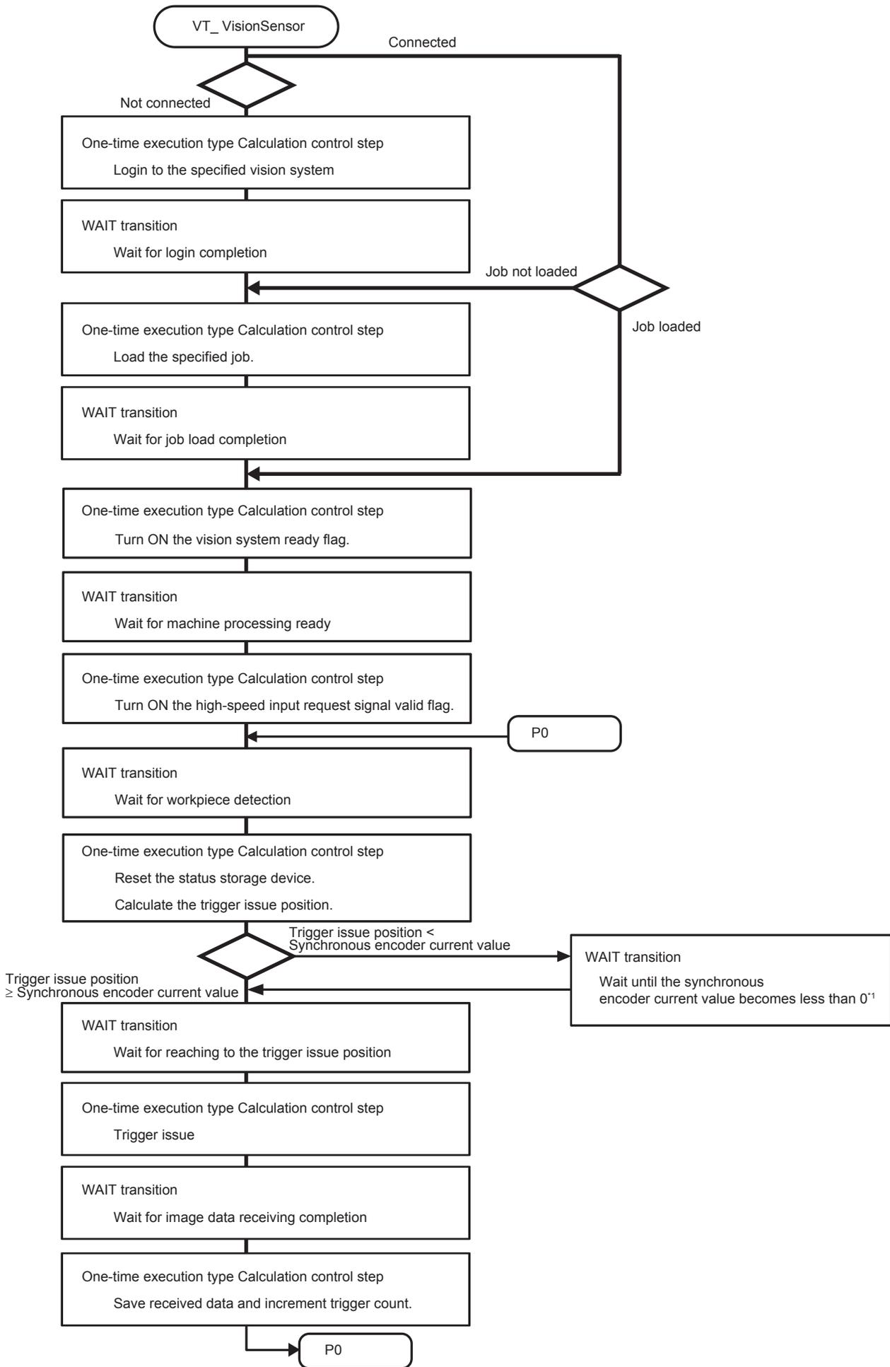
\*1 The "trigger issue position" is the sum of "synchronous encoder current value (at mark detection)" and "distance between detection sensor and vision sensor". As a result, "trigger issue position" is more than "synchronous encoder current value". At the transition of waiting for trigger issue position, the vision trigger is issued when "synchronous encoder current value" is more than "trigger issue position".
