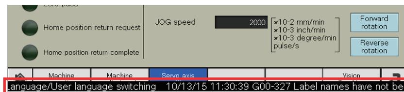
When a GOT system alarm occurs, a system alarm is displayed overlapping the bottom of the screen that is being displayed. For details on the GOT system alarms, refer to "Page 89 GOT system alarm".
