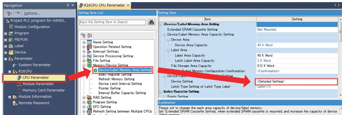
2. Set D100 in the latch (1) setting window of data register D.
