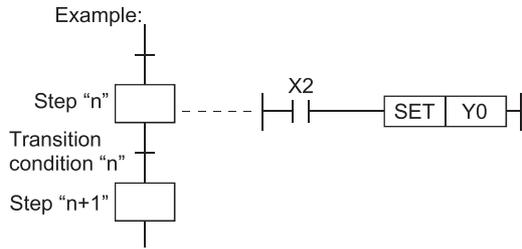
When transition condition "n" becomes satisfied at the step "n" operation output where Y0 is ON (by SET instruction), the Y0 ON status will be maintained even after the transition to step "n + 1".
