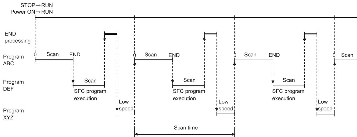
\*1 For the Universal model QCPU and LCPU, only one SFC program (one normal SFC program) can be scanned.
