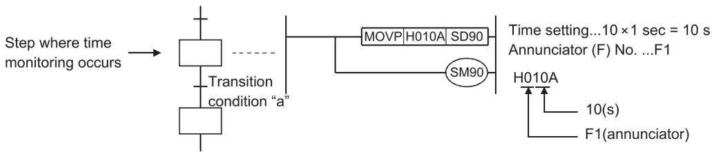
When SM90 is turned ON in the operation output of the step that performs a time check as shown below, the step transition watchdog timer starts timing.
