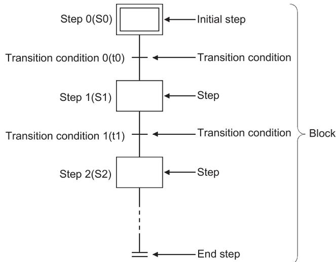
An SFC program starts at an initial step, executes a step following a transition condition in due order every time that transition condition is satisfied, and ends a series of operations at an end step.
