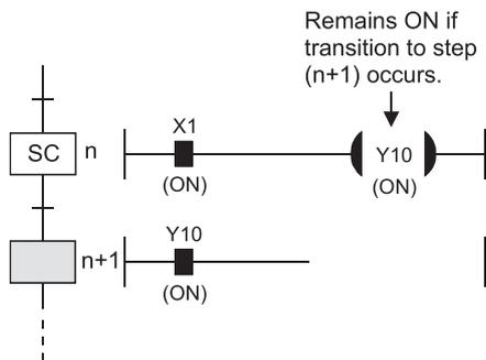
At a designated coil HOLD step, "Y10" (switched ON by OUT instruction) will remain ON even when the transition condition is satisfied.
