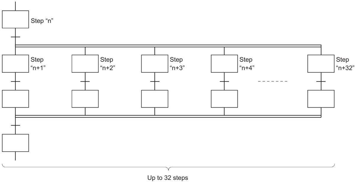
If another block is started by the parallel processing operation, the START source block and START destination block will be executed simultaneously. (In the example below, processing from step "n+1" will be executed simultaneously with block 1.)
