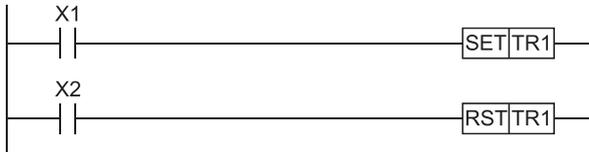
When step is designated by operation output of other than block 1 or sequence program
