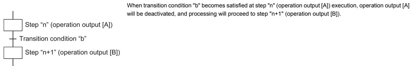
A maximum of 512 serial transition steps can be described in each block.\*1 Therefore, a maximum of 512 serial transitions (+) can be described. However, there is a restriction on the number of lines as indicated below depending on the SFC display column setting.
