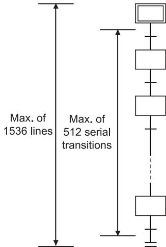
\*Examples of the permissible number of lines corresponding to a few SFC display column setting values are shown below. The SFC display column setting value can be designated freely within a 1 to 32 range.
