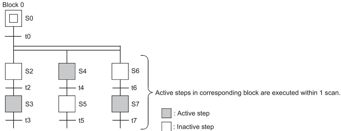
At the end of the operation output execution at each step, whether the transition condition to the next step is satisfied or not is checked.
