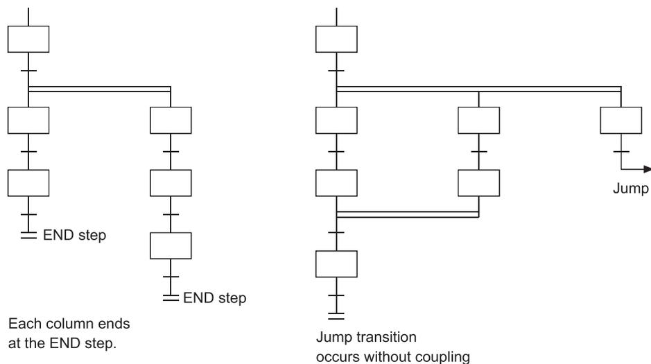
As a rule, a waiting step must be created prior to the coupling. However, in cases such as the example below where each of the parallel transition columns consist of only 1 step (program without a transition condition between the parallel transition branch and the coupling), a waiting step is not required.
