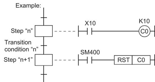
When the counter (C0) is reset at step "n+1" (or subsequent step), the present value will be cleared, and the contact will be switched OFF.
