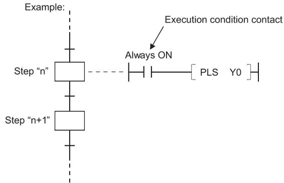
The ladder shown above is actually executed as shown below. Because the step conditions contact is ON when the step is active and OFF when the step is inactive, the PLS or □P instruction will be executed when the step becomes active, even though the execution condition contact is always ON.
