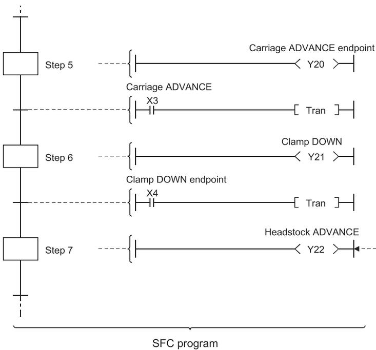
As shown in the SFC program at left, the steps require no "operation completed" interlock contact with the previous step. With a conventional sequence program, carriage FORWARD (Y20) and clamp DOWN (Y21) interlock contacts would be required at the ladder used for the headstock ADVANCE.
