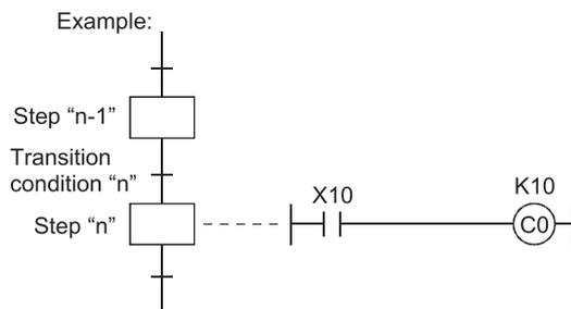
If X10 at step n is already ON while step (n-1) is active, counter C0 counts once when execution proceeds to step n after transition condition n is satisfied.
