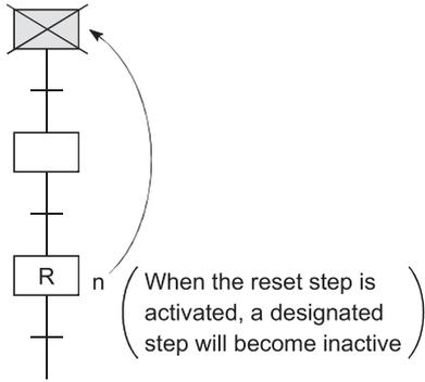
When a HOLD status becomes unnecessary for machine control, or on selective branching to a manual ladder occurs after an error detection, etc., a reset request can be designated for the HOLD step, deactivating the step in question.
