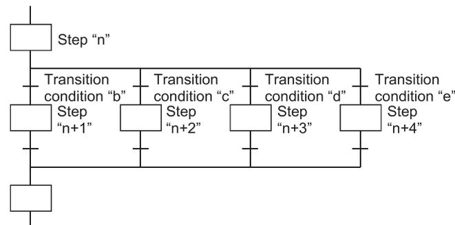
In a selection transition, a coupling can be omitted by a jump transition or end transition.
