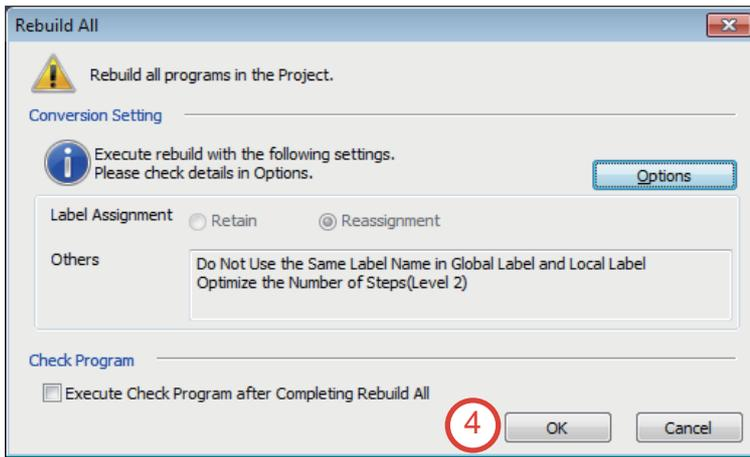
4. Check that "Label Assignment" is set to "Reassignment", and click the [OK] button.
