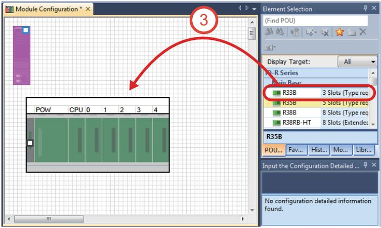
3. Select the main base unit "R35B" in the "Element Selection" window, and drag and drop it to the "Module Configuration" window.
