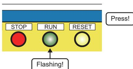
1. Press the emergency stop switch of the demonstration machine (safety component side).
