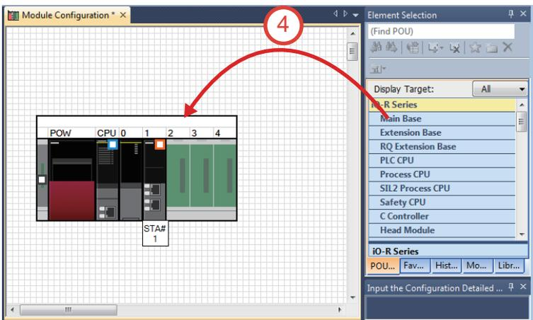
4. Select modules in the "Element Selection" window, and drag and drop them to the "Module Configuration" window in the same way as Step 3.
