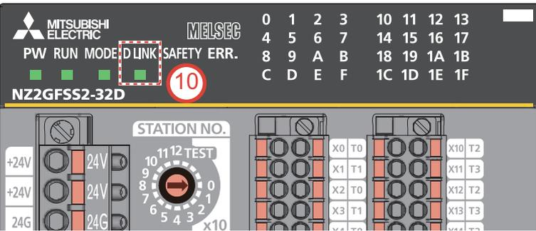
10. Check that the D LINK LED of the safety remote I/O module is on.
