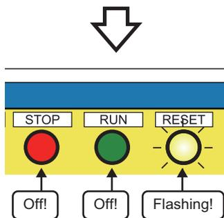
3. When the demonstration machine recovers, the indicator lamp of the operation preparation switch (RESET) flashes.
