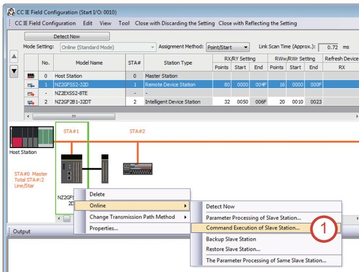
1. On the "CC IE Field Configuration" window, right-click on "NZ2GFSS2-32D", and select [Online] → [Command Execution of Slave Station].
