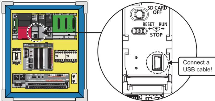
1. Connect the personal computer to the safety programmable controller with a USB cable.
