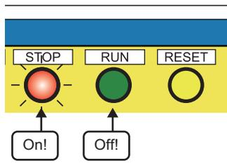
2. The indicator lamp of the start switch (RUN) turns off, and the stop indicator lamp (STOP) turns on.
