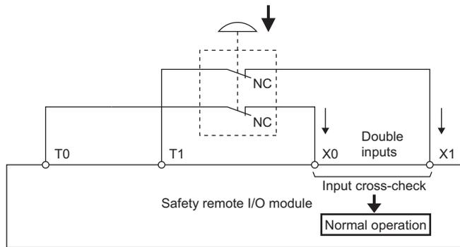
(Disconnection simulation switch: On (disconnection))
