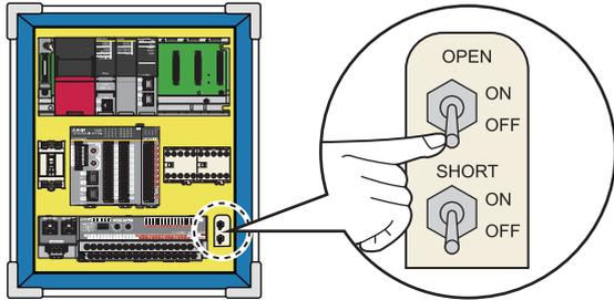
1. Turn off the OPEN (disconnection simulation) switch and the SHORT (short-circuit simulation) switch.
