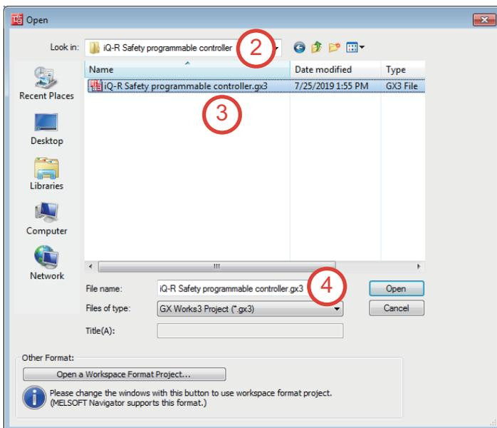
2. The "Open" window appears. Specify the location where the sequence program "iQ-R Safety programmable controller" is stored.
