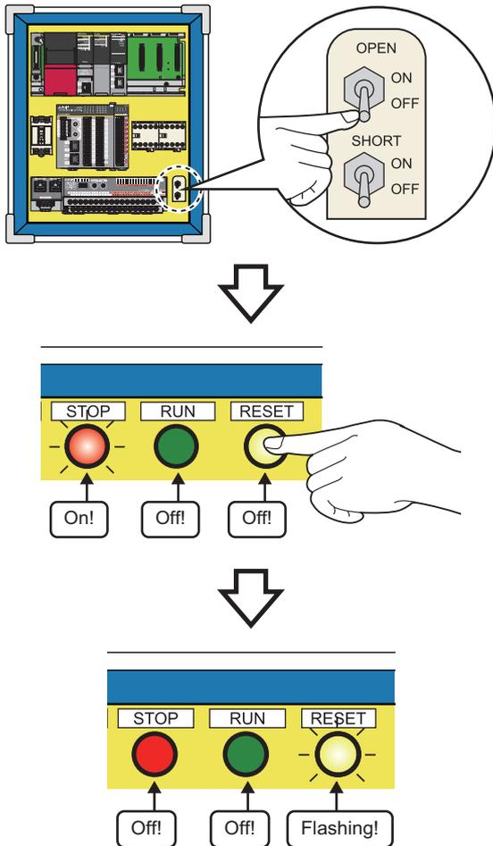
**1.** Turn off the OPEN (disconnection simulation) switch and the SHORT (short-circuit simulation) switch.
