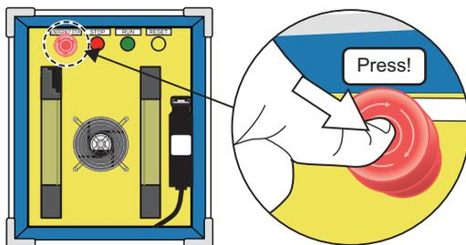
3. Press the emergency stop switch of the demonstration machine (safety component side).
