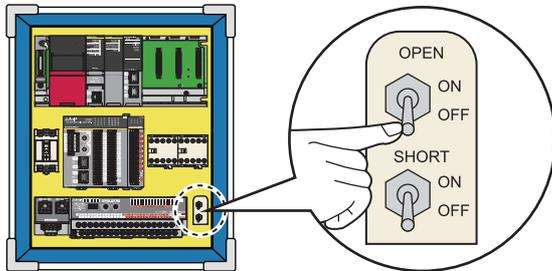
1. Turn off the OPEN (disconnection simulation) switch.
