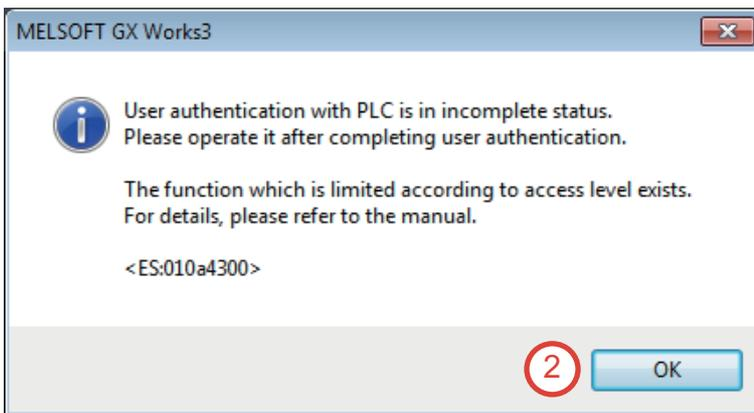
2. If the user authentication with the programmable controller is not completed, the "Use Authentication" window appears. Click the [OK] button.
