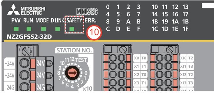
**10.** Check that the SAFETY LED of the safety remote I/O module is on.
