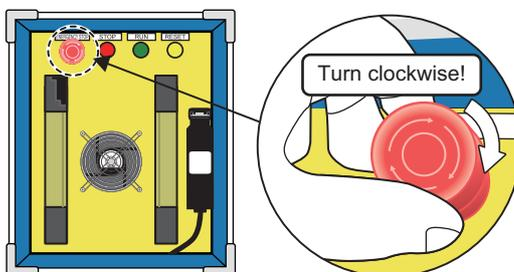
4. Return the emergency stop switch to its original position.
