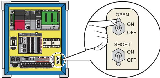
1. Turn on the OPEN (disconnection simulation) switch of the demonstration machine (safety programmable controller side).
