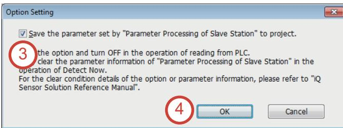
3. Check that the "Save the parameter set by "Parameter Processing of Slave Station" to project." checkbox is selected.
