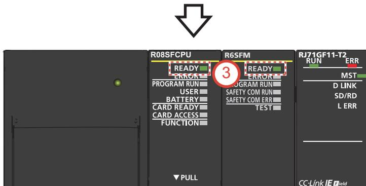
3. Check that the READY LED of the Safety CPU (R08SFCPU) and the safety function module (R6SFM) is on.
