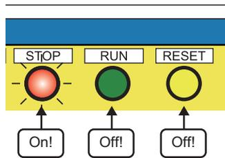
2. The fan stops. The indicator lamp of the start switch (RUN) turns off, and the stop indicator lamp (STOP) turns on.
