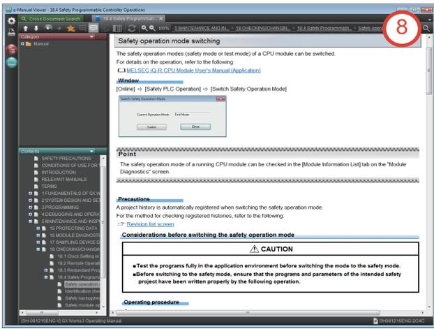
8. Every time the project is written to the safety programmable controller, e-Manual Viewer starts up and precautions for the safety operation mode switching are displayed. Click the [X] button.
