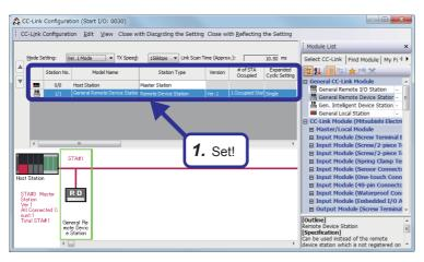
In the "CC-Link Configuration" dialog box, drag and drop the following modules from "Module List" to the list of stations or the network map.
