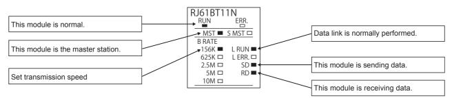
(2) LED display of the remote I/O station Check that the LED display is as follows.
