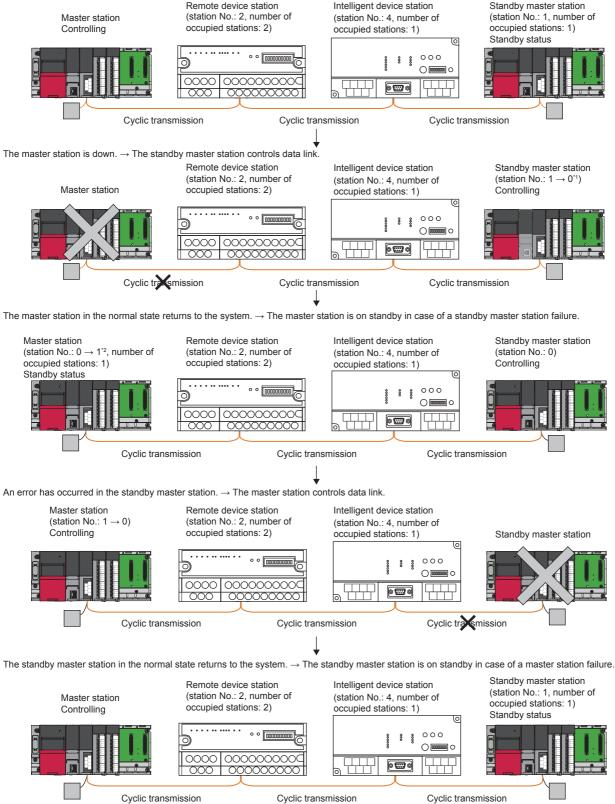
\*1 The dot matrix LED displays the station number set in the module instead of "0". The MST LED turns on and the S MST LED turns off. \*2 When the master station returns to the system, it operates with the station number of the standby master station, but the dot matrix LED displays the station number set in the module ("0" for the master station). The MST LED turns off and the S MST LED turns on.
