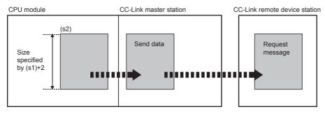
When the number of bytes in the send data ((s1)+2) is odd, the lower byte is sent as for the last data.
