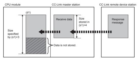
If the receivable data size ((s1)+3) is smaller than the receive data size ((s1)+4), the master station cannot receive data from the remote device station. The G(P).RDMSG instruction completes with an error (error code: B418H).
