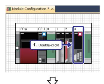
**1.** Double-click the RJ61BT11 module in the module configuration.
