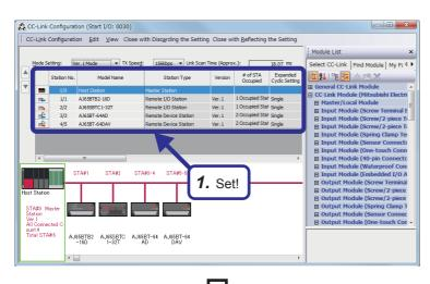
In the "CC-Link Configuration" dialog box, drag and drop the following modules from "Module List" to the list of stations or the network map.
