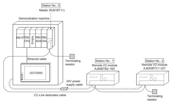
\*1 The settings of modules used in the master station and remote I/O stations and the connection methods of CC-Link dedicated cables and 24V power supply cables are the same as those for Exercise 1.
