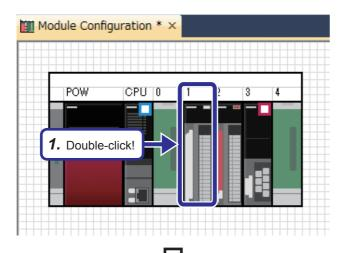
**1.** Double-click the R60AD4 module in the module configuration.
