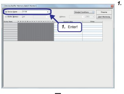
Enter "D1108" in "Device Name" and press the <u>Inter</u> key on the "Device/Buffer Memory Batch Monitor" dialog box.
