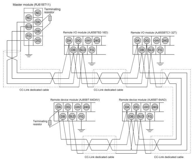
After connecting CC-Link dedicated cables and 24V power supply cables, check if the connection status is normal through a line test. ( Page 3 - 28 Writing parameters)
