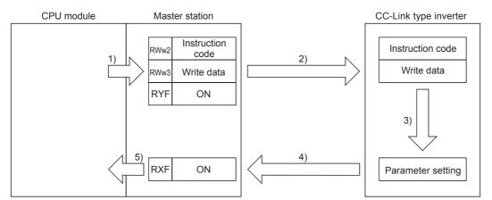
1) Set an instruction code and write data in the remote register with sequence programs and turn on the instruction code execution request signal (RYF).
