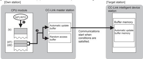
O Data is read from the device specified by (s) and later of the master station.
