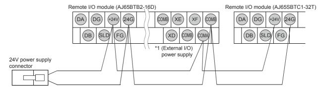
\*1 The external I/O power supply of the AJ65BTB2-16D has both polarities. (Both the combination of COMA+ and COMB- and the combination of COMA- and COMB+ are available.)
