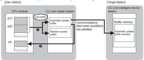
Data is read from the automatic update buffer or random access buffer specified by (s1) and (s2) that is in the master station.
