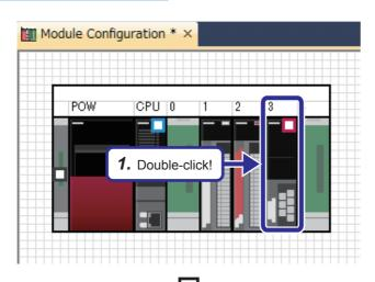
**1.** Double-click the RJ61BT11 module in the module configuration.
