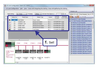
In the "CC-Link Configuration" dialog box, select "RJ61BT11" from "Master/Local Module" in "Module List" and drag and drop it to the list of stations or the network map.
