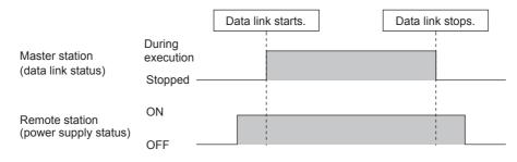
(2) Upon a momentary power failure of a remote station
