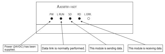
(3) LED display of the remote device station Check that the LED display is as follows.
