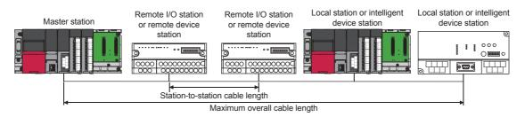
Ver.1.10-compatible CC-Link dedicated cable (a terminating resistor of 110Ω used)
