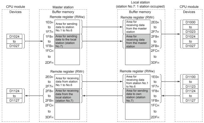
Between the master station and the local station, each data is stored diagonally.
