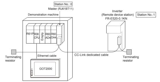
The CC-Link type inverter is handled as a remote device station.
