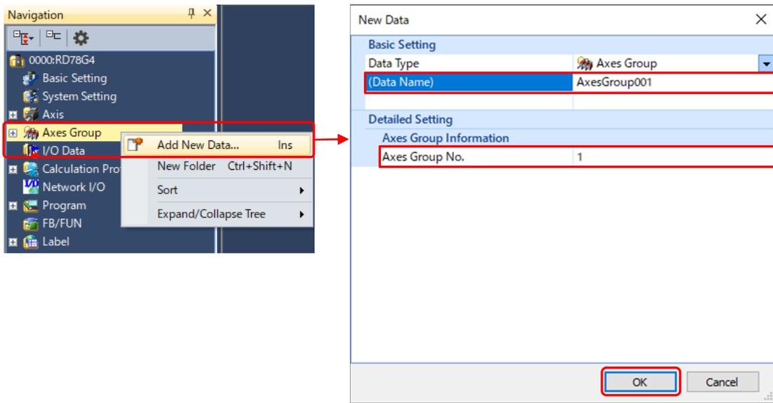
The X axis (Axis0001) and Y axis (Axis0002) of the following two-axis machine example (refer to Section 2.1) are registered in an axes group.
