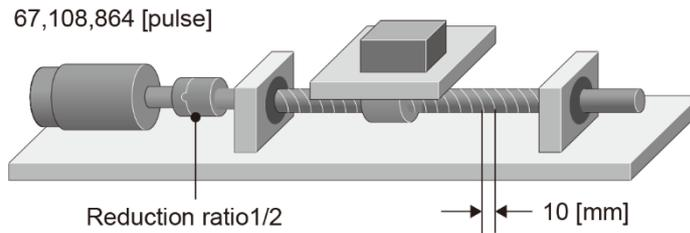
Servo motor encoder resolution: 67,108,864 [pulse] (26 bits)
