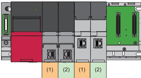
(1) Programmable controller CPU No.1 (trigger relay device)/recorder module (recording device) controlled by CPU No.1
