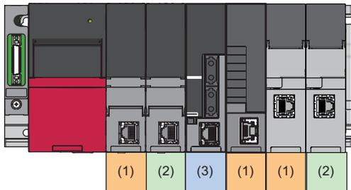
(1) Programmable controller CPU No.1/recording device controlled by CPU No.1
