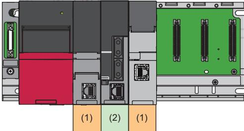
(1) Programmable controller CPU No.1 (trigger relay device)/camera recorder module (recording device) controlled by CPU No.1
