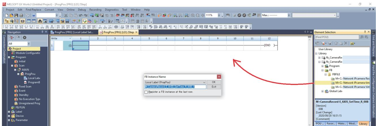
2. Enter the input labels and output labels of the created FB to create a program.
