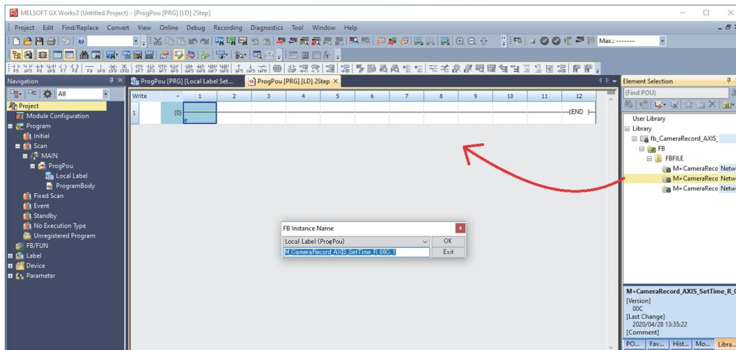
2. Enter the input labels and output labels of the created FB to create a program.
