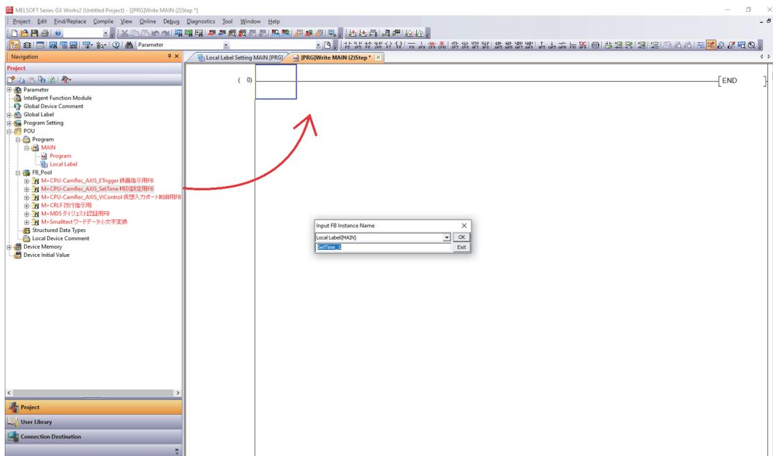
2. Enter the input labels and output labels of the created FB to create a program.
