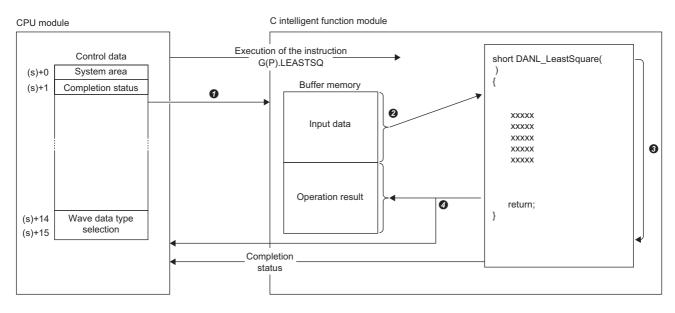
• A value specified in the control data is passed to a C intelligent function module.
