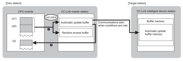
• Data is read from the automatic update or random access buffer specified by (s1) and (s2) that is in the master station.
