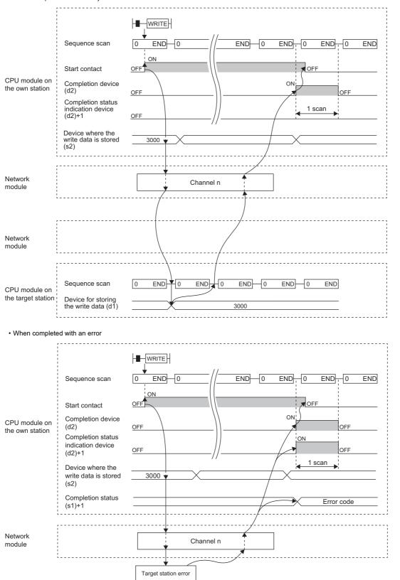
· Write processing is performed only once on the rising edge when the write command turns on.
