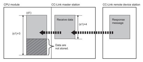
If the receivable data size ((s1)+3) is smaller than the receive data size ((s1)+4), the master station cannot receive data from the remote device station. The G(P).RDMSG instruction completes with an error (error code: B418H).
