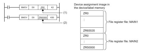
(1) The transfer destination is in the range of file register MAIN1. Data is written to ZR0 and ZR1.
