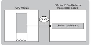
• The execution status and the completion status of the G(P).CCPASET instruction can be checked with the completion device (d) and the completion status indication device (d)+1.
