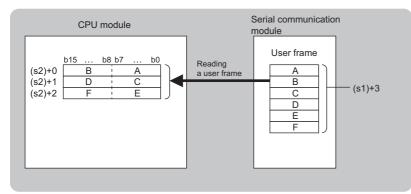
• The completion status of the G(P).GETE instruction can be checked with the completion device (d) and the completion status indication device (d)+1.
