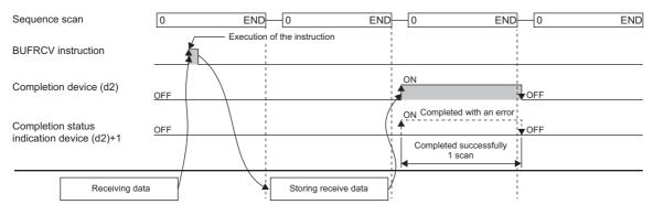
The BUFRCV instruction is executed on the rising edge (off to on) of the socket/fixed buffer receive status signal (Un\G1900016 to Un\G1900023).
