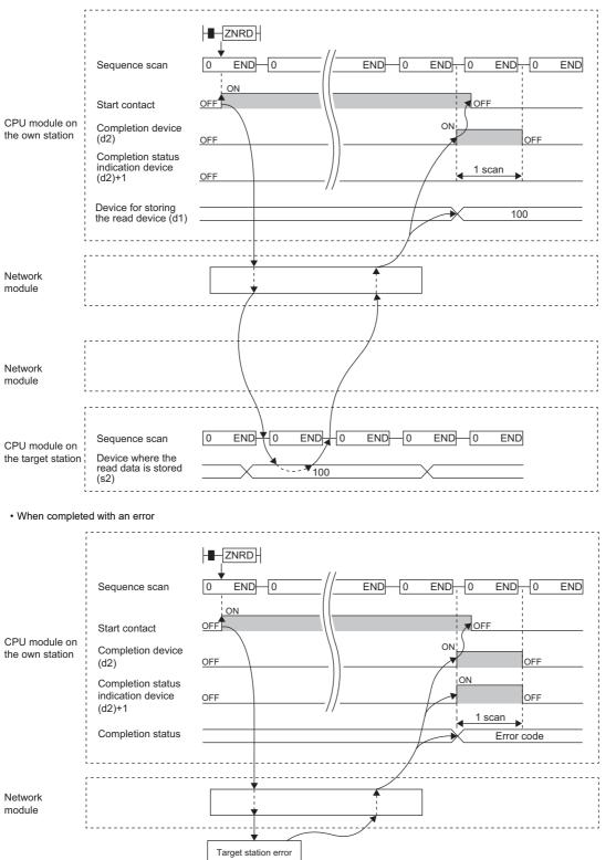
The completion status is stored in the special register (SW) when the CC-Link IE Controller Network is used, in the buffer memory when Ethernet is used, or in the special register (SW0031) when the MELSECNET/H is used.
