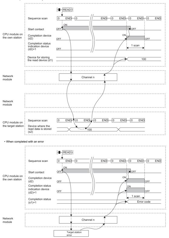
· Read processing is performed only once on the rising edge when the read command turns on.
