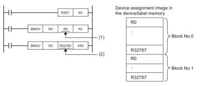
(1) The transfer destination is in the range of the R device of block number 0. Data is written to R0 and R1.
