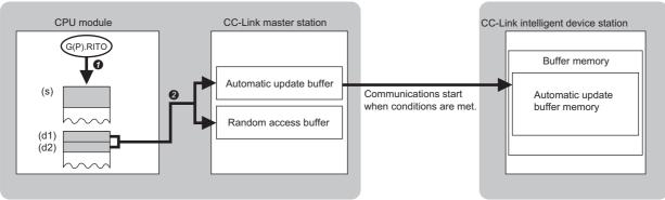
O Data is read from the device specified by (s) and later of the master station.
