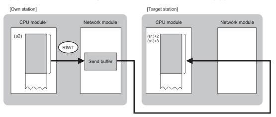
• The execution status and the completion status of the RIWT instruction can be checked with the completion device (d) and the completion status indication device (d)+1.
