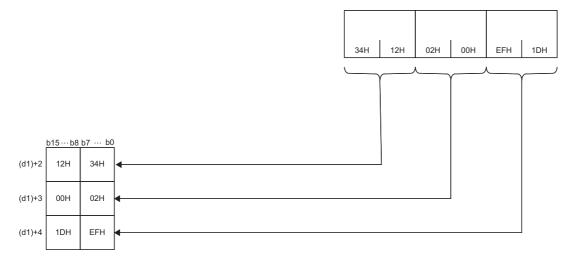
• The following example shows that request data is stored in (s2)+2 and later (station number extension frame).
