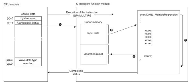
• A value specified in the control data is passed to a C intelligent function module.
