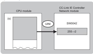
• The execution status and the completion status of the UINI instruction can be checked with the completion device (d) and the completion status indication device (d)+1.
