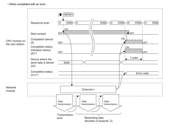
• Send processing is performed only once on the rising edge when the send command turns on.
