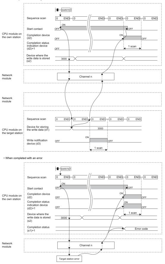
• Write processing is performed only once on the rising edge when the write command turns on.
