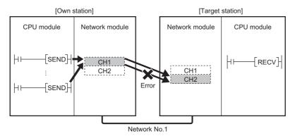
• When multiple network modules are mounted in the target station, specify the network number and station number of the network module that receives a request from the own station.
