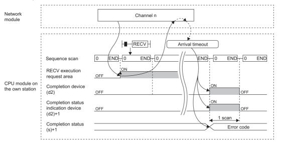
Read processing is performed only once on the rising edge when the read command turns on.
