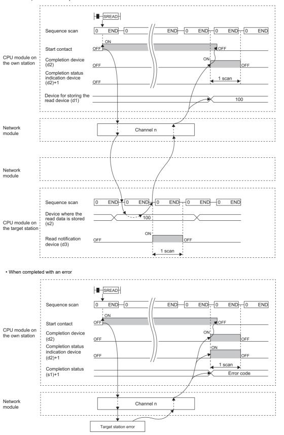
· Read processing is performed only once on the rising edge when the read command turns on.
