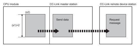
When the number of bytes in the send data ((s1)+2) is odd, the lower byte is send as for the last data.
