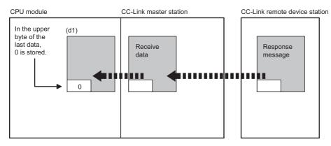
• When the number of bytes in the receive data ((s1)+4) is odd
