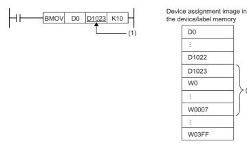
(1): The transfer destination is in the range corresponding to D1023 to D1032. Even though the range D1024 to D1032 does not exist, the data are written and the data in W0 to W0007 are overwritten.
