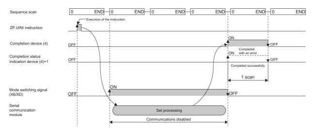
• Stop the whole data communication with the external device before issuing the ZP.UINI instruction. If the ZP.UINI instruction is issued while data communication is in progress with the external device, the following will occur.
