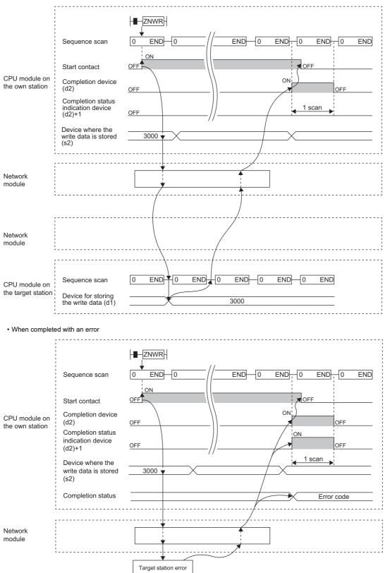
The completion status is stored in the special register (SW) when the CC-Link IE Controller Network is used, in the buffer memory when Ethernet is used, or in the special register (SW0033) when the MELSECNET/H is used.
