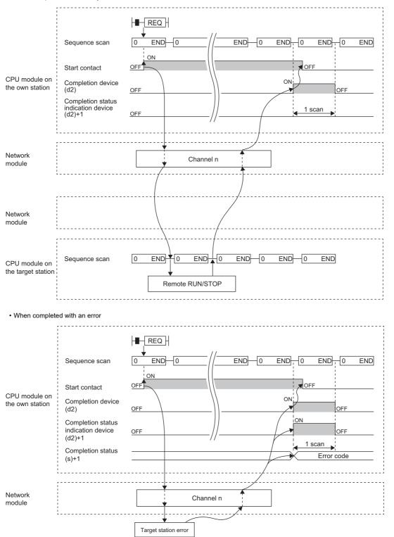
When the J.REQ/G.REQ instruction is used for execution, one complete cycle of write processing is followed by another while the write command is on. When the JP.REQ/GP.REQ instruction is executed, write processing is performed only once on the rising edge when the write command turns on.
