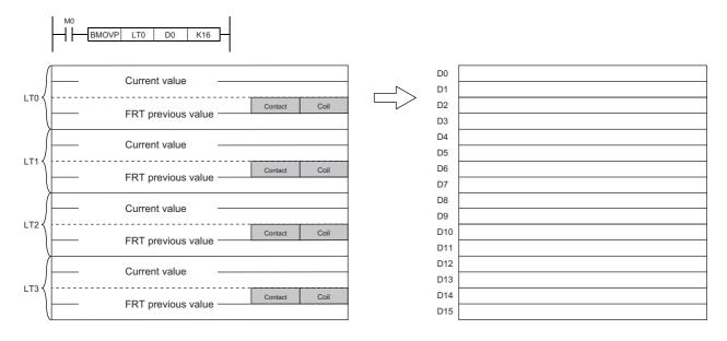
When the DMOV instruction is used, only current values are batch-transferred.
