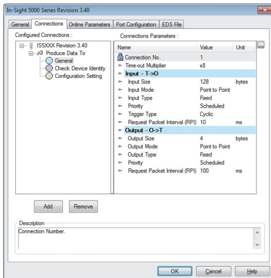
**3.** Configure the Class 1 tag communication settings for the connection 2 EtherNet/IP device.
