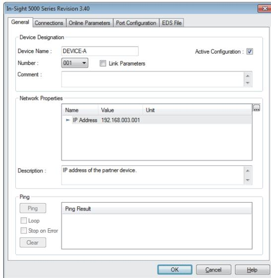
2. Configure the Class 1 instance communication settings for the connection 1 EtherNet/IP device.
