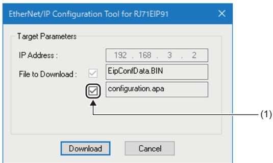
(1) Select the checkbox for "configuration.apa" under "File to Download" to download the setting file (\*.apa). The parameters can be changed as required by uploading the downloaded setting file (\*.apa).
