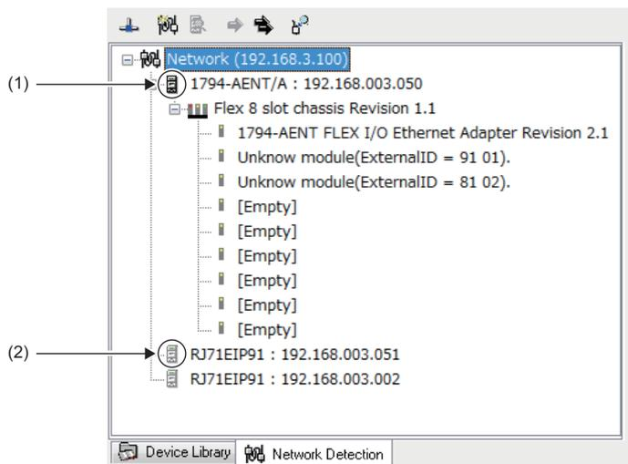
(1) Indicates that the EDS file for the detected RJ71EIP91 or EtherNet/IP device is added in "Device Library".
