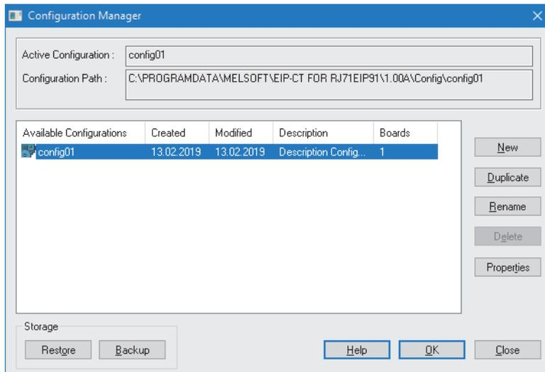
2. Click the [Restore] button to import the setting file to EtherNet/IP Configuration Tool.
