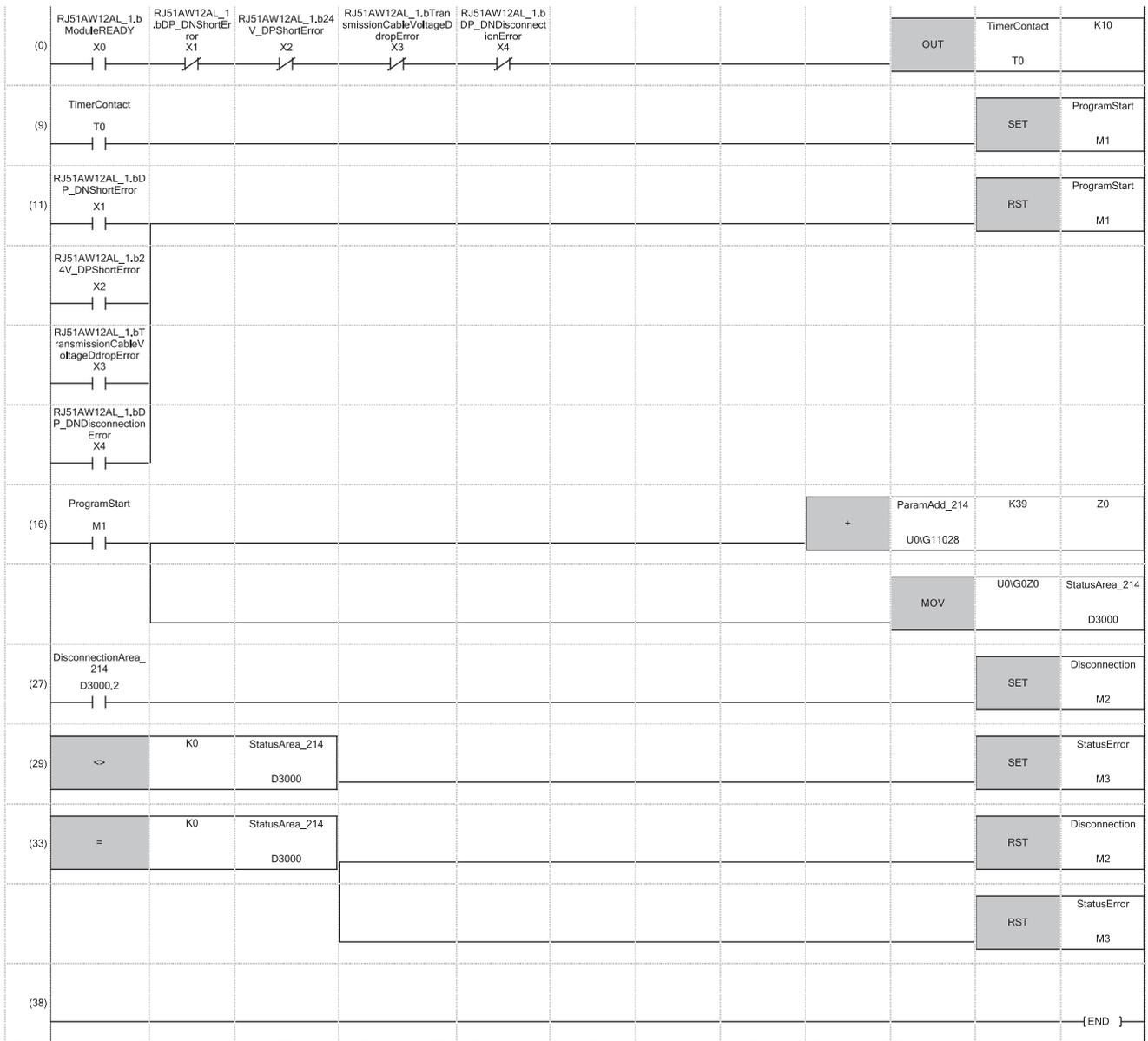
(16) Once 'ProgramStart' (M1) turns on, the buffer memory address determined by adding 39 to 'ParamAdd\_214' (U0G11028) of the remote module (ID: 214H) with the address 20 is stored in 'StatusArea\_214' (D3000).
