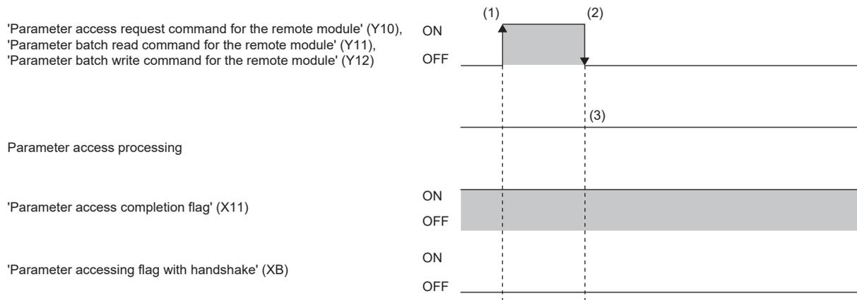
(1) Turn off and on any of the signals at any time to start the parameter access.
