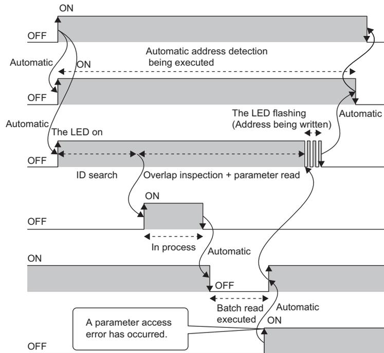
\*1 After turning on 'Automatic address detection command' (Y1), check that 'Automatic address detection flag' (X14) is on or check the SET LED status. Then, turn off 'Automatic address detection command' (Y1) with a program.
