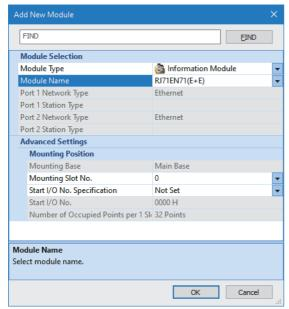
**5.** Click the [OK] button to add the module labels of the RJ71EN71.
