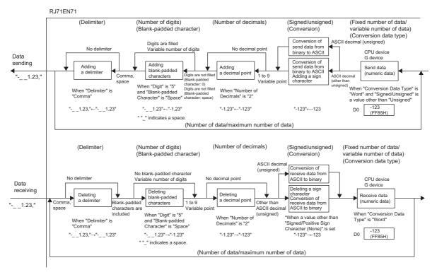
• Operation when "Conversion" is "HEX→ASCII Decimal" or "ASCII Decimal→HEX" and "Conversion Data Type" is "FLOAT [Single Precision]" or "FLOAT [Double Precision]"
