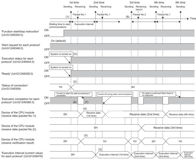
(1)When the latency time has elapsed and if 'Function start/stop instruction' (Un\G1249300.0) is turned on (enable) and 'Start request for each protocol' (Un\G1249348.0) is turned on (start), the data communication is started.
