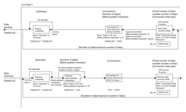
Operation when "Conversion" is "HEX—ASCII Decimal" or "ASCII Decimal—HEX" and "Conversion Data Type" is "Word" or "Double Word"
