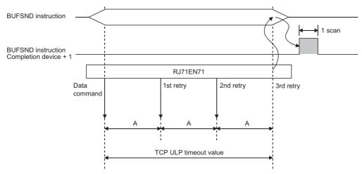
A: TCP resend timer value (The time at which data are sent when ACK is not returned after data transmission)
