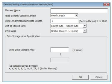
Use this to send the CPU module device or buffer memory data as part of the send packet, or to store part of the received packet in the CPU module device or buffer memory.
