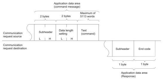
· When exchanging data with ASCII codes
