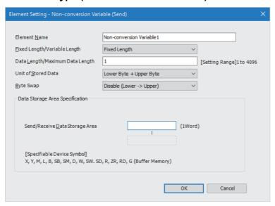
Use this type to send data of the CPU module device or buffer memory as part of the send packet, or to store part of the receive packet in the CPU module device or buffer memory.
