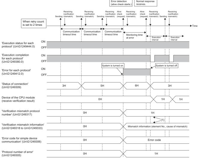
(1)The error will not be cleared even when the verification mismatch has been resolved. To clear the error, use 'Error clear request' (Un\G1249307).
