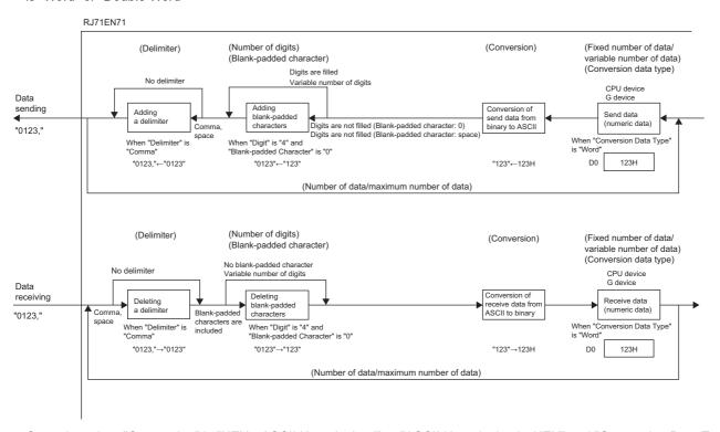
Operation when "Conversion" is "HEX—ASCII Hexadecimal" or "ASCII Hexadecimal—HEX" and "Conversion Data Type" is "FLOAT [Single Precision]" or "FLOAT [Double Precision]"
