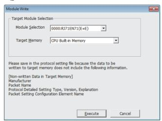
14. Write the set parameters to the CPU module. Then reset the CPU module or power off and on the system.
