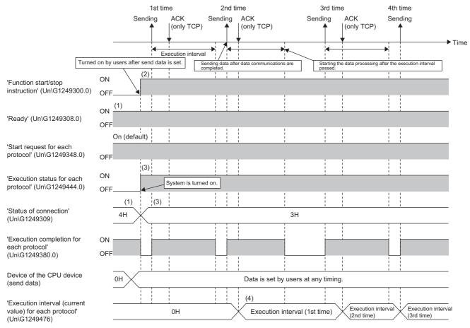
(1)When the system is powered off and on or the system is reset and the reset state is cleared and then the latency time has elapsed, 'Ready' (Un\G1249308.0) is turned on (ready) and 'Status of connection' (Un\G1249309) becomes 4H (function being stopped).
