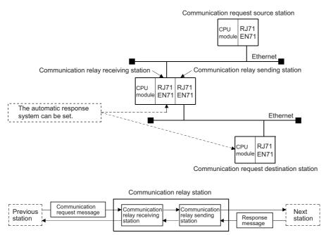
Conversion processing of the automatic response system is as below.
