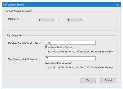
13. Write the set parameters to the CPU module. Then reset the CPU module or power off and on the system.
