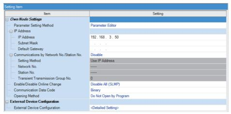
3. Write the set parameters to the CPU module. Then reset the CPU module or power off and on the system.
