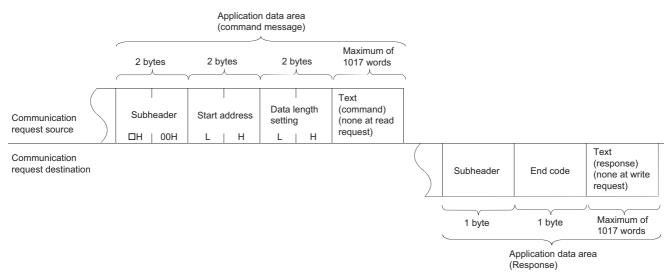
· When exchanging data with ASCII codes
