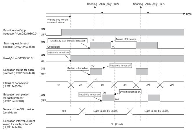
(1)Set data to be sent to the CPU module device and turn on (start) 'Start request for each protocol' (Un\G1249348.0).
