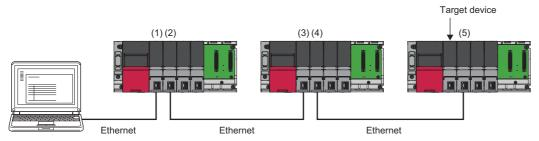
When a remote password is set for (1), the target device becomes accessible after the remote password is unlocked. When remote passwords are set for (2) to (5), the target device is accessible even when the remote passwords are not unlocked.
