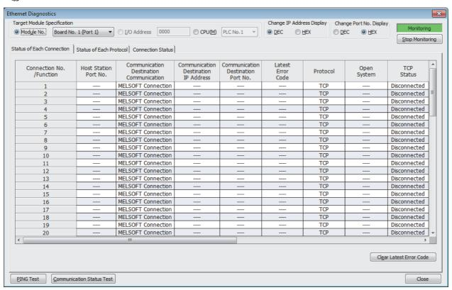
Set the Ethernet-equipped module to be diagnosed in "Target Module Specification".
