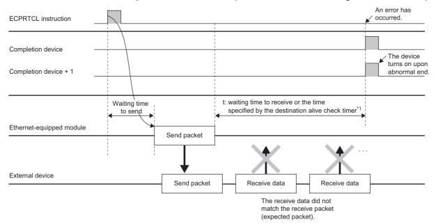
\*1 When the receive packet (expected packet) verification does not match before the reception wait time, or when other device existence cannot be checked within the destination alive check time (time calculated from destination alive check start interval timer value, destination alive check interval timer value, and destination alive check resend count).
