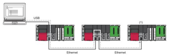
When communicating with CPU module shown as (1), ensure that all CPU modules have the firmware of the version supporting the communications by network number/station number. Also, set the network number and station number to all CPU modules.
