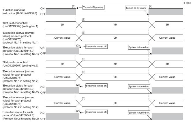
(1)Turn off (stop) 'Function start/stop instruction' (Un\G1249300.0) to stop communications with all the devices through the relevant Ethernet port. (2)When the stop request is accepted, 'Execution status for each protocol' (Un\G1249444.0) (protocol No.1 in setting No.1), 'Execution status for each protocol' (Un\G1250642.0) (protocol No.1 in setting No.2), and 'Execution status for each protocol' (Un\G1250642.1) (protocol No.2 in setting No.2) are turned off (execution stop).
