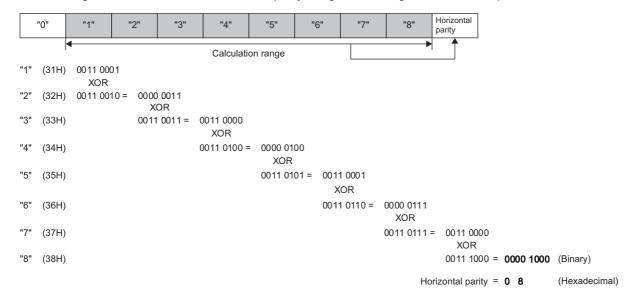
• Data flow: Forward direction, "No complement calculation" specified (08H in hexadecimal is 8 in decimal)
