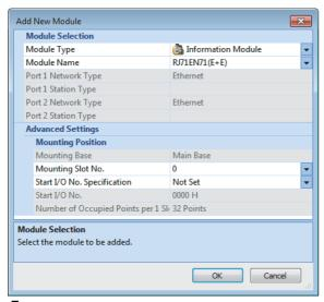
**5.** Click the [OK] button to add the module labels of the RJ71EN71.
