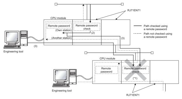
\*1 The remote password check is set, so the communication request from the external device is not accepted. If the remote password check is not set, the communication request can be accepted and data can be exchanged from the external device.
