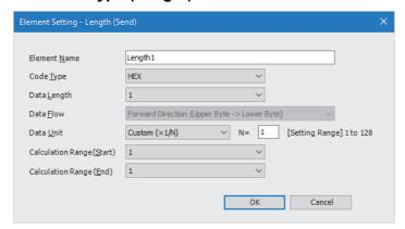
The length code is used when there is an element that indicates the data length in the packet.
