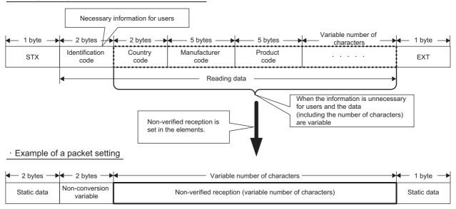
In the above type of packet format, the following operation can be executed by setting reception without verification.
