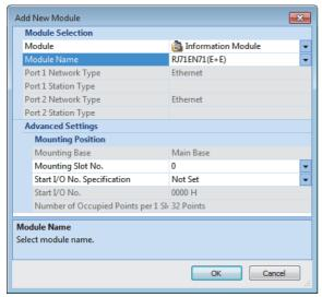
**5.** Click the [OK] button to add the module labels of the RJ71EN71.
