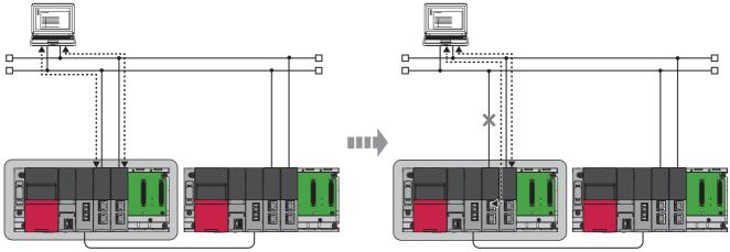
When both grouped RJ71EN71s have a communication error, a system switching request is issued.
