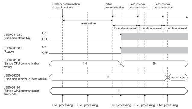
The standby system does not start simple CPU communication, even after the latency time elapses, and stands by until it becomes the control system due to system switching.
