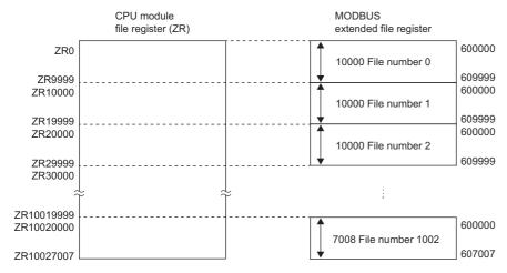
The size of the MODBUS extended file register depends on the size of the file register (ZR) set in the CPU module. For details, refer to the following.
