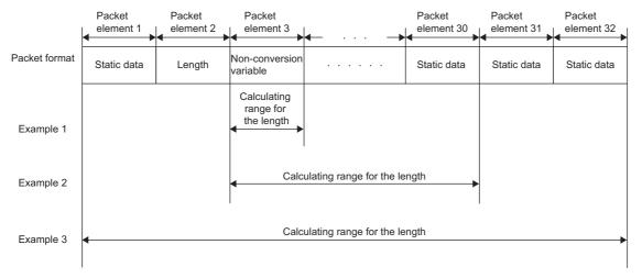
Example 1:Calculating range when start of range is set as 3 and end is set as 3
