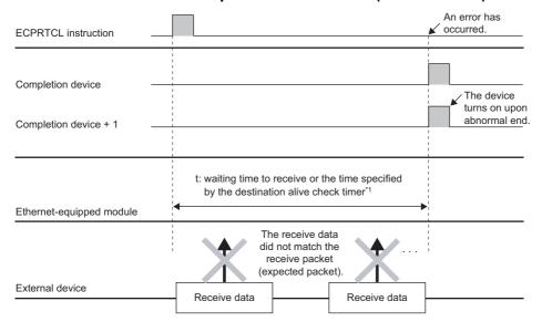
\*1 When the receive packet (expected packet) verification does not match before the reception wait time, or when other device existence cannot be checked within the destination alive check time (time calculated from destination alive check start interval timer value, destination alive check interval timer value, and destination alive check resend count).
