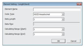
The length code is used when there is an element that indicates the data length in the packet.
