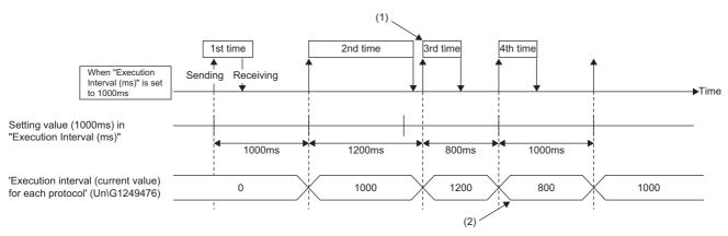
(1)If a response from the communication destination takes time more than "Execution Interval (ms)" that is set, the next sending is immediately executed. (2)If the response time from the communication destination exceeds "Execution Interval (ms)" in the previous communication, the value to be stored in 'Execution interval (current value) for each protocol' (Un\G1249476) in the next communication will be smaller than the value set for "Execution Interval (ms)".
