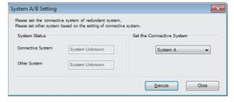
**11.** Write the set parameters to the system A CPU module.
