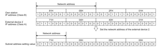
Ex. When the network address of the Ethernet-equipped module on the own station is the same as that of the external device
