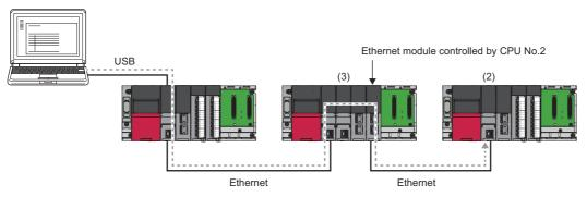
When communicating with CPU module shown as (2), ensure also that all CPU modules have the firmware of the version supporting the communications by network number/station number. Note, however, that the communication is possible even when the network number and station number are not set to CPU module shown as (3) of the CPU No.2.
