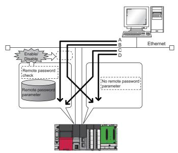
The remote password is checked when accessing with path A or B.
