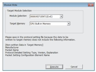
Select the module and memory into which the protocol data is to be written, and execute write.
