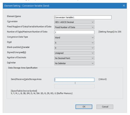
Use this type to send numerical value data of the CPU module device or buffer memory while converting it into an ASCII string or to store receive data (ASCII string) in the CPU module device or buffer memory while converting it into numerical value data.
