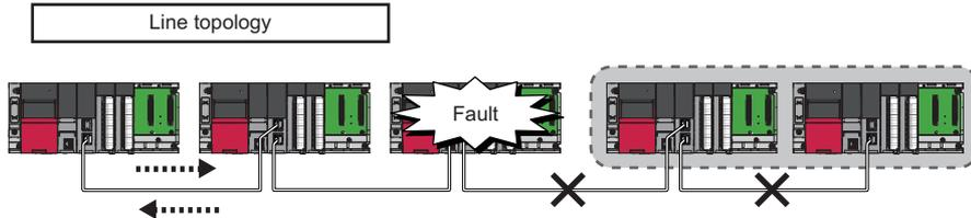
Stations connected after the faulty station are disconnected.
