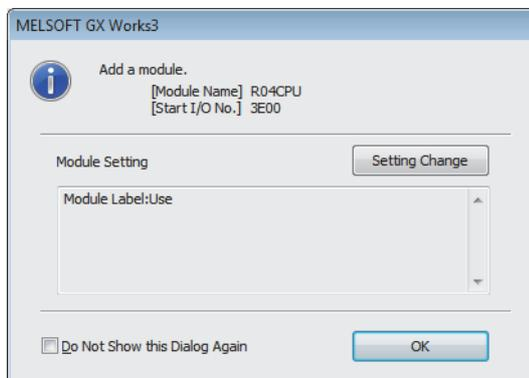
3. Click the [OK] button to add the module labels of the CPU module.
