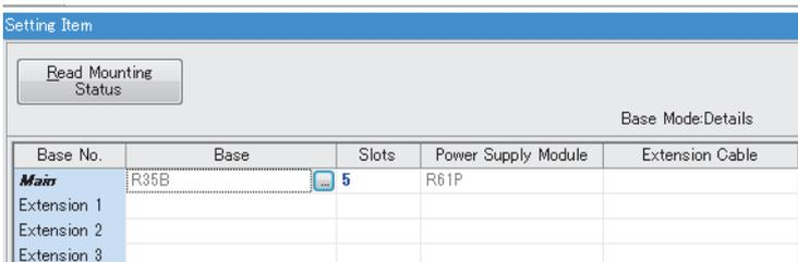
3. In the I/O assignment setting, set the I/O module with diagnostic functions to be mounted.
