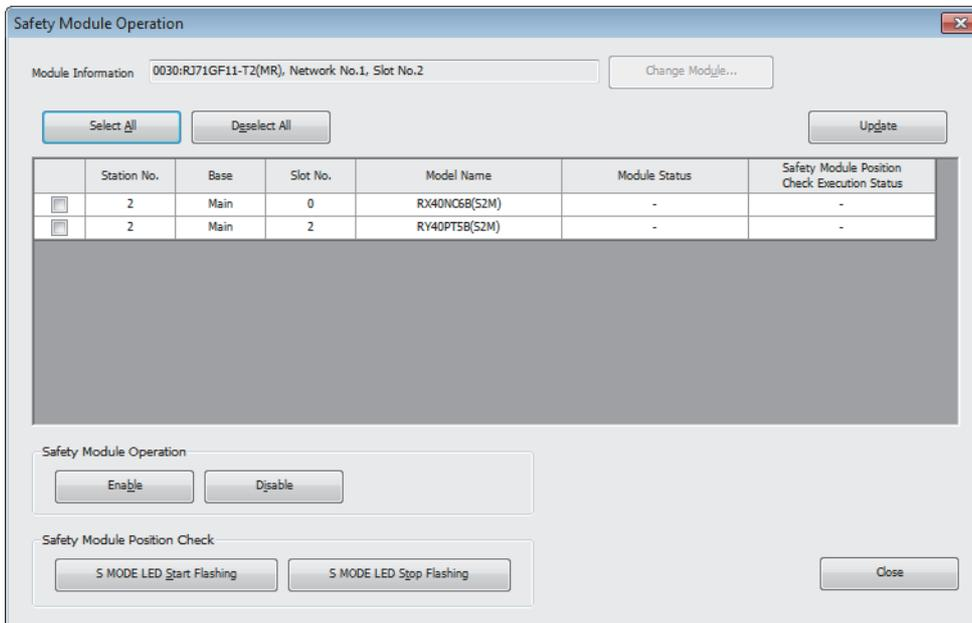
27. Select the checkbox of the RX40NC6B(S2M) and the RY40PT5B(S2M) to be validated, and click the [S MODE LED Start Flashing] button. Check the flashing of the LEDs on the RX40NC6B(S2M), RX40NC6B(S2S), RY40PT5B(S2M), and RY40PT5B(S2S). Following this step allows you to check whether the target module is set properly before starting validation.
