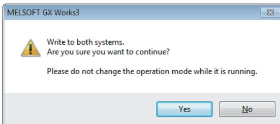
9. Either reset the CPU modules of both systems or power off and on both systems.
