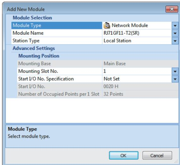
4. Click the [OK] button to add a module label of the RJ71GF11-T2.
