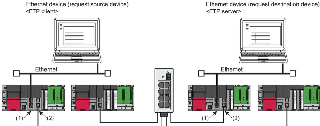
(1) RJ71EN71 ("Port 1 Network Type" and "Port 2 Network Type" is set to "Ethernet")
