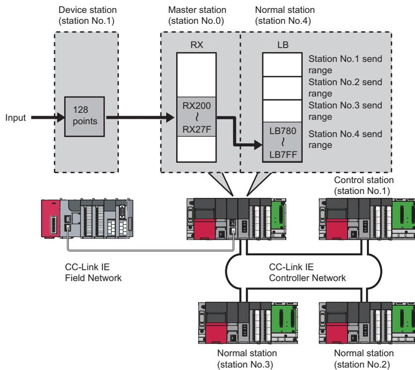
1. Select "0000: RJ71GF11-T2 (Master Station)" for "Transfer Source Module" and "0020: RJ71GP21-SX (Normal Station)" for "Transfer Destination Module", and enter the transfer ranges of link devices.
