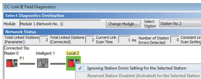
1. In "Network Status" of the "CC-Link IE Field Diagnostics" window, select the icon of the station for which temporary error invalid station setting is to be canceled.
