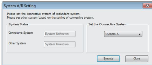
9. Write the set parameters to the system A CPU module.
