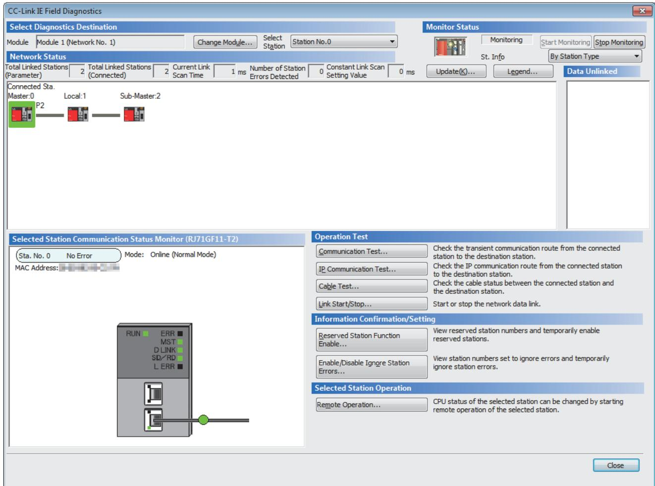
If an error icon appears in "Network Status" area on the "CC-Link IE Field Diagnostics" window, use the CC-Link IE Field Network diagnostics to identify the cause of the error and take corrective actions. (Page 269 Checking the Network Status)
