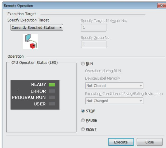
1. Select the module where the remote operations are performed in the CC-Link IE Field Network diagnostics.
