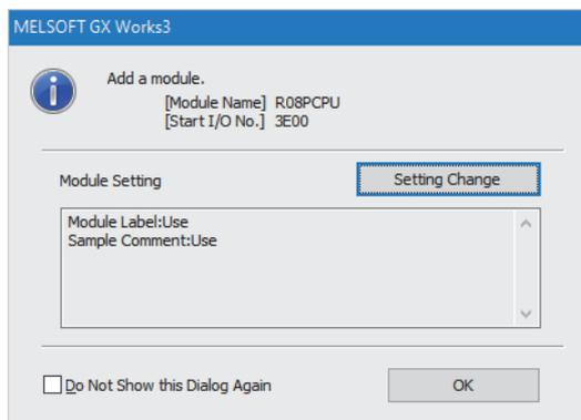
3. Click the [OK] button to add the module labels of the CPU module.
