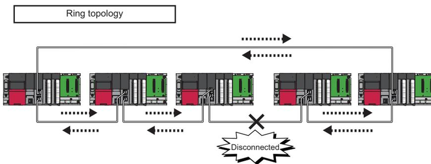
Even if a cable disconnection occurs, the system automatically performs loopback to continue the data link.
