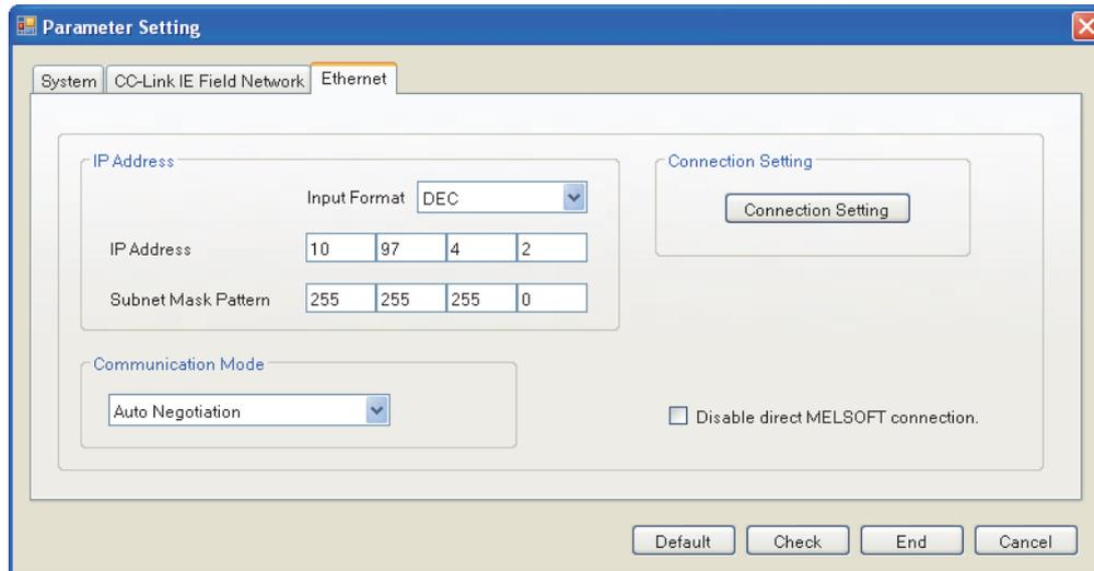
2. The IP address setting is not required for the Ethernet adapter module 2 (CC-Link IE Field Network part). The network address set in the master station 2 (station No.0) is automatically assigned.
