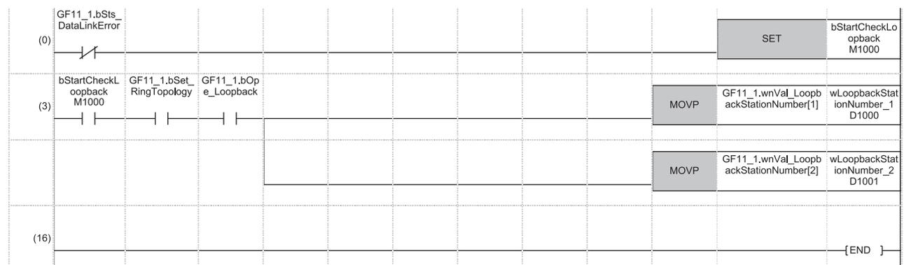
(3) When 'Network topology setting' (SB0078) and 'Loopback status' (SB0065) are on, 'Loopback station number 1' (SW0070) and 'Loopback station number 2' (SW0071) are saved.
