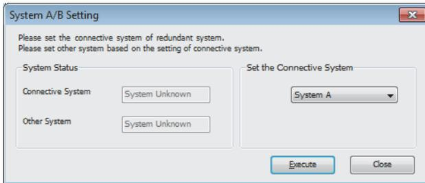
7. Write the set parameters to the system A CPU module.
