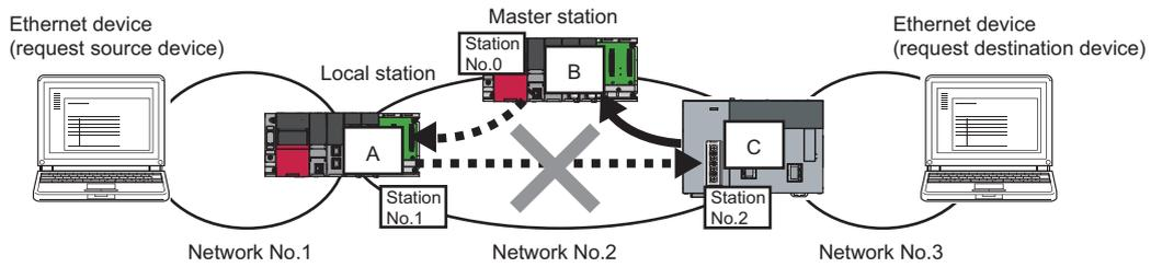
.....> Communication routes set using the routing parameters
