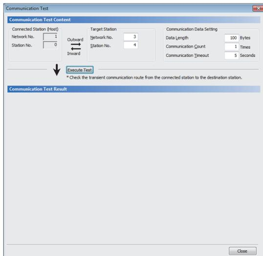
1. Open the "Communication Test" window and enter values for "Target Station" and "Communication Data Setting".
