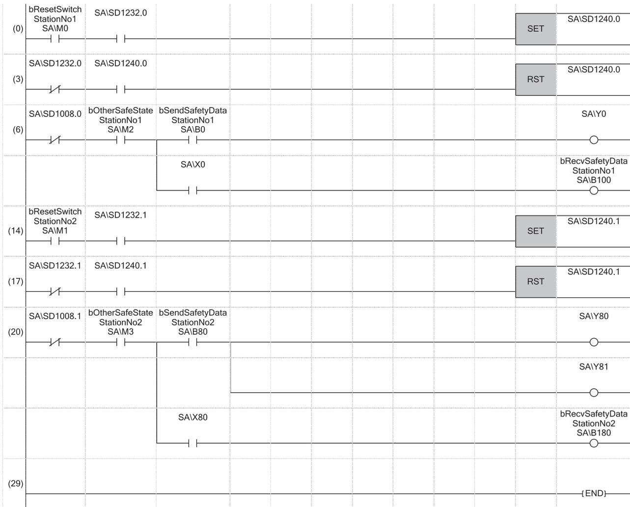
(0) Processing to release the safety station interlock status in safety communications with station No. 1
