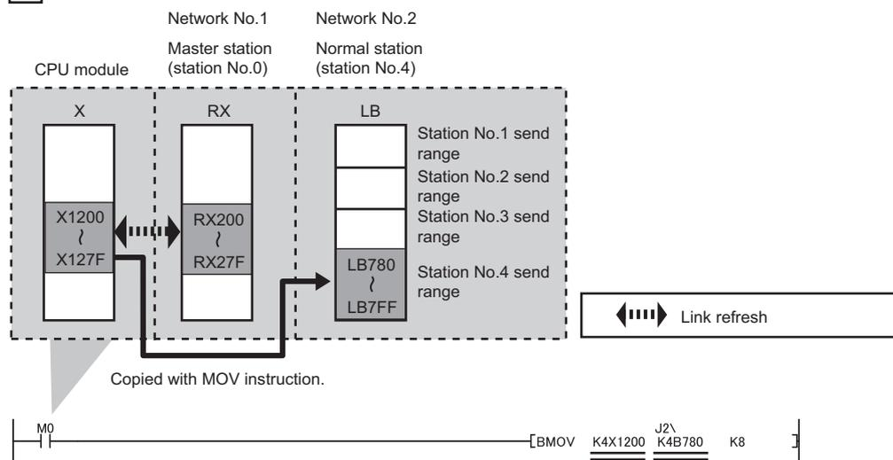
Link direct device cannot be specified for both the first and second arguments. Specify CPU device by link refresh for either one.
