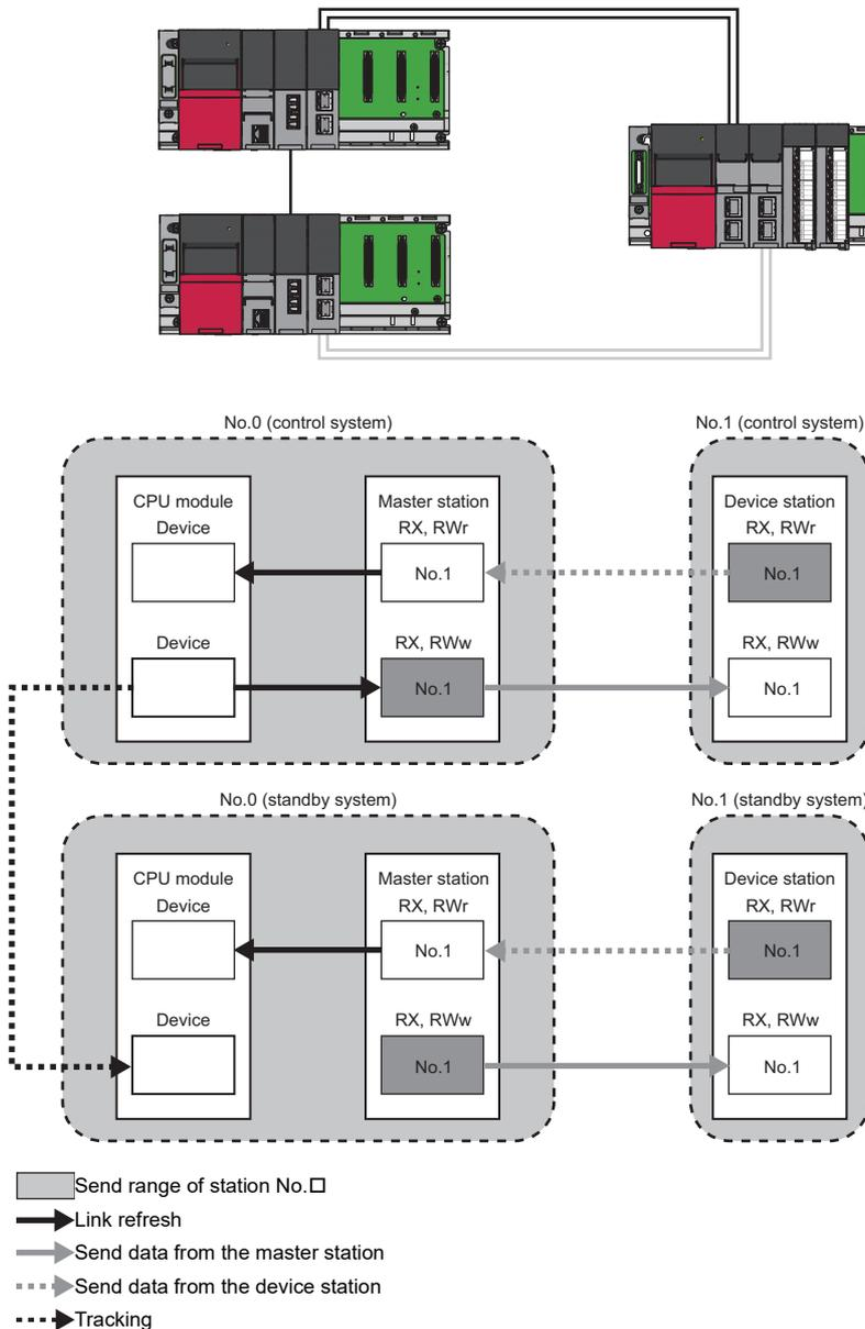
When system switching occurs due to an error in the control system, the control is switched to the network of the new control system.
