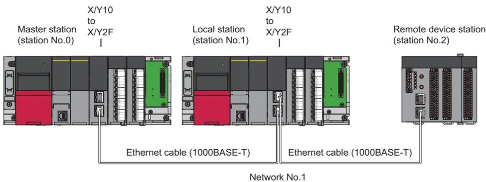
In this program example, I/O devices are connected to X0, X1 (double input) and Y0, Y1 (double output) of the remote device station.
