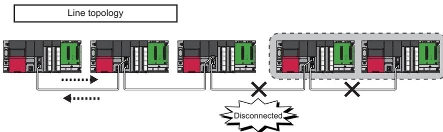
Stations connected after the cable disconnection point are disconnected.
