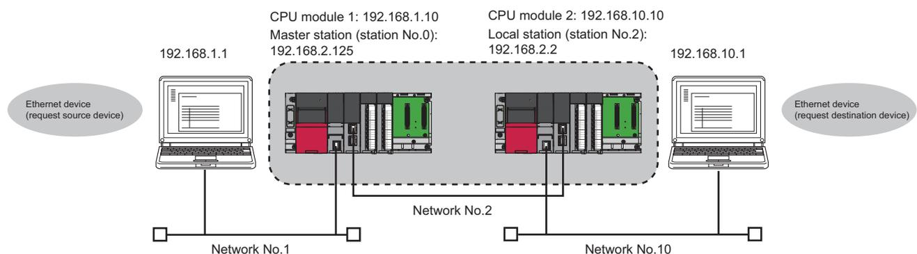
1. Open the "IP Communication Test" window. Enter the IP address of the CPU module 2 or the local station (station No.2) connected to the request destination device in "Communication Target". When the module that is connected to the request destination device is an Ethernet adapter module, enter the IP address of the request destination device in "Communication Target".
