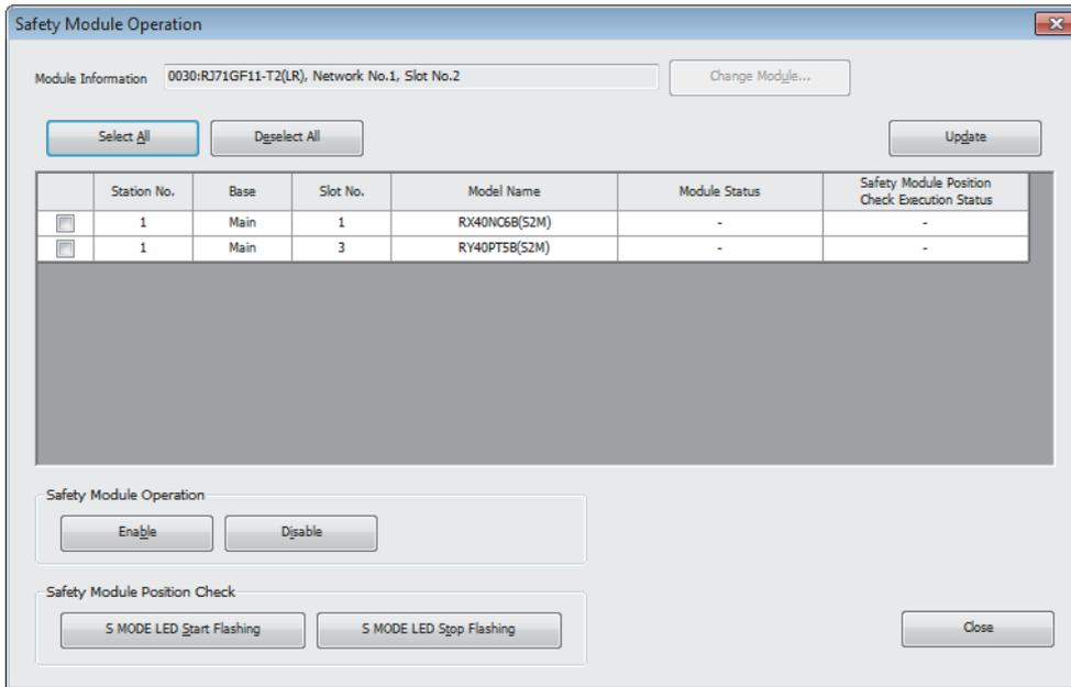
**27.** Select the checkbox of the RX40NC6B(S2M) and the RY40PT5B(S2M) to be validated, and click the [S MODE LED Start Flashing] button. Check the flashing of the LEDs on the RX40NC6B(S2M), RX40NC6B(S2S), RY40PT5B(S2M), and RY40PT5B(S2S) to be validated. Following this step allows you to check whether the target module is set properly before starting validation.
