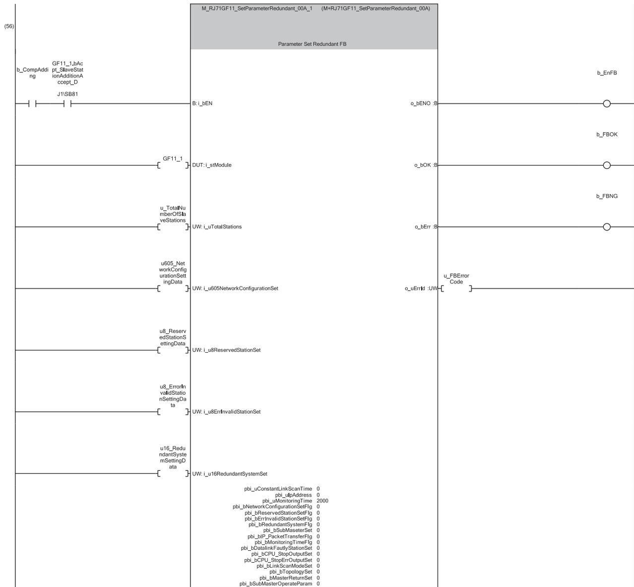
(56) Check that 'Device station addition acceptance status' (SB0081) is turned on and add the fourth station (local station (station No.3)) to the system configuration. By turning on b\_CompAdding, the parameters can be set.
