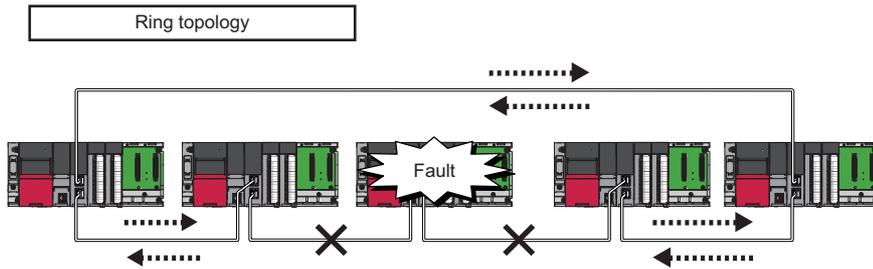
The system disconnects faulty stations and automatically performs loopback to continue the data link.
