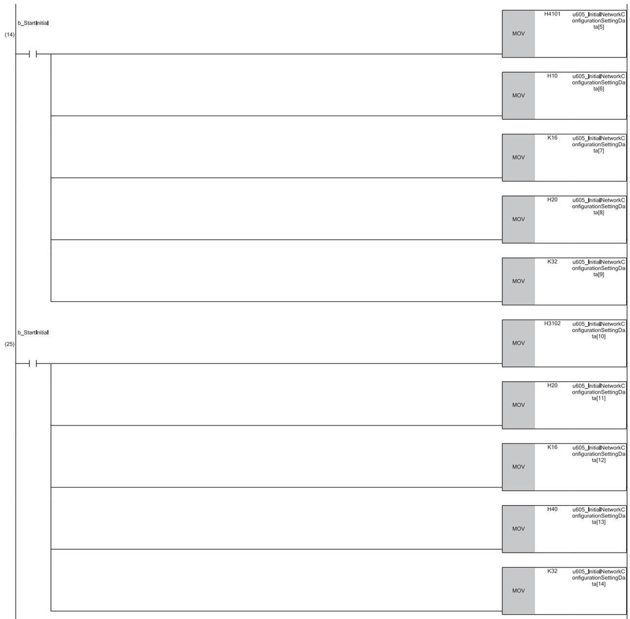
(14)Set the network configuration setting data for the second station (submaster station (station No.1)).
