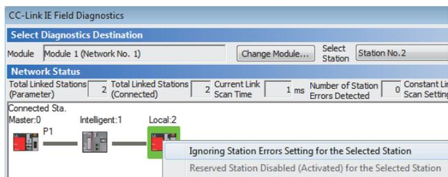
1. In "Network Status" of the "CC-Link IE Field Diagnostics" window, select the icon of the station to be temporarily set as an error invalid station.
