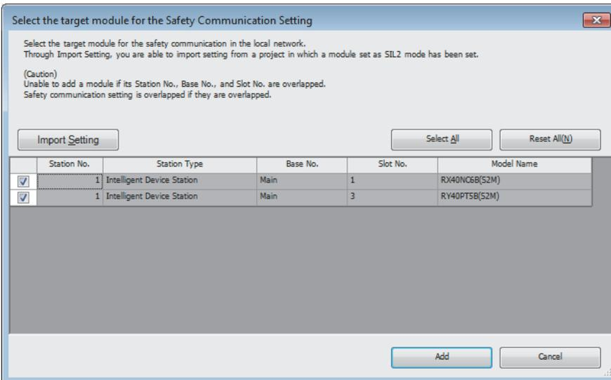
20. Set the safety communication setting of the added module in the "Safety Communication Setting" window.
