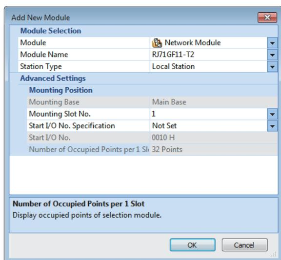
4. Add the module labels of the safety function module and master/local module. The addition method of the module label is the same as that of the master station. (☞ Page 190 Setting in the master station and remote device station)
