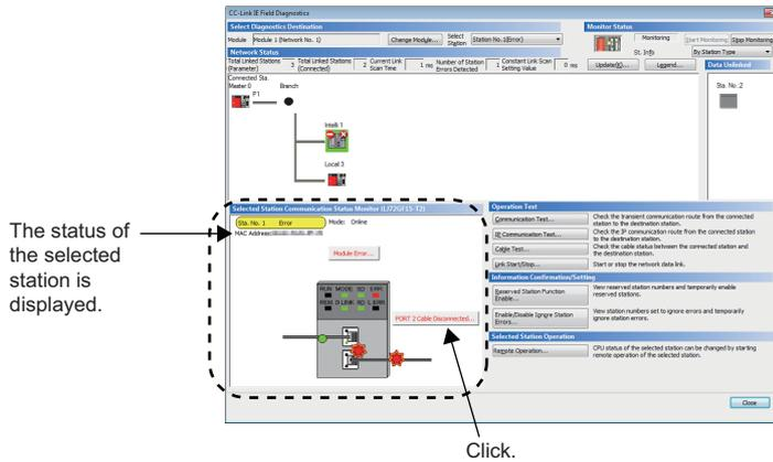
6. Various tests and operations can be performed by clicking the "Operation Test", "Information Confirmation/Setting", or "Selected Station Operation" on the bottom left of the window. (👉 Page 288 Link Start/Stop to Page 296 Remote Operation)
