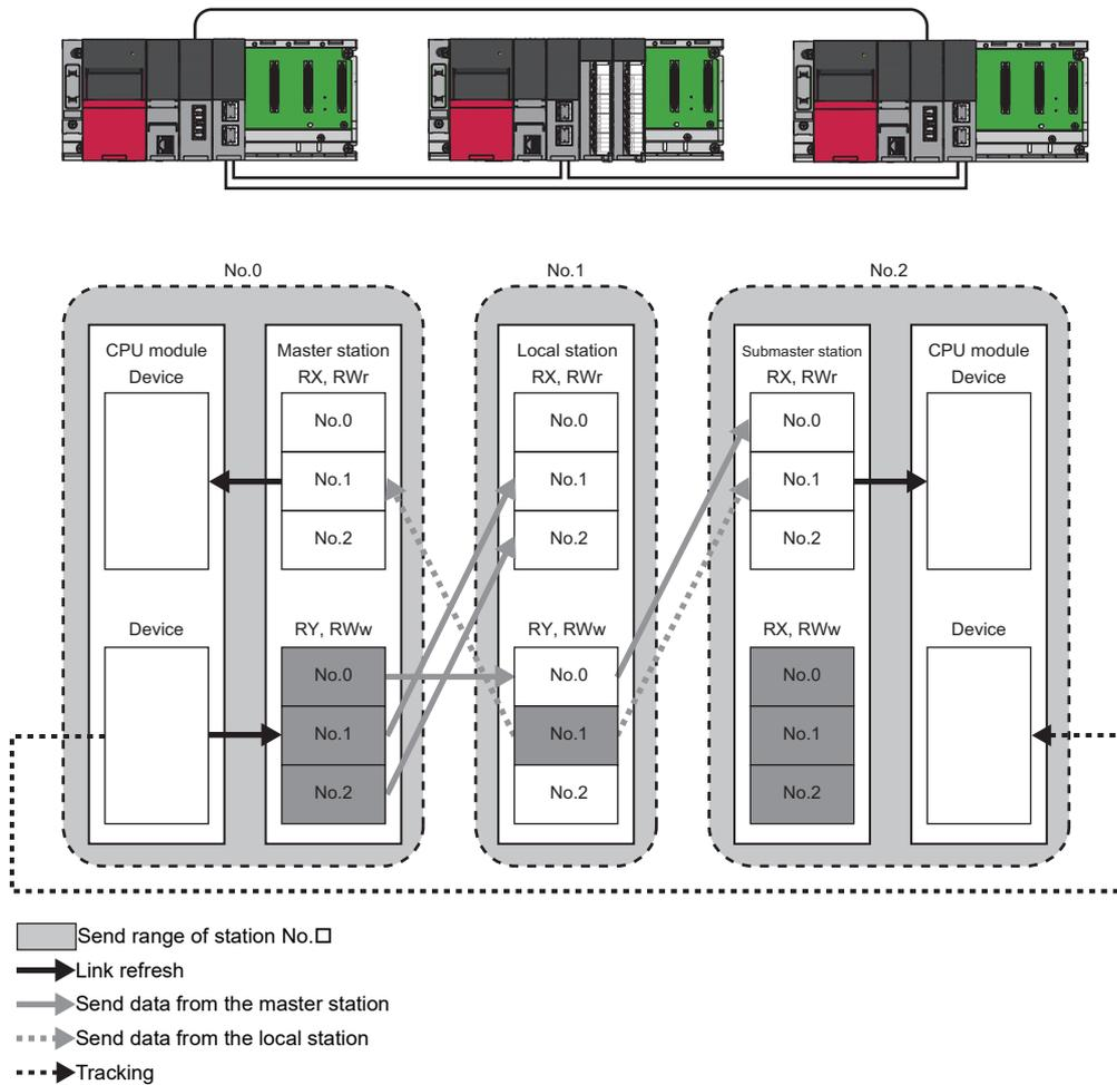
If system switching occurs due to an error in the master station (station No.0), the cyclic data is sent from the submaster station (station No.2), which starts operating as the new control system.
