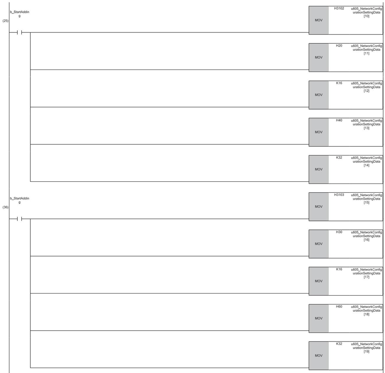
(25)Set the network configuration setting data for the third station (local station (station No.2)).
