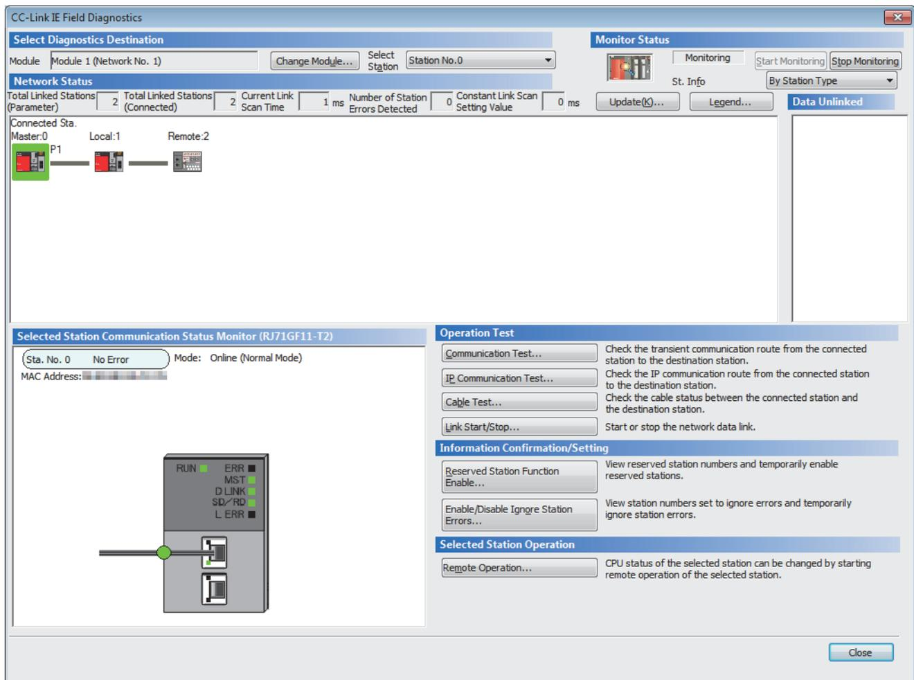
If an error icon appears in "Network Status" area on the "CC-Link IE Field Diagnostics" window, use the CC-Link IE Field Network diagnostics to identify the cause of the error and take corrective actions. (
