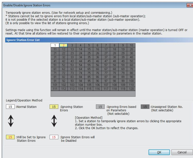
1. Open the "Enable/Disable Ignore Station Errors" window in the same way as described in the procedure for setting a temporary error invalid station.
