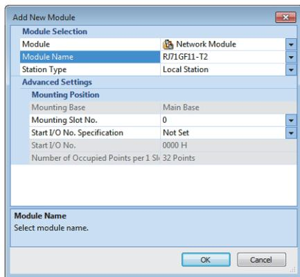
3. Add the module labels of the master/local module. The addition method of the module label is the same as that of the master station. (☞ Page 176 Setting in the master station)
