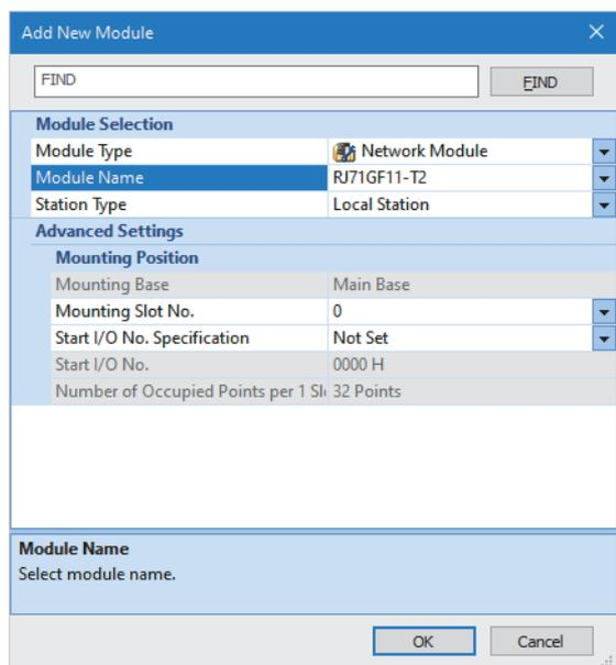
5. Click the [OK] button to add a module label of the RJ71GF11-T2.
