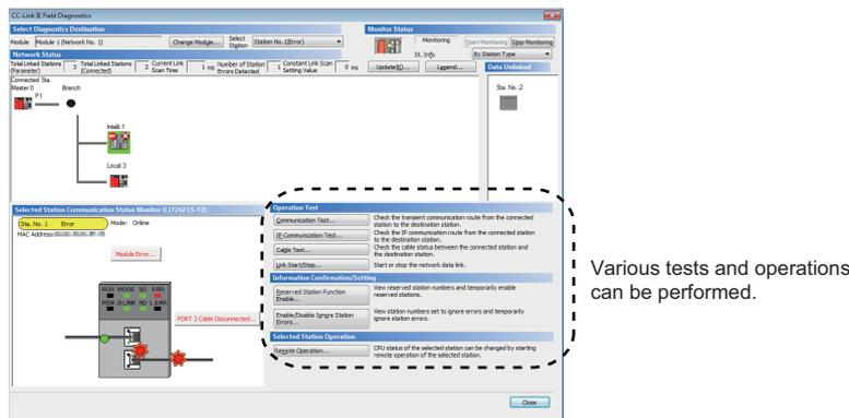
■ When a setting other than "No Specification" is specified in "Other Station Setting" on the "Specify Connection Destination Connection" window
