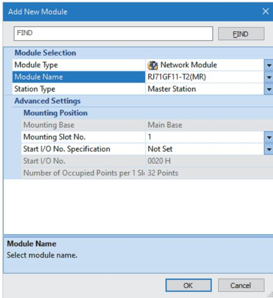
6. Click the [OK] button to add a module label of the RJ71GF11-T2.
