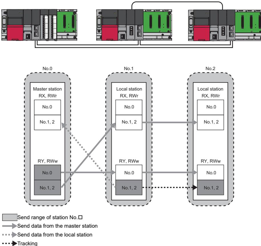
If system switching occurs due to an error in the local station (station No.1), the cyclic data is sent from the local station (station No.2), which starts operating as the new control system.
