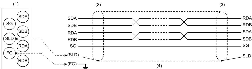
(1): Correspondence of the RS-422/485 terminal block and signal position
