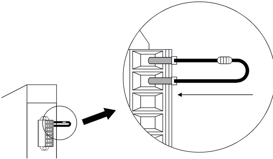
Incorrect insertion (Inserted horizontally)
