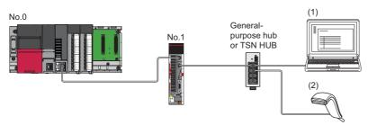
No.0: Master station No.1: Remote station (1), (2): Ethernet device
