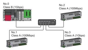
No.0: Master station No.1, No.2, No.3: Remote station Class A: CC-Link IE TSN Class A device Class B: CC-Link IE TSN Class B device
