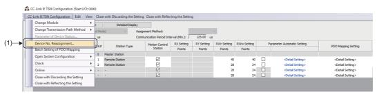
• Select the range of station Nos. to be reassigned device numbers (start station to end station) (2), and click the [Apply] button (3). The start/end of the linked device will be set automatically.
