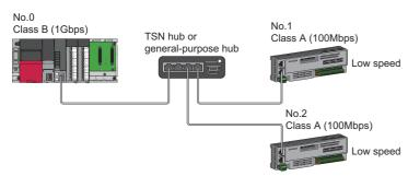
No.0: Master station No.1, No.2: Remote station Class A: CC-Link IE TSN Class A device Class B: CC-Link IE TSN Class B device
