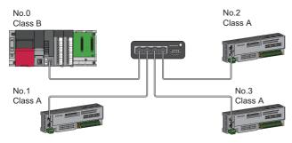
No.0: Master station No.1, No.2, No.3: Remote station Class A: CC-Link IE TSN Class A device Class B: CC-Link IE TSN Class B device When the "Communication Mode" is "Multicast", communication may not be possible depending on the communication
