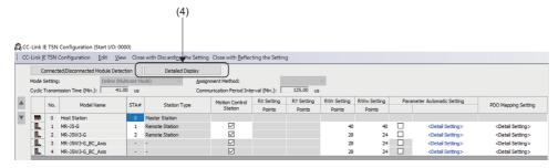
• Set the motion control station link device start in the first column of the RWr setting (5) and RWw setting (6) that are blank voluntarily.
