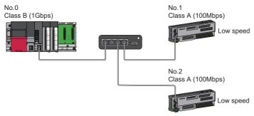
No.0: Master station No.1, No.2: Remote station Class A: CC-Link IE TSN Class A device Class B: CC-Link IE TSN Class B device
