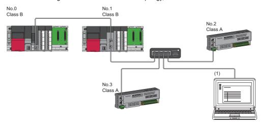
No.0: Master station No.1: Local station No.2, No.3: Remote station (1), (2): Ethernet device Class A: CC-Link IE TSN CI
