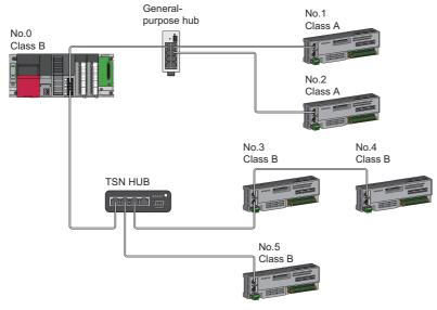
No.0: Master station No.1, No.2, No.3, No.4, No.5: Remote station Class A: CC-Link IE TSN Class A device Class B: CC-Link IE TSN Class B device
