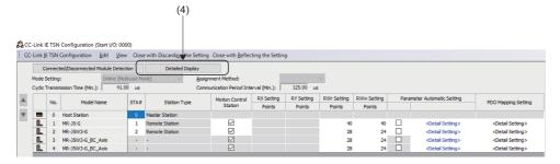
• Set the motion control station link device start in the first column of the RWr setting (5) and RWw setting (6) that are blank voluntarily.
