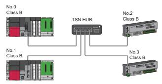
No.0: Master station No.1: Local station No.2, No.3: Remote station Class B: CC-Link IE TSN Class B device
