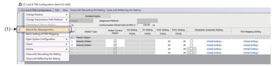
• Select the range of station numbers to be reassigned device numbers (start station to end station) (2), and click the [Apply] button (3). The start/end of the linked device will be set automatically.
