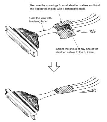
■Assembling of the connector (A6CON1)
