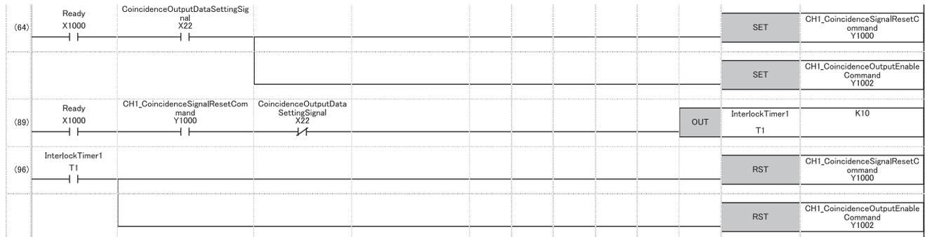
(64) Turns on 'CH1 Coincidence signal No.1 reset command' (Y1000) and 'CH1 Coincidence signal enable command' (Y1002).
