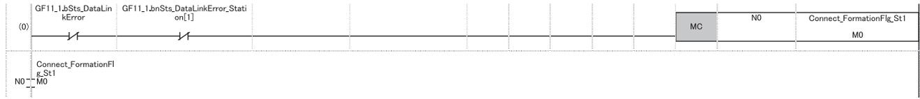
(0) Checks the data link status of the remote head module (station number 1).
