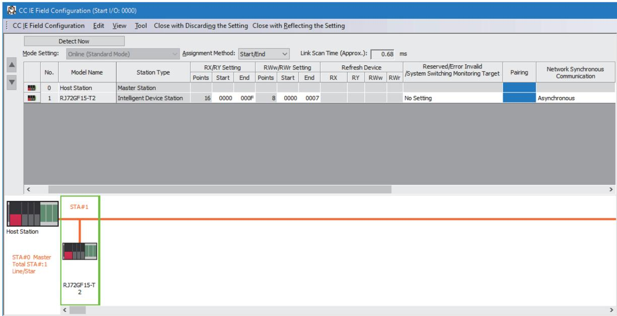
8. Set "Refresh Setting" of the module parameter of the master/local module as shown below.
