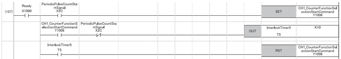
(157) Starts and stops the cycle pulse counter function
