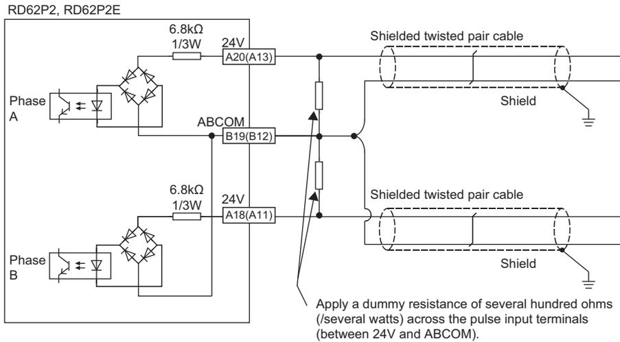
Shaping a pulse waveform is effective as a countermeasure against the following two cases.
