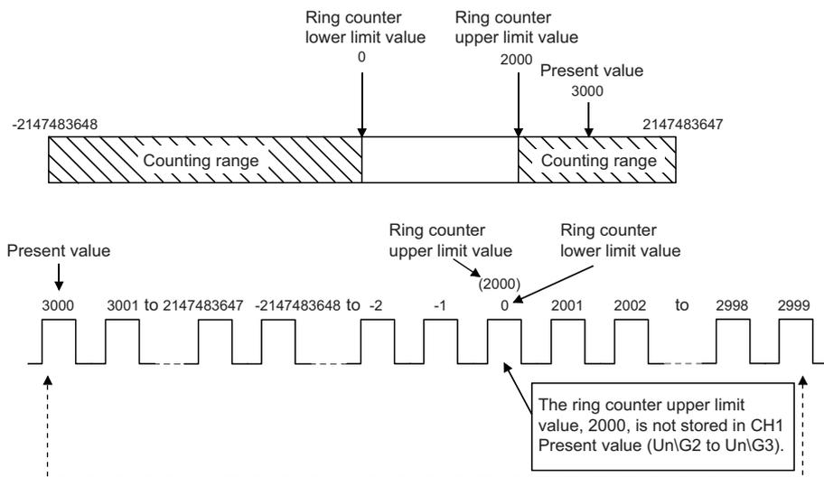
**■When the count range is Ring counter lower limit value = Ring counter upper limit value**
