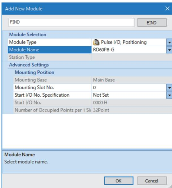
4. Set the window as follows to add the module label of the pulse input module.
