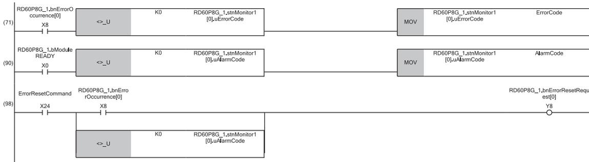
(71)'CH1 Error code' (Un\G9) is read. It is held even after the error is reset.
