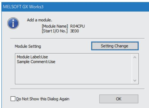
3. Add the pulse input module with the window set as follows.
