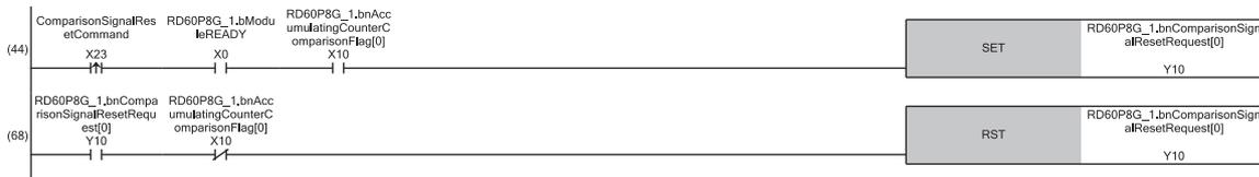
(44) 'CH1 Comparison signal reset request' (Y10) is turned on.
