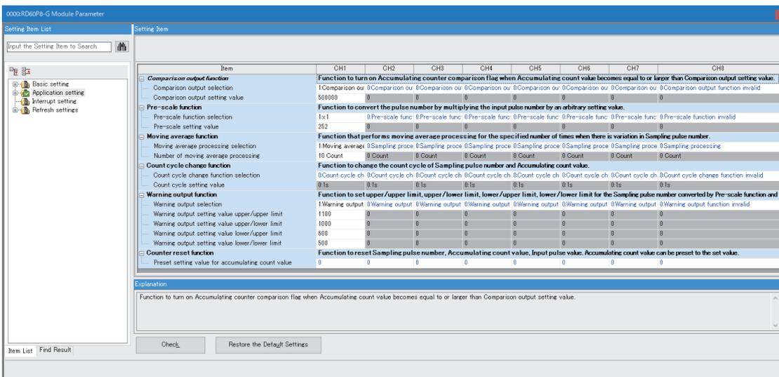
7. Write the set parameters to the CPU module on the master station. Then, reset the CPU module or power off and on the system.
