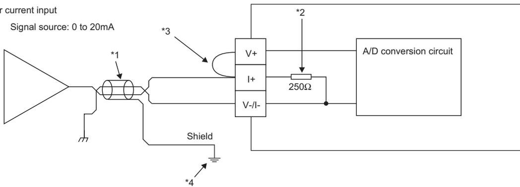
\*1 For the wire, use the 2-core twisted cable.
